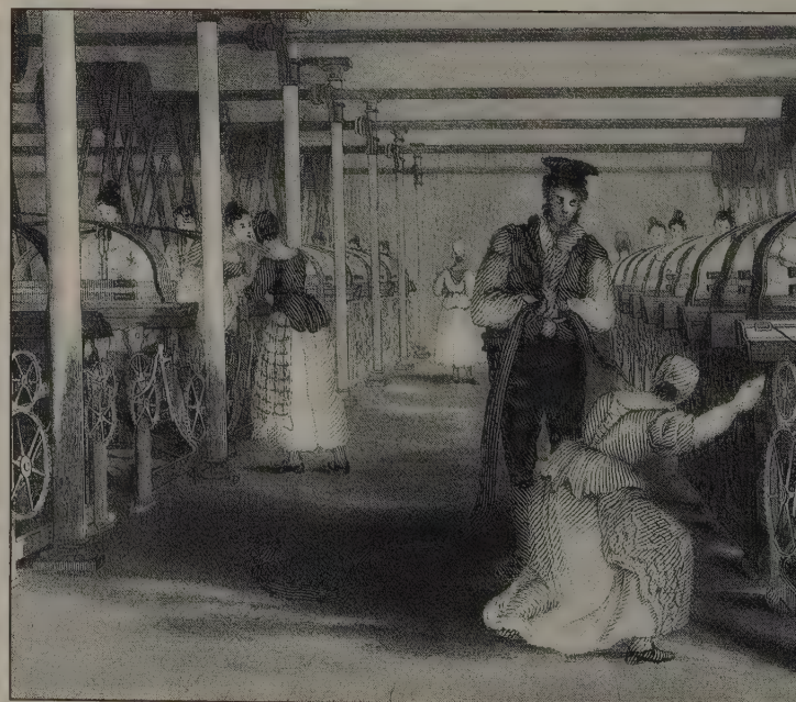
Looms in a cotton mill. They are driven by the belts connected to revolving shafts in the ceiling. The shafts were powered by a steam-engine.
