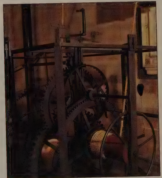
Part of the mechanism of the 600-year-old clock in Salisbury Cathedral, England. The clock is of the rope-and-drum type.
