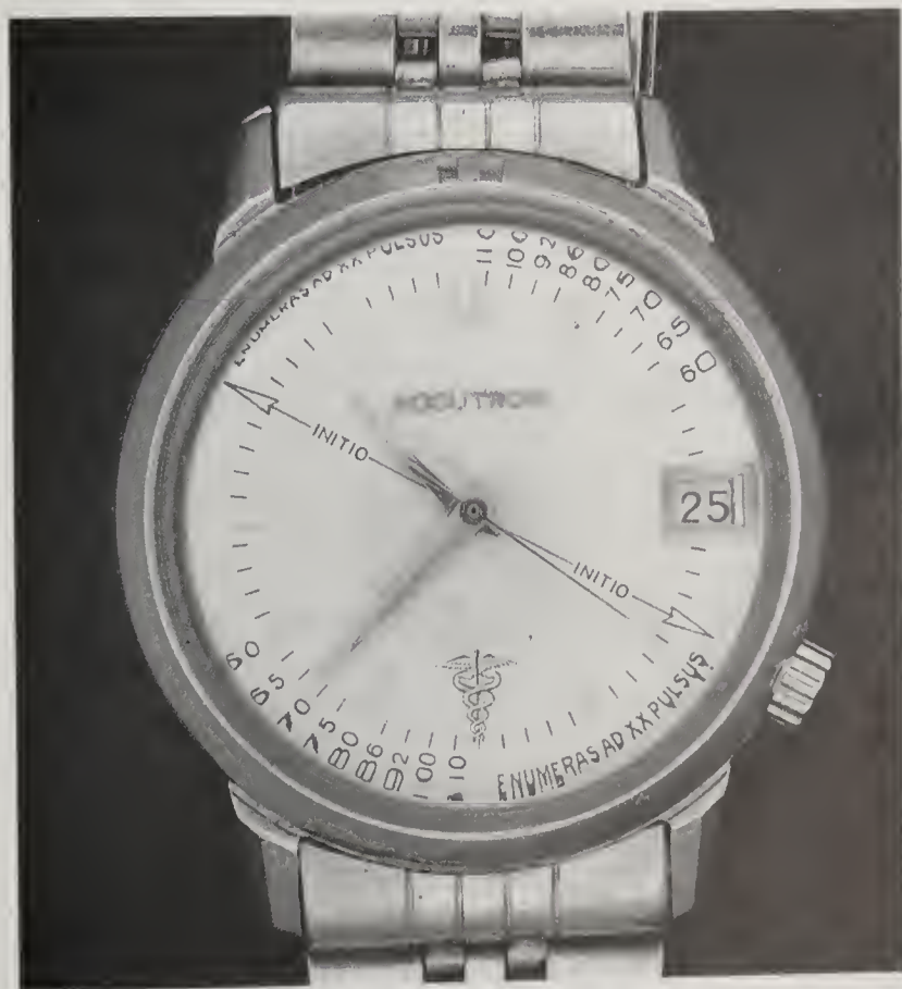
The Accutron electronic wristwatch had about half the moving parts of average watches. It supposedly never lost more than a minute a month.
