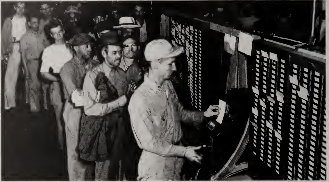
Factory workers inserted cards in automatic time clocks that stamped the hour they started and ended their workday.
