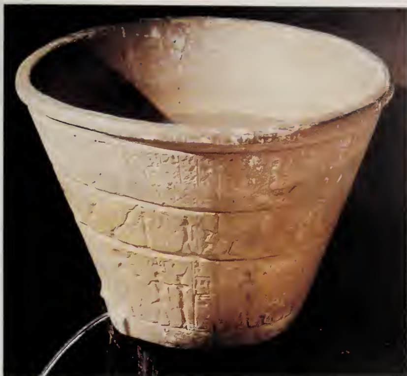
In a simple water clock, such as this one from Egypt around 1400 B.C., water flowed out of a hole. The dropping water level gave an indication of how much time had passed.
