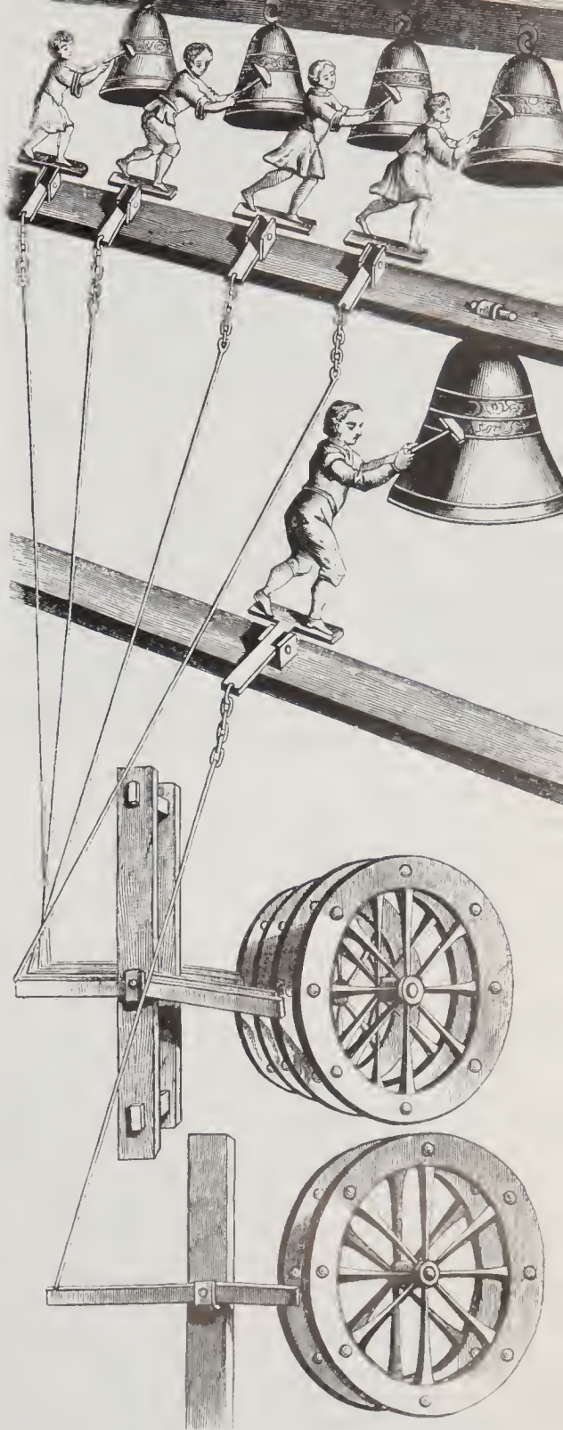
An illustration of a sixteenth-century French cathedral clock depicts jacks striking bells to sound the hour.
