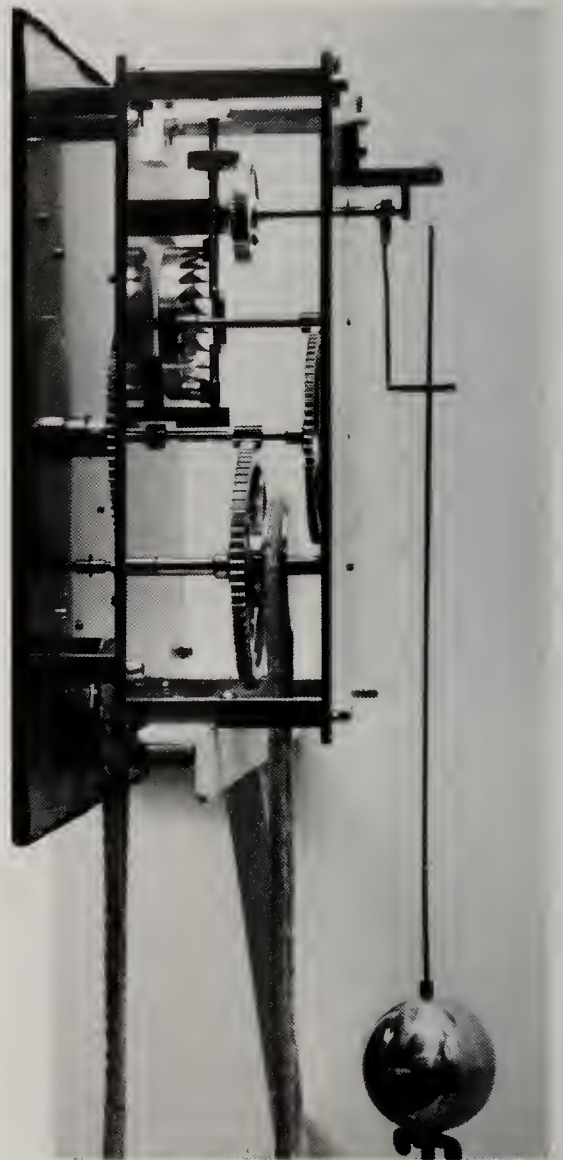
The pendulum made clocks more accurate than ever before. A reconstruction of Christian Huygens's seventeenth-century pendulum clock is shown here.
