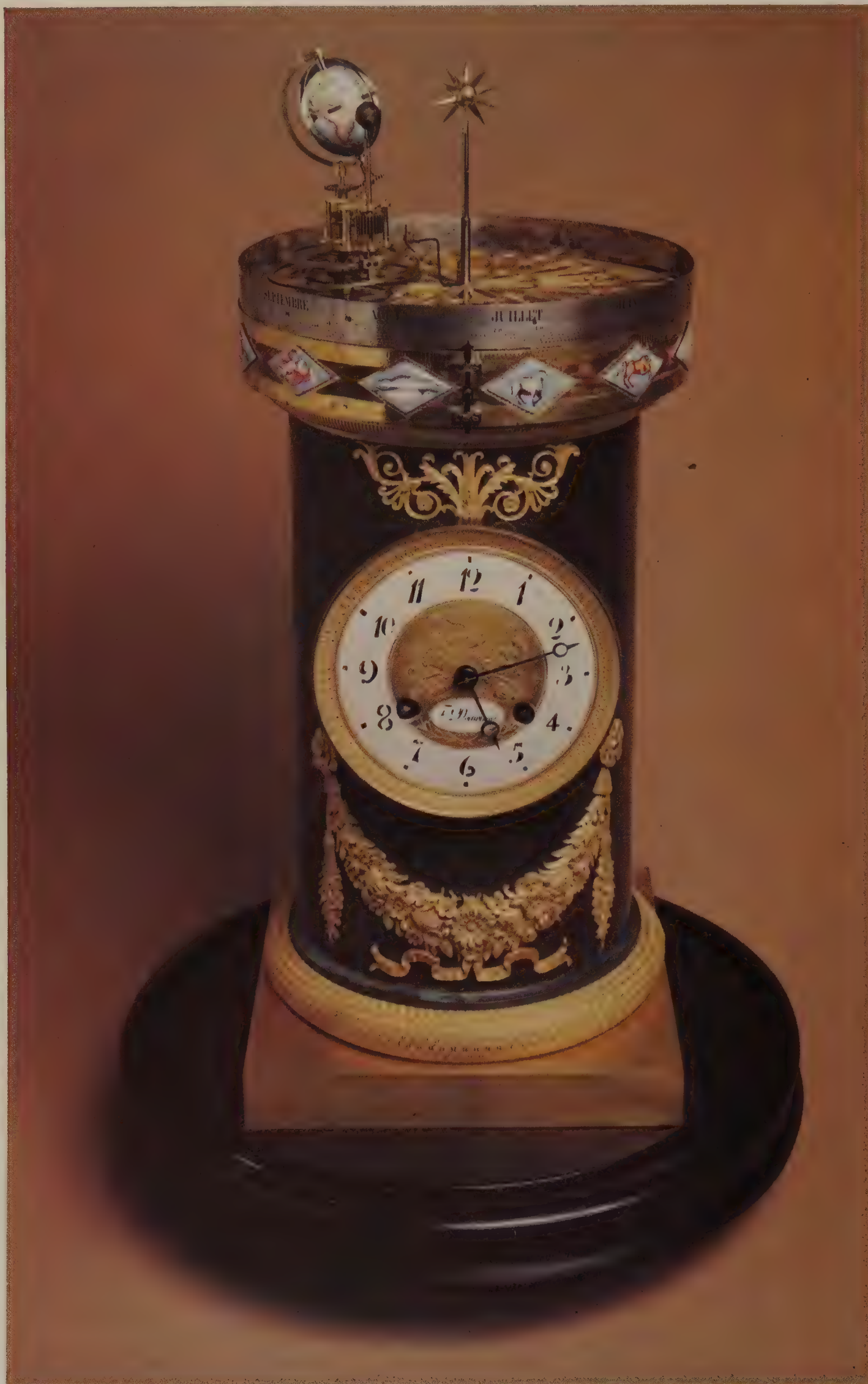
Left : A Swiss orrery clock by J. F. Ducommun of La Chaux de Fonds. The Earth revolves around the sun and the moon around the Earth.
