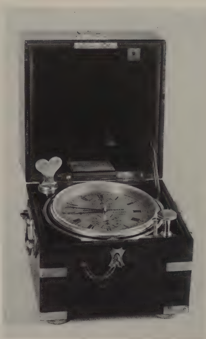
Left: A two-day box chronometer by Charles Frodsham, London. Two-day chronometers were normally for use at sea. The key, in a hole near the top hinge, was removed and the chronometer turned over in its gimbals for winding through a covered hole in the back. An up-and-down dial showed the number of hours in reserve.
