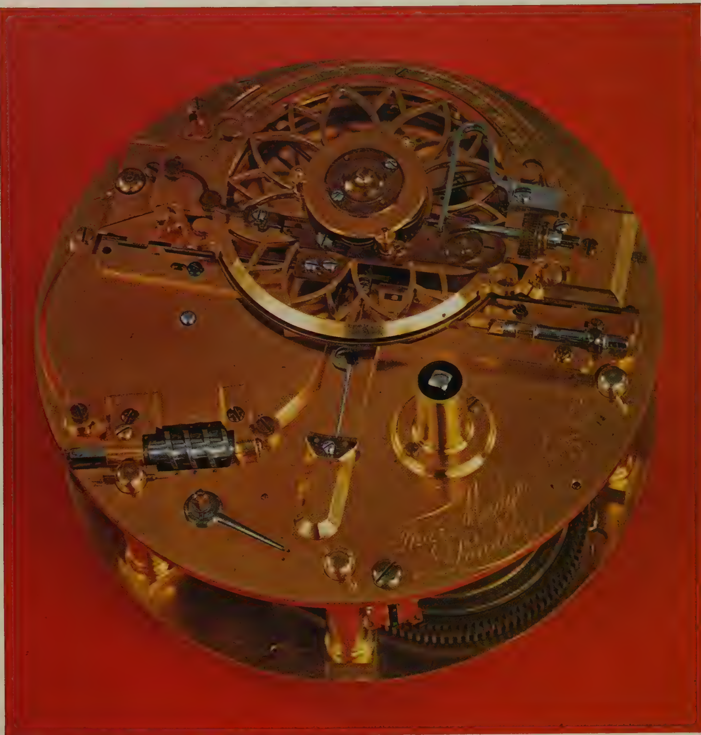
Left: After being appointed a member of the committee to examine Harrison's No. 4, Mudge became more and more interested in marine timepieces. This is the movement of his first (which he always referred to as his 'watch' because it did not strike). Later he made two copies, known as the 'Blue' and the 'Green'.
