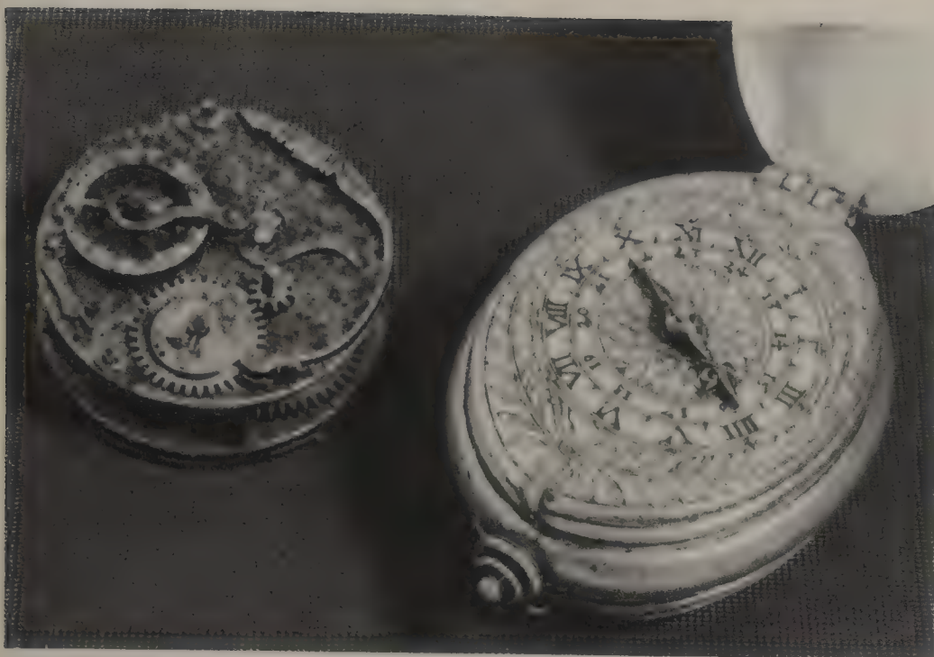
Above: A German sixteenth-century watch and the movement of another, both with stackfreed control. The stackfreed – the curved spring with a roller on the end that presses on the edge of a cam on the mainspring arbor – can be seen on the left. The toothless part of the toothed winding wheel is the stopwork.
