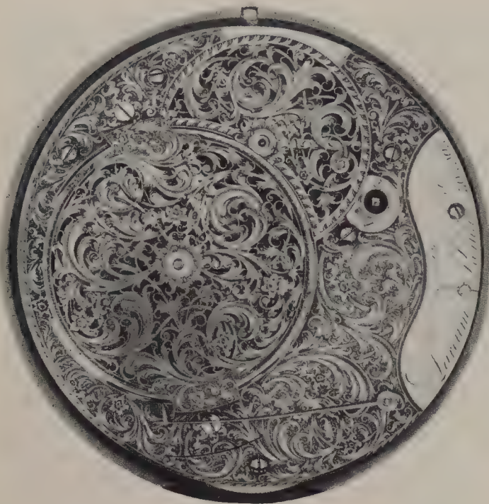
Left : The back plate of Larcum Kendall's first duplicate, K.1, of H.4. Captain Cook used it for navigation in his second voyage to the Pacific in 1772.
