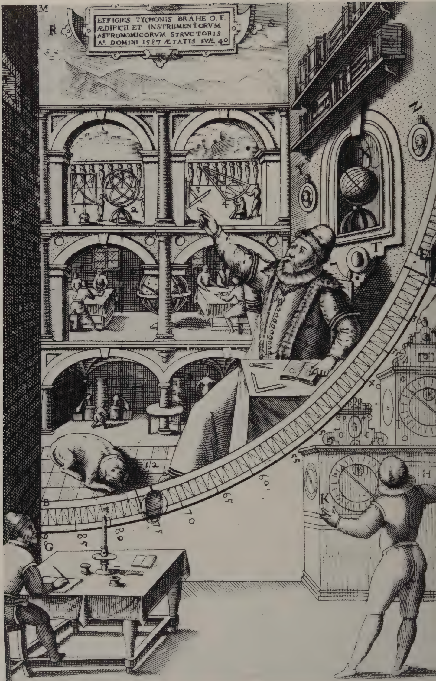
Right : Tycho Brahe's mural quadrant and two clocks, shown in the 1602 edition of his Astronomiae Instauratae Mechanica (1598).
