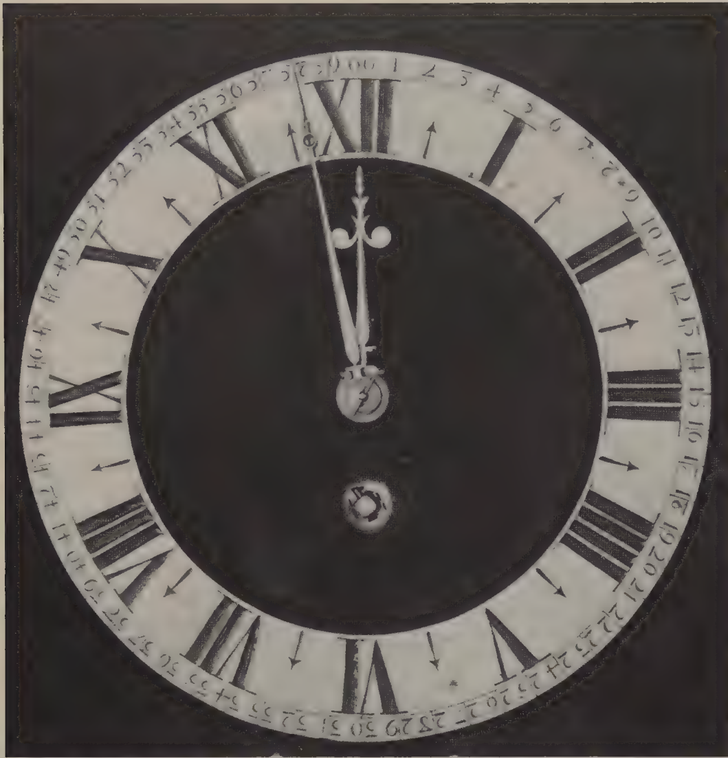
Above: The dial of the original pendulum clock of 1657, which has a velvet ground. It is a small spring-driven wall clock.
