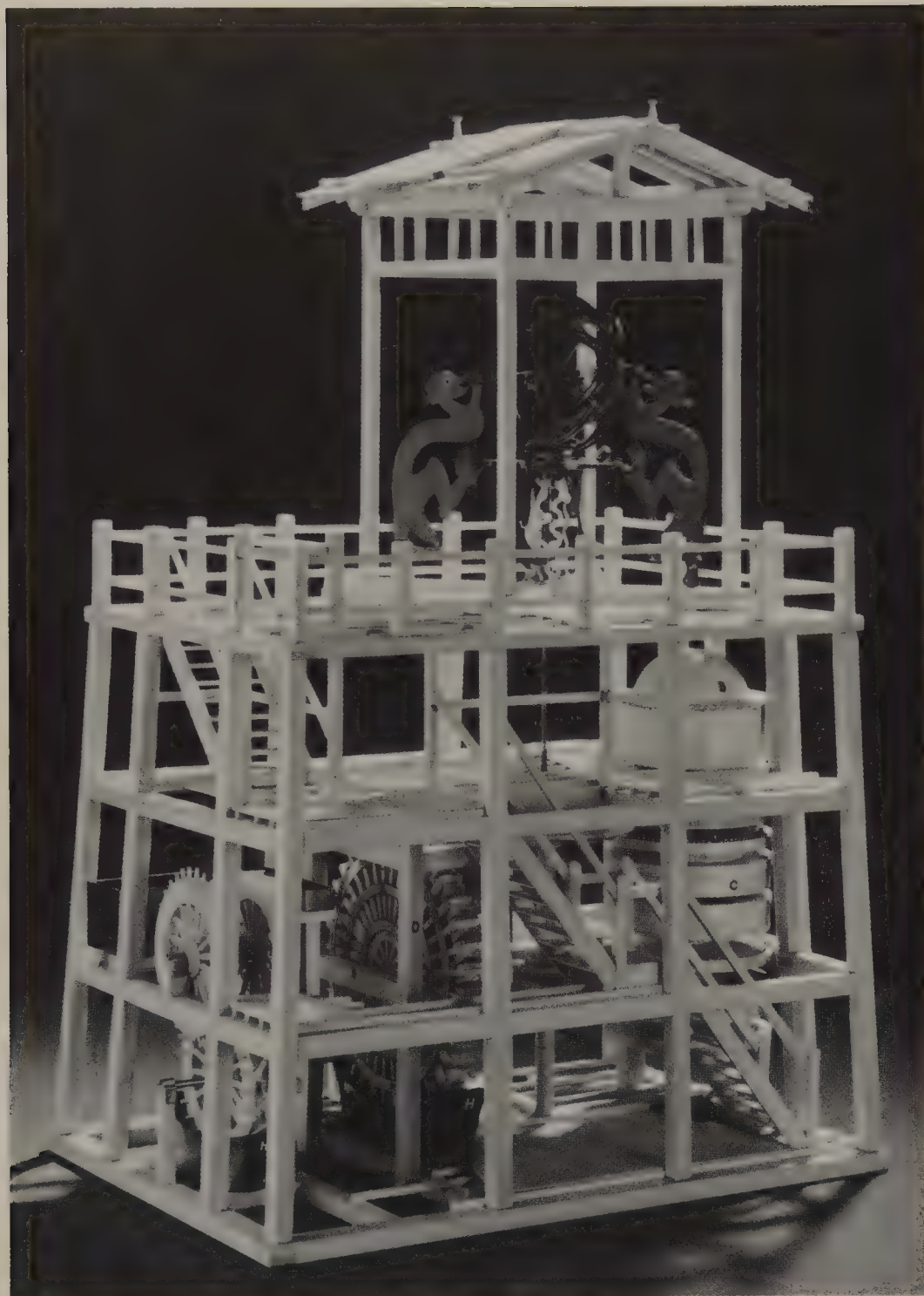
Above: A model of Su Sung's astronomical hydraulic clock tower of 1088 by Mr J. H. Combridge, in the Science Museum, London. The original tower was 11.3m (37 ft) high.
