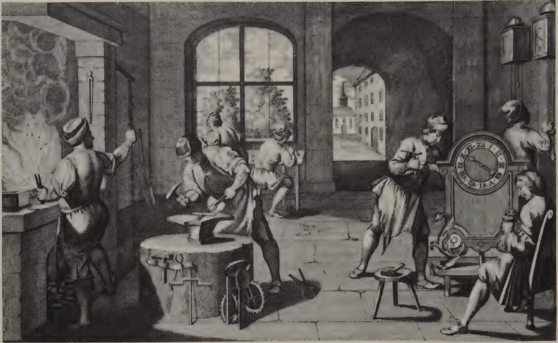
Above : A clockmaker's workshop c. 1740, in a print by Martin Engelbrecht, Augsburg. The frame of a watchman's clock and a foliot are propped up against the anvil base in a way reminiscent of the Stradanus print on page 62. Again, the bench work, such an essential part, is very much in the background.
