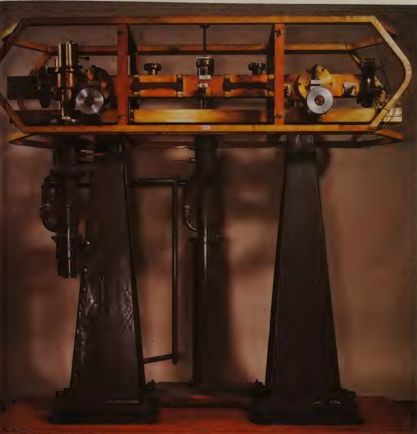
Left : The original atomic clock at the National Physical Laboratory. It kept time to the equivalent of one second in three hundred years. The latest version is more than ten times more accurate.
