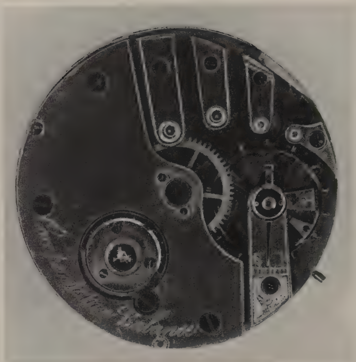
Right : Jean Antoine Lépine introduced his Lépine calibre about 1760 in which separate bars were used instead of a top plate. The idea was developed in such movements as this, to make them thinner and easier to service.
