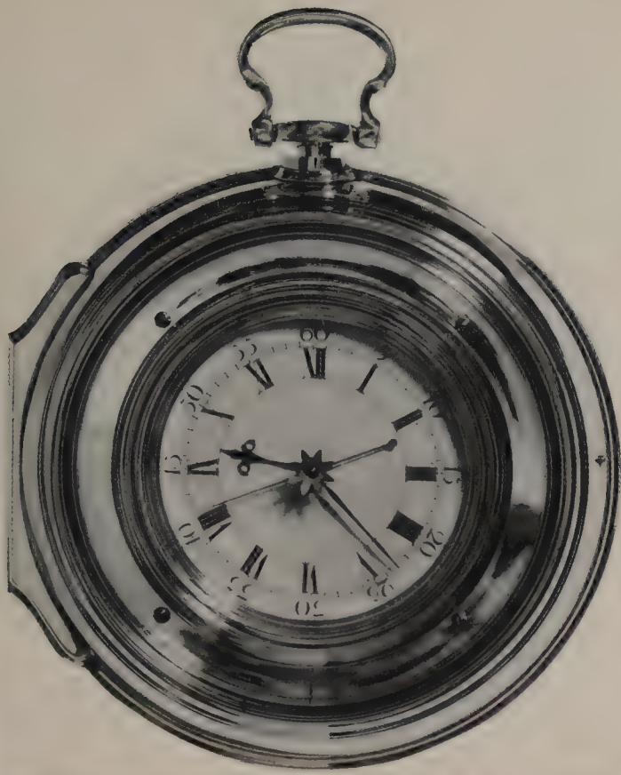
Left : Harrison's last marine timepiece, H.5, which he made under protest. It is like H.4 but plainer. The gold star in the middle is for setting the hands. George II tested it in 1772.
