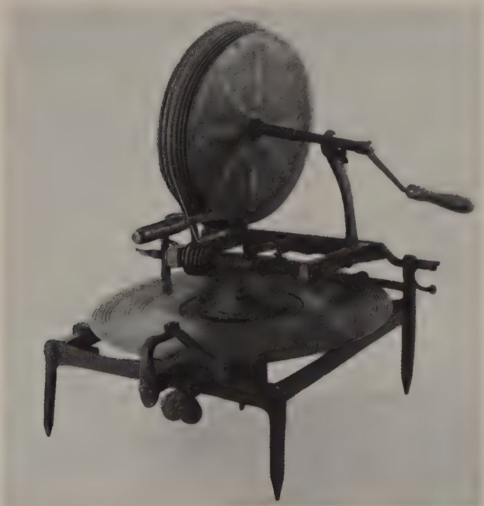
Left : A wheel cutting engine inscribed ‘Knight’s Horologium machina 1783’. The indexing wheel at the bottom determines the number of teeth. The pulley drive provides high speeds for the cutting wheel.
