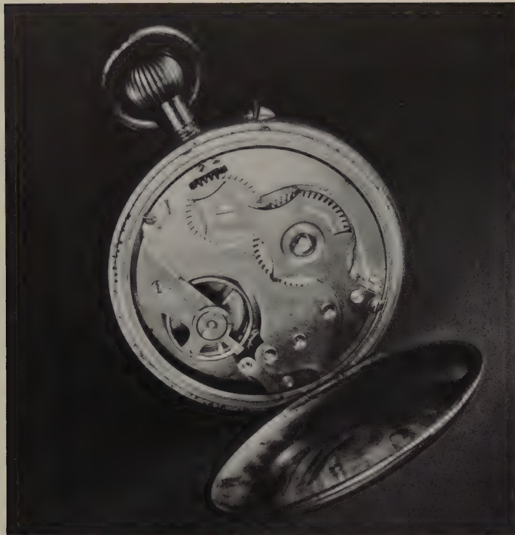
Above: The back of a Roskopf watch. It has no centre wheel and employs steel pins instead of jewels for the escapement pallets.
