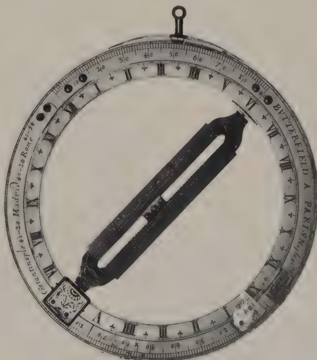
Left : A folded universal ring dial suitable for use at sea. The equatorial ring (inner one with Roman numerals) is turned at right angles to the outer meridian ring. The bridge (crosspiece) is turned flat and to the correct latitude, and the slide with pinhole moved to the correct date. When the instrument is suspended from a cord and a spot of sunlight falls on the equatorial ring, the spot shows local time.
