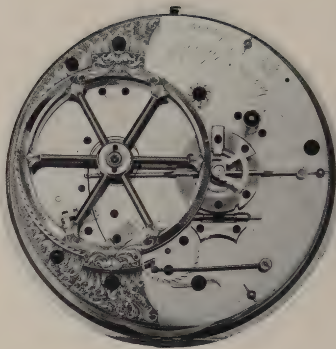
Below : Kendall's third watch, K.3, was practically identical to K.2 except for the escapement and the three separate dials. It was set in a case in gimbals and Cook used it on his third voyage on Discovery.
