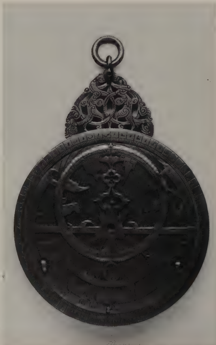
Left: Front of the astrolabe shown on page 31. This is the rete side - a star map - in this case for 38 stars. Normally the rete is set to show star positions by an angle obtained by the alidade on the other side, but because there is a calendar on the back, two perforated projections are provided on this side for sighting.
