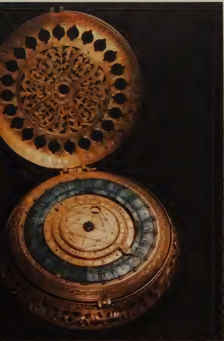
Left : A late Renaissance travelling alarm clock made in Lübeck by Nicolaus Siebenhaer. The small knobs on the outer double-XII chapter ring are touch knobs for finding the time in the dark. Inside is a 1-24 ring of Arabic numerals, then a double-XII ring.
