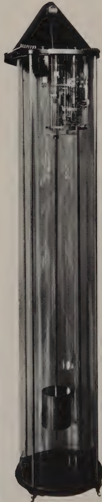
Left and right : The Shortt free pendulum in its low pressure chamber on the left and the slave pendulum with which it is associated on the right. This is a converted Synchronome clock.
