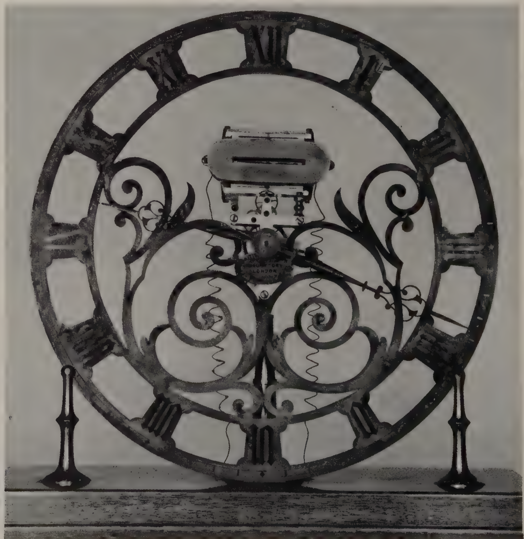
Below, left and right: The electric master clock and slave dial made by Wheatstone’s company, the British Telegraph Manufacturing Co., in about 1870. A pendulum with a coil for a bob behaves like a generator of alternating current to drive the slave.
