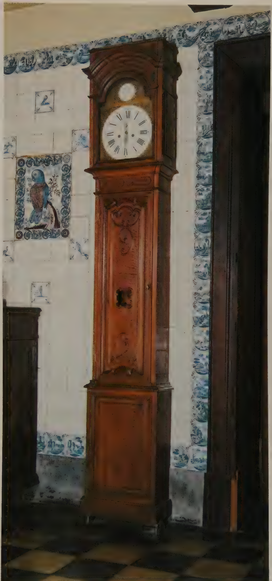
Right: A Belgian version of the longcase clock, made about 1750 by Gilles de Beefe, Liège, in the English style. It has an anchor escapement and long pendulum and the lever in the dial arch is to silence the striking.
