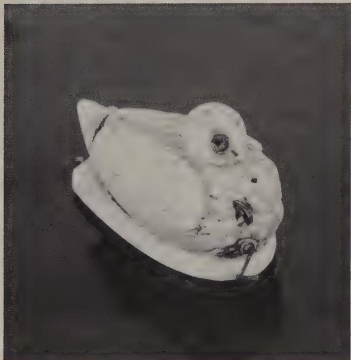
Below: A miniature portable compass dial in the shape of a duck. The compass helps to align it north-south to read the shadow.
