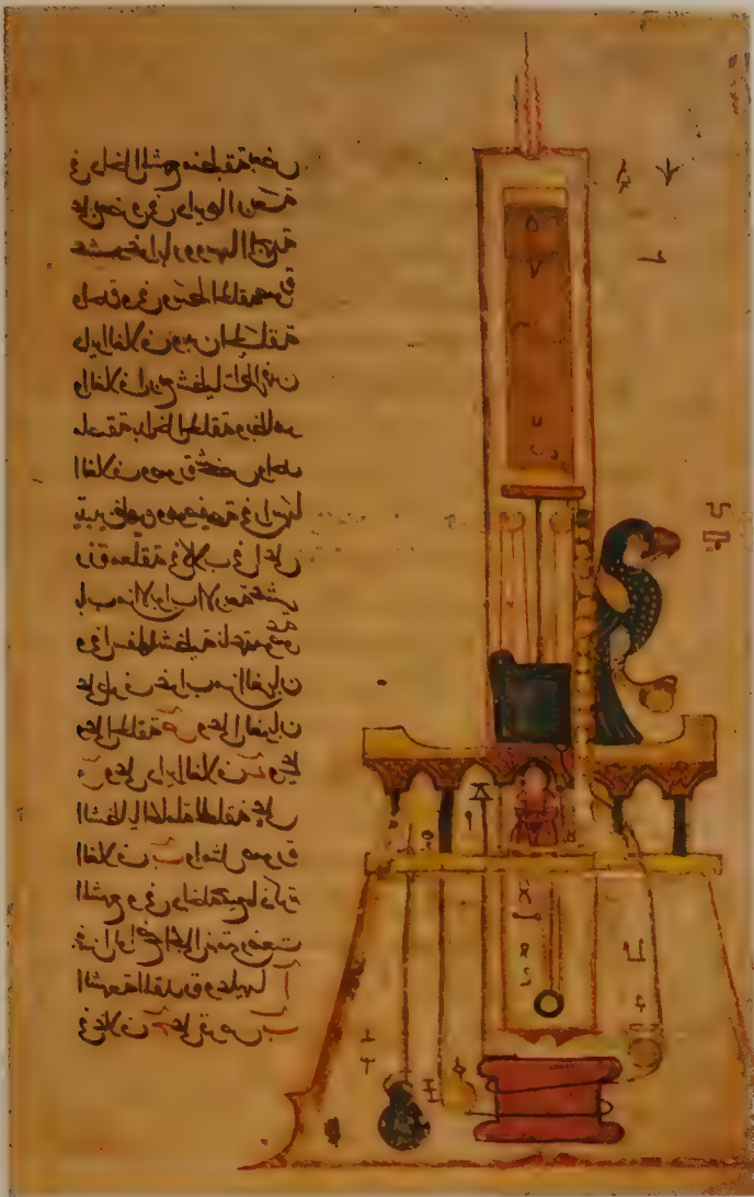
Above : Another illustration from 'The Automata', with some of the text. It shows the clock of doors, which has a candle at the centre and 14 doors around the candle holder. When an hour had passed from lighting the wick, a ball fell from a falcon's beak, the door opposite opened and a figure emerged. At each hour a different door opened.
