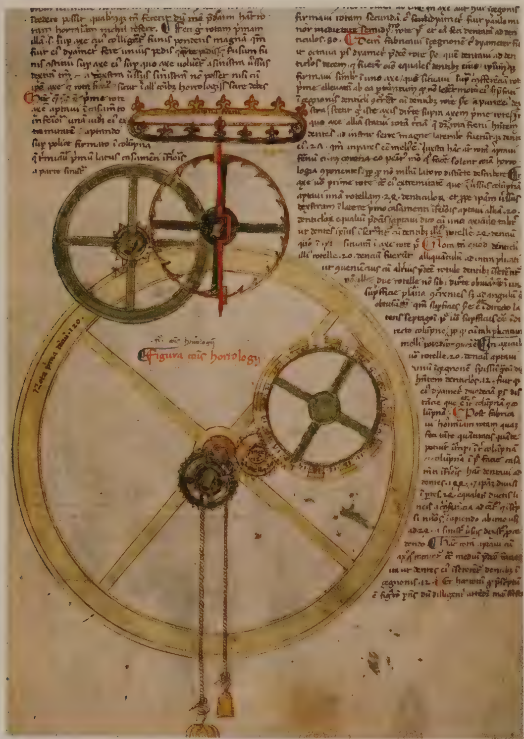
Below: A fourteenth-century copy of 'Il Tractus Astarii', in which Giovanni da Dondi described in detail the construction of his planetary clock of 1348–64. The drawing below is by far the earliest of a clock escapement, showing the crown wheel and the balance, which is also like a crown.
