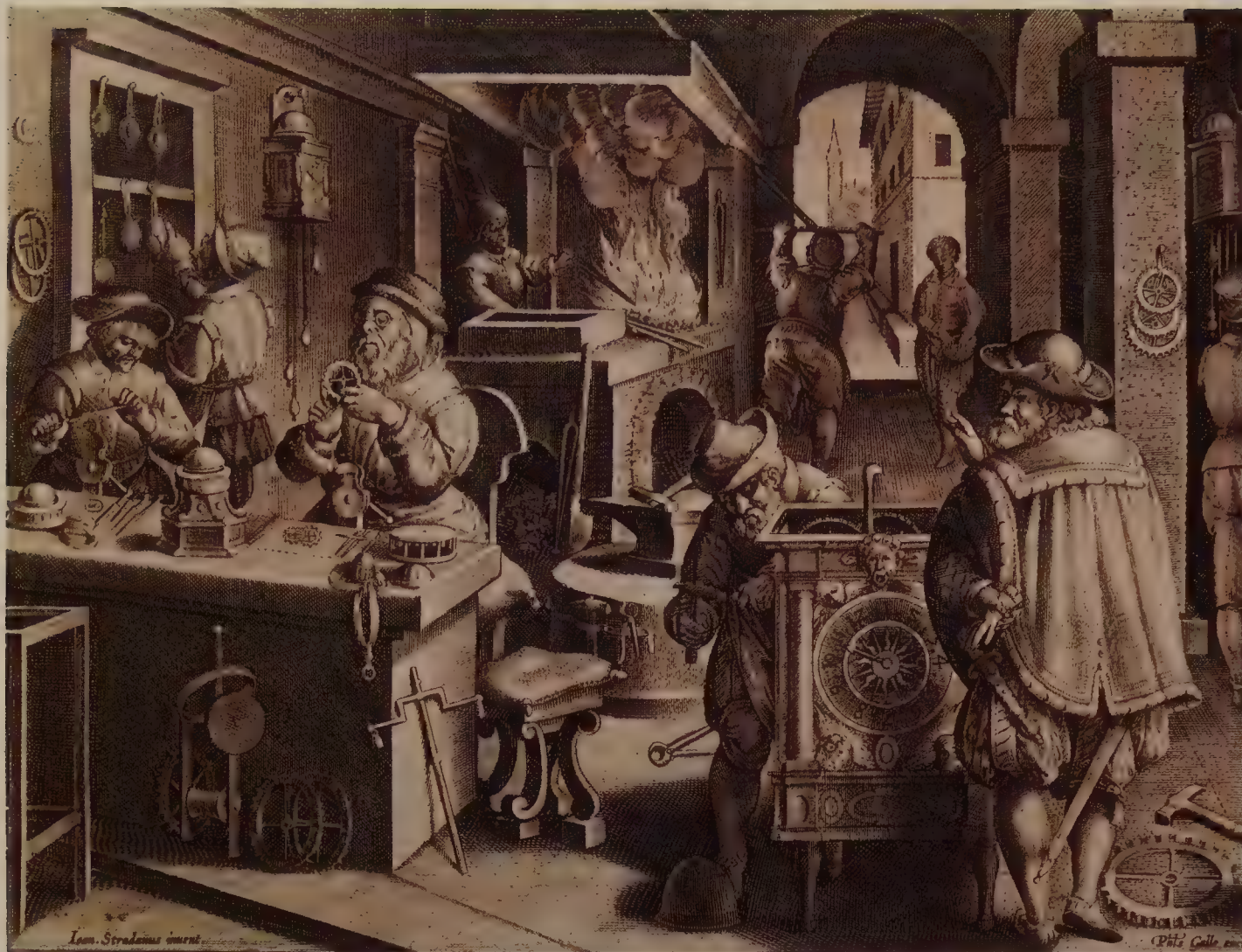
Left: A sixteenth-century engraving of a clockmaker's workshop in Flanders, attributed to Stradanus. There is a forge in the background, but no bench for the making of parts by sawing and filing is shown. Weight-driven clocks and watches hang from the walls. A watchman's clock and a verge and foliot are propped up against the bench.
