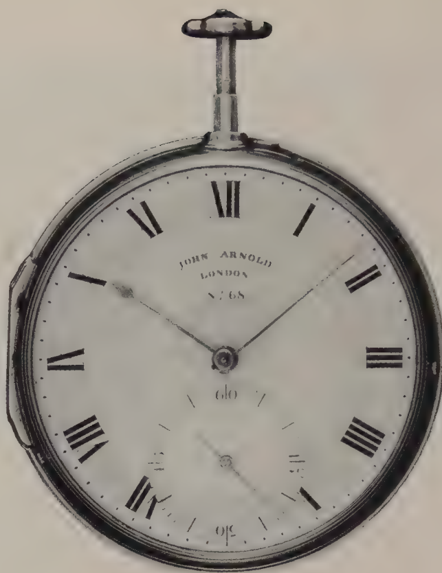
Right: A marine chronometer by John Arnold and Son, dated between 1787 and 1799, in a box without an inner case. It is under-sprung (the balance is between the balance and the plate), unlike the usual arrangement of spring on the outside.
