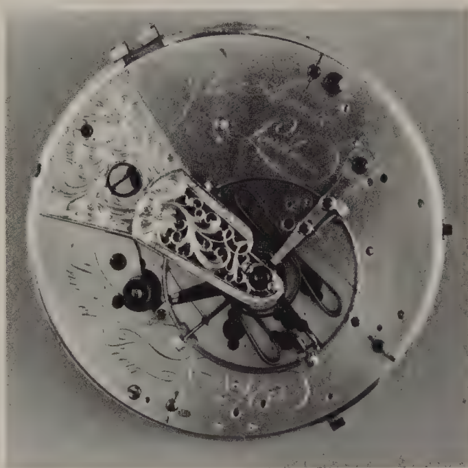
Left: Back plate of the Arnold pocket chronometer. The balance is Arnold's so-called double-S type, which refers to the shape of the bimetallic strips used for temperature compensation. He also used various other shapes.
