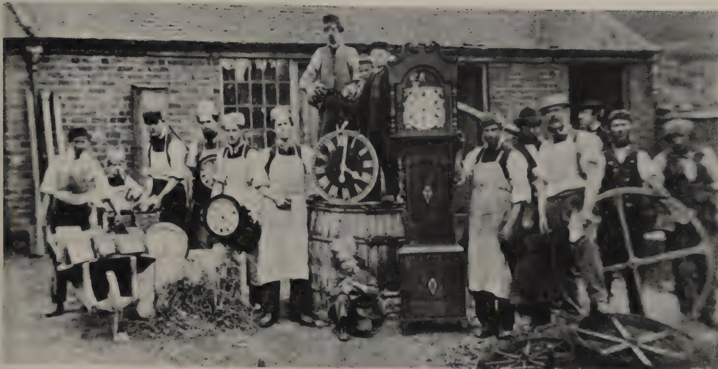
Left : The staff of Ashbourne, Derby, England, packing clocks into a crate in about 1865. The firm made longcase and skeleton clocks on a batch programme which, as in other small factories of the time, had some unrecognized elements of mass production.
