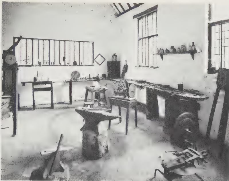
Plate 116 Reconstruction of Samuel Deacon's workshop of 1771 in the Newarkes Houses Museum, Leicester, showing the wheel-cutting engine used by Deacon in 1771.
