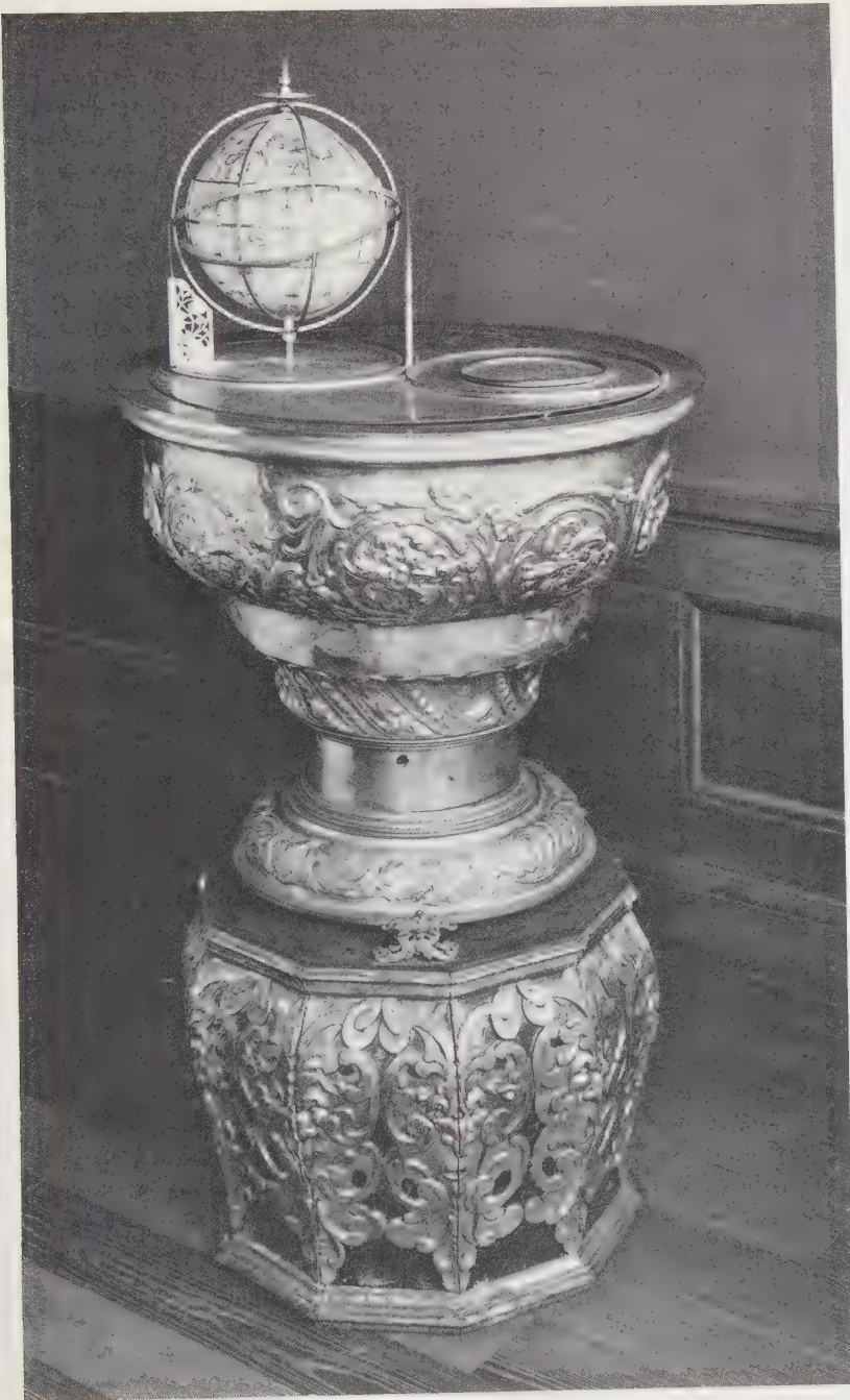
Plate 4 Astronomers were concerned with making working models of the universe which had to be driven by a clock. This Copernican system was made in c. 1651, before the pendulum, for the Duke of Gottorp and is in Frederiksborg Castle, Denmark.
