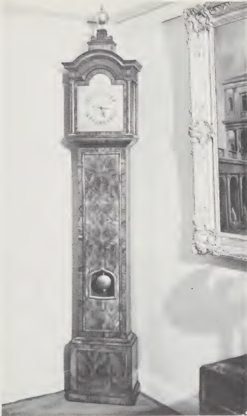
Plate 17 A magnificent Thomas Tompion clock in a walnut case. It has a 24-hour dial and an equation of time dial in the arch, and the movement goes for a year with one winding. It was made about 1695, and has the first known break-arch dial and hood. The anchor escapement is under the movement. Reproduced by gracious permission of H. M. The Queen.
