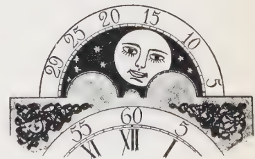
Fig. 24 Moon dial in the arch of a clock, which shows the correct shapes of the quarters. The age is shown by a central pointer at the top (not indicated in the drawing).
