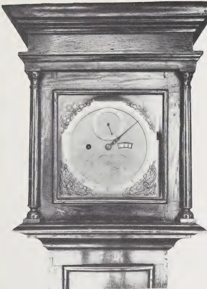
Plate 84 One of the most famous of all regulators, made for the first Astronomer Royal, John Flamsteed, by Thomas Tompion in 1691. It runs for about 35 days, and has a long pendulum beating two-thirds of a second. The dial shows minutes and seconds in degrees of arc. The hours, shown in the aperture, indicate up to 36, also in degrees. ( 360^\circ = 24 hours, i.e. one revolution of Earth.)
