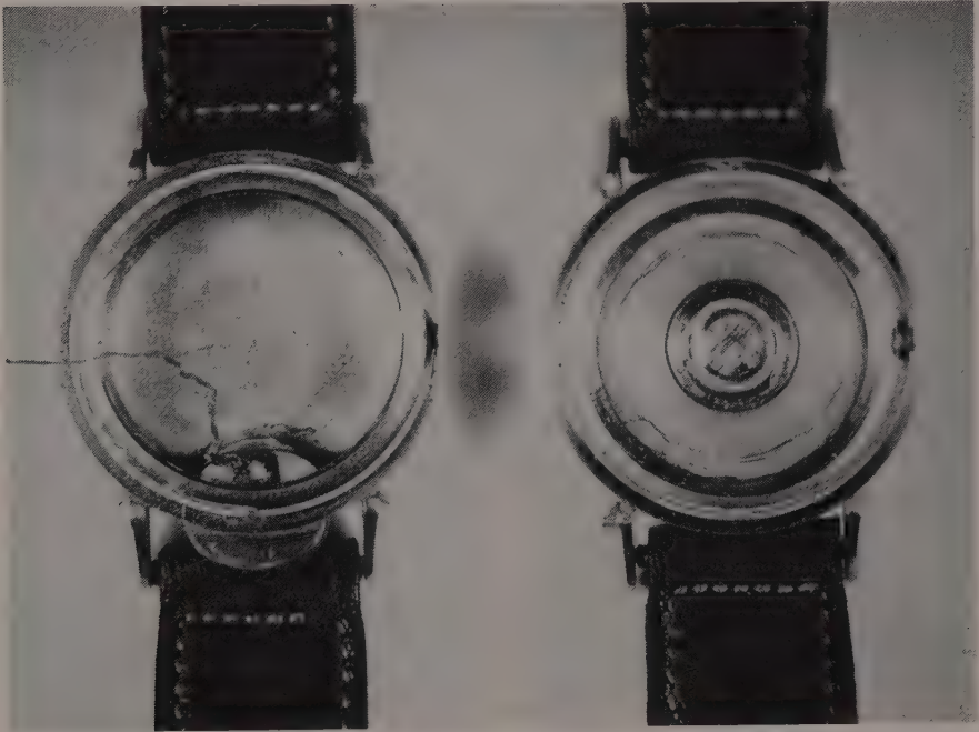
The cases for Mark 3 (left) and Mark 2 (right) illustrate the efforts taken to fit the battery into the case rather than the strap. The case back was deepened to accommodate the battery in Mark 2, making an extremely bulky case when seen from the side.
