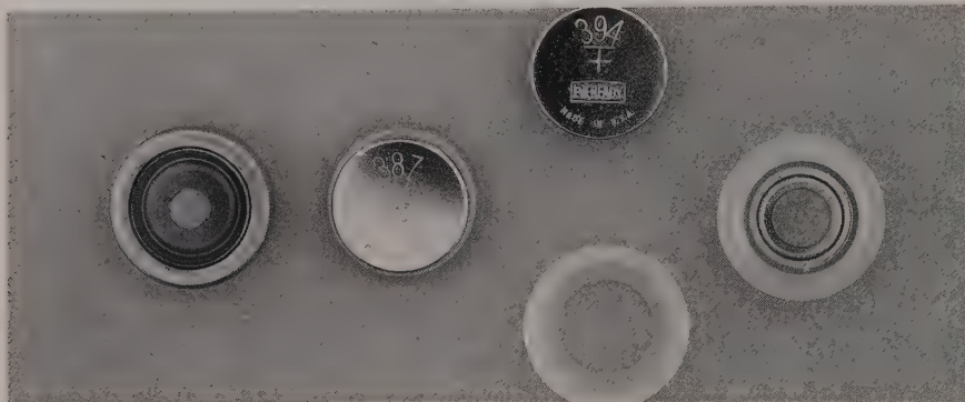
The original 201 battery [left] is no longer produced. A suitable replacement can be made by fitting a 394 battery into the plastic grommet taken from an old 387.
