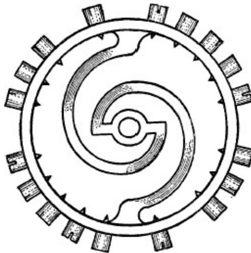
Figure 15A. Wyler shockproof balance.
