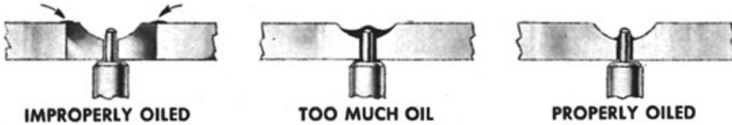
PROPER METHOD OF OILING CAPPED JEWELS
