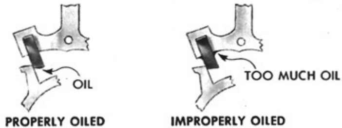
REPRODUCED BY THE PERMISSION OF THE DEPARTMENT OF TUB ARMY Figure 12. Proper and improper oiling.
