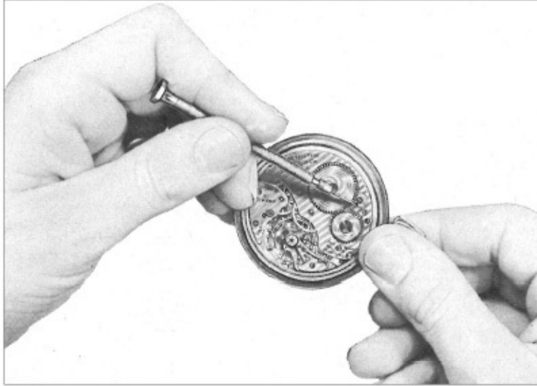
REPRODUCED BY THE PERMISSION OF THE DEPARTMENT OF TUB ARMY Figure 7. Releasing power of the mainspring.
