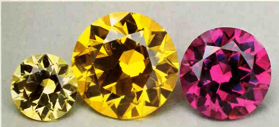
325. SYNTHETIC GARNETS: yellow = dysprosium- aluminum; orange = samarium- gallium; red = neodymium-gallium; all 1-5 carats.
