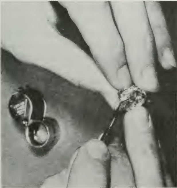
An expert examines a diamond through a powerful magnifying glass—the loupe shown above—to see how the stone can be cut for maximum weight. After studying the stone's imperfections, he marks the diamond where it must be divided. (N.W. Ayer & Son, Inc.)
