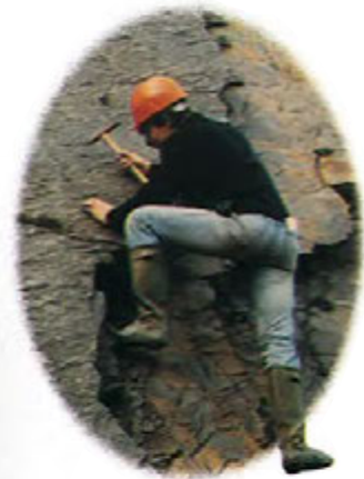
FIELDWORK Use a geological hammer to collect in the field. Wear suitable clothing and boots, a hard hat, and eye protector. Ask permission to collect on private land and always observe the local laws.
