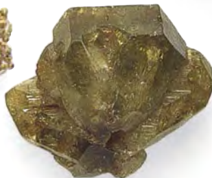
CHRYSOBERYL CRYSTAL Crystal system: orthorhombic; hardness: 8.5; specific gravity: 3.68–3.78.
