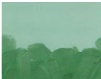
The liquid cools rapidly. Stubby, cloudy prismatic (p. 23) crystals form.
