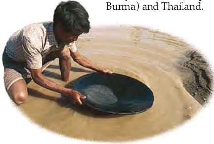
Panning for gold in the Irrawaddy River, Myanmar. The prospector looks for the glint of gold grains within the waste.
