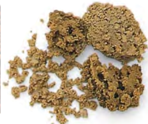
KETTLE FUR Crystals can be found in your kettle. Even after purification processes there are still some harmless minerals dissolved in tap water. These crystallize and coat the inside of your kettle when the water is boiled.
