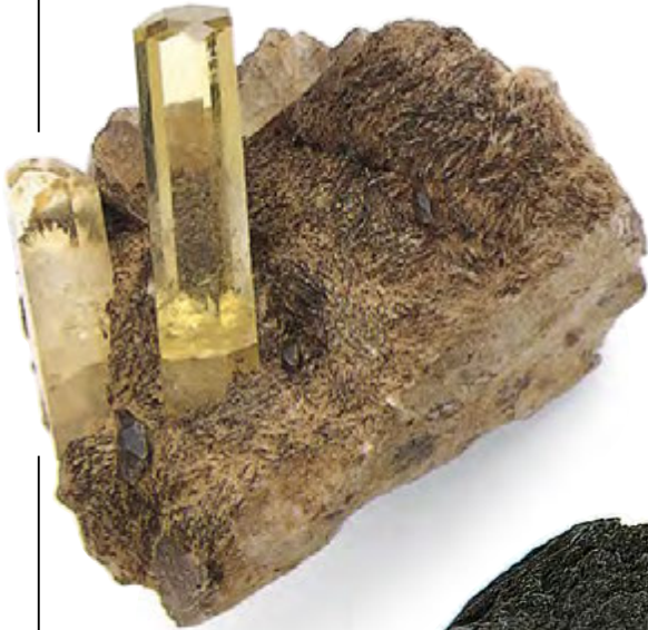
BERYL CRYSTAL Crystal system: hexagonal; hardness: 7.5; specific gravity 2.63–2.91.
