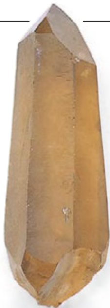
QUARTZ CRYSTAL Crystal system: trigonal; hardness: 7; specific gravity: 2.65.
