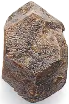
ZIRCON CRYSTAL Crystal system: tetragonal; hardness: 6–7.5; specific gravity: 4.6–4.7.
