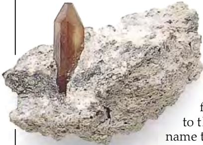
TOPAZ CRYSTAL Crystal system: orthorhombic; hardness: 8; specific gravity: 3.52–3.56.
