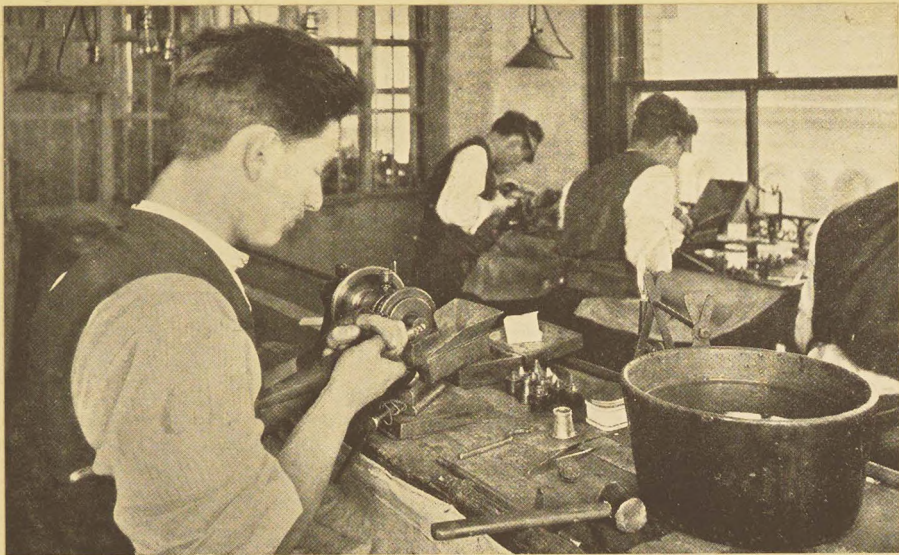
DIAMOND-CUTTING LATHE WITH CUTTER AT WORK, SHOWING THE MANNER OF CUTTING A DIAMOND
