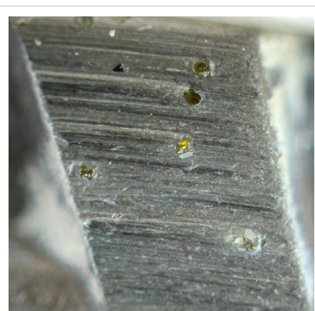
Close-up photograph of an angle grinder blade with tiny diamonds shown embedded in the metal
