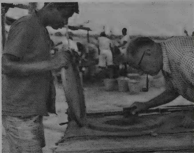
Fig. 4.7. A sieve, twisted in water to bring diamonds to the centre of a pile of concentrate, has here been upturned to empty its contents on the picking table, with heaviest material at the top in the centre.
