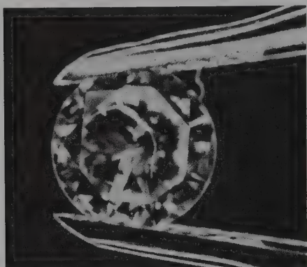
Fig. 13.36 Crack under the table.
