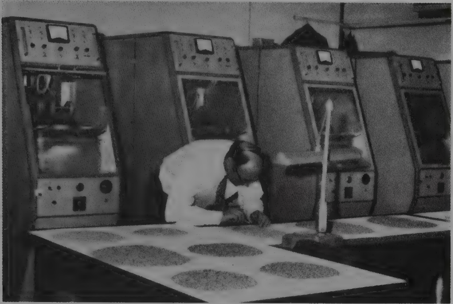
Fig. 5.12. Optical separation units, which are similar in principle to X-ray units.
