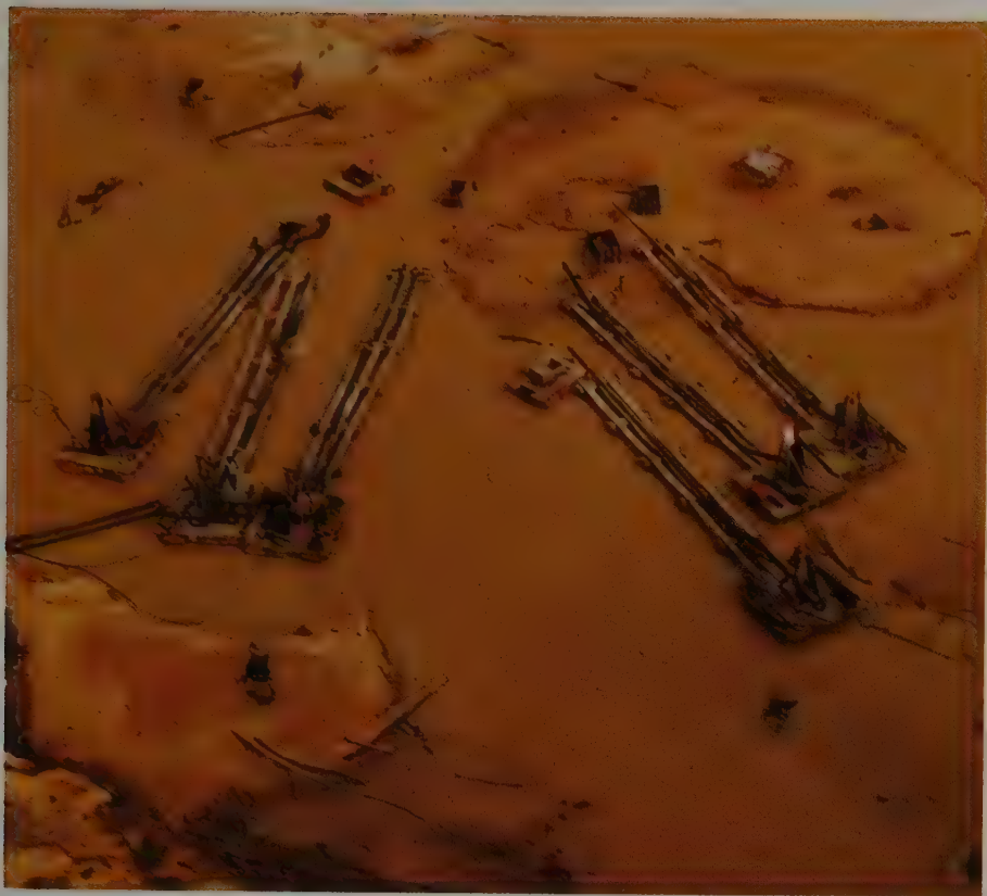
Air lifts on the Sewa River in Sierra Leone, part of the alluvial mining operation two miles south of the confluence. Diamond areas extend to the north-east into Guinea.
