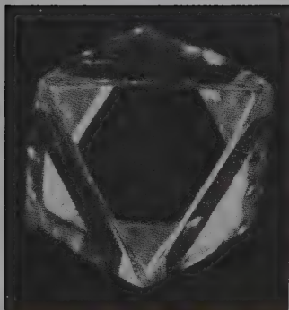
Fig. 1.7. A natural octahedral diamond crystal of the type called a glassie which was sometimes set in jewellery.
