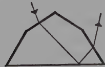
Fig. 10.15. Light passing through a portrait stone. Fig. 10.16. (centre) Light internally reflected from the back of a theoretical rose-cut stone. Fig. 10.17. Light internally reflected more towards the front of a rose-cut stone.
