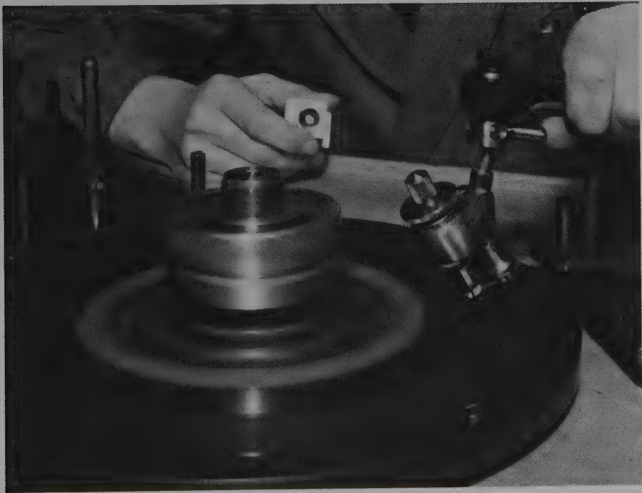
Fig. 11.25. A modern scaife with ball-bearing mounting instead of a top pivot, in use in Belgium. The mechanical dop is also of modern adjustable design.
