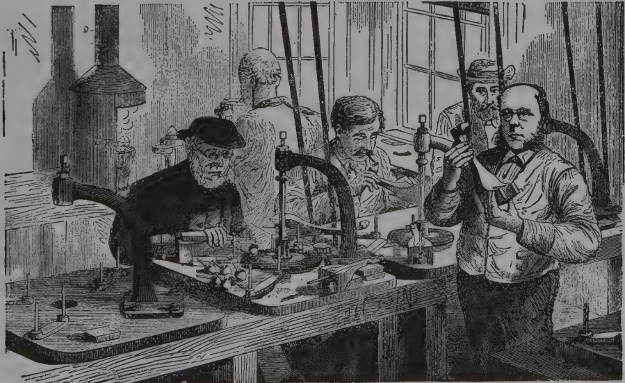
Fig. 9.12. Another polisher's workshop of later nineteenth century. The pins at the ends of the bars fixed on the benches (left) are to prevent tangs from being swept off the rotating scaifes. The tang is placed between the pins.
