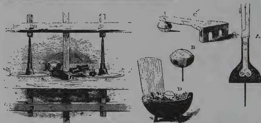
Fig. 9.11. Diamond polishing equipment in mid-nineteenth century. The scaife spindles are running in blocks of the hard wood, lignum vitae (as in Fig. 9.10). Top right is a tang with dop fitted and right a tang showing the tail. The brazier in the centre was to melt the solder in the dop, which holds the diamond being polished and is like an acorn in its cup.
