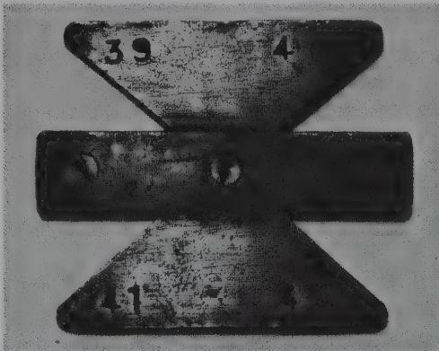
Fig. 11.35. The extremely simple gauge used by most diamond polishers to make sure that the pavilion angle to the girdle is as required.
