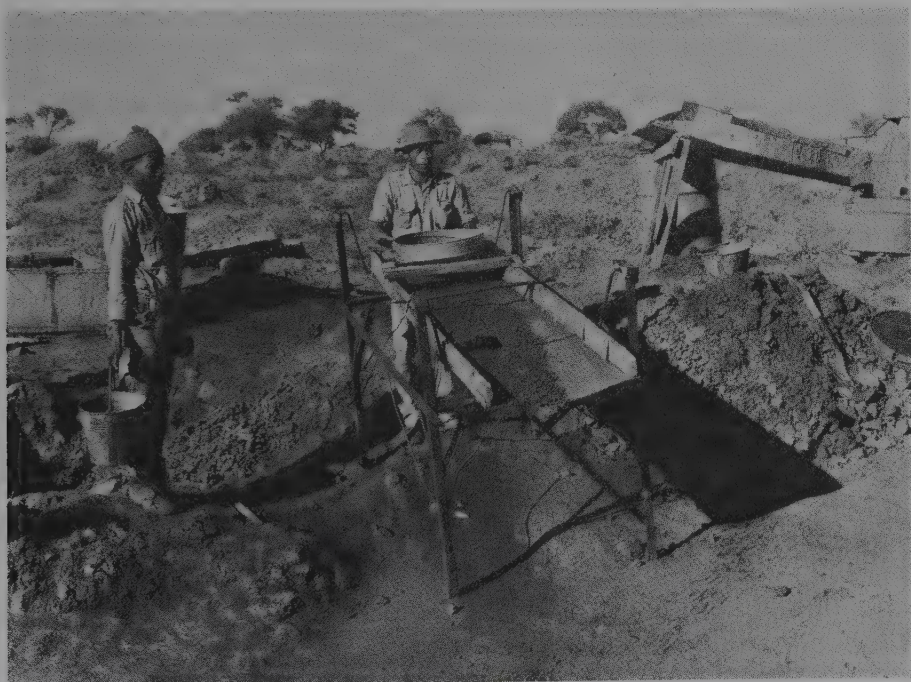
Fig. 4.4. A form of rocking cradle to separate smaller pebbles including diamonds from larger ones.
