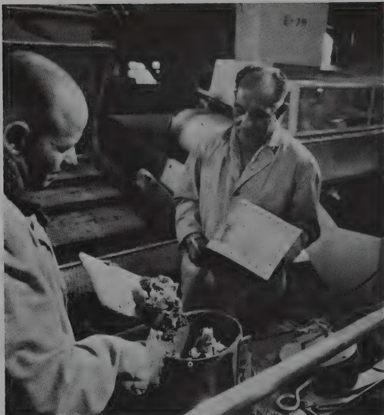
Fig. 5.8. After the grease on a grease table has trapped diamonds it is scraped off and put into drums. The grease is boiled off to leave the diamonds and other material that might have been trapped.
