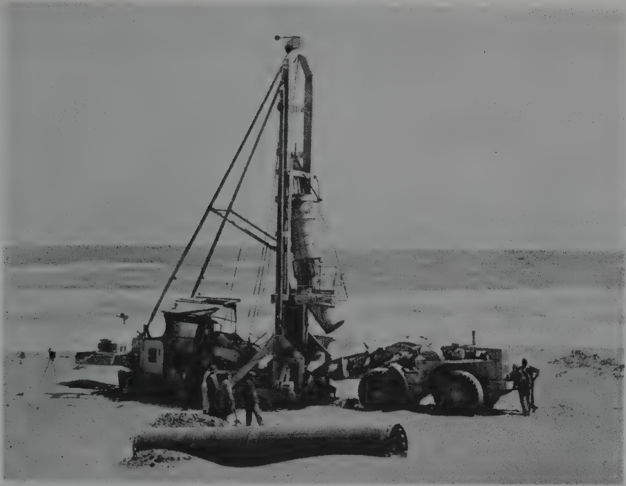
Fig. 6.9. Foreshore prospecting by Consolidated Diamond Mines of South West Africa. A Benoto drill is in action accompanied by a front-end loader on the right.
