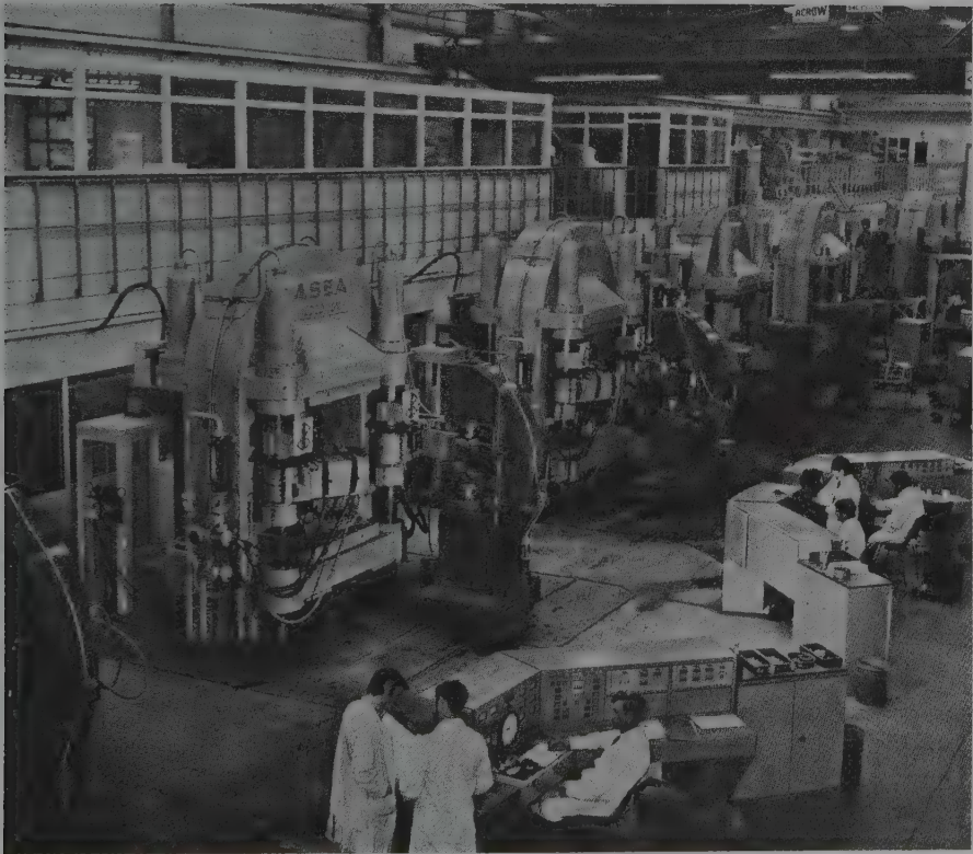
Fig. 19.7. Presses and control consoles for the commercial production of synthetic diamonds at De Beers' plant at Shannon, Eire.
