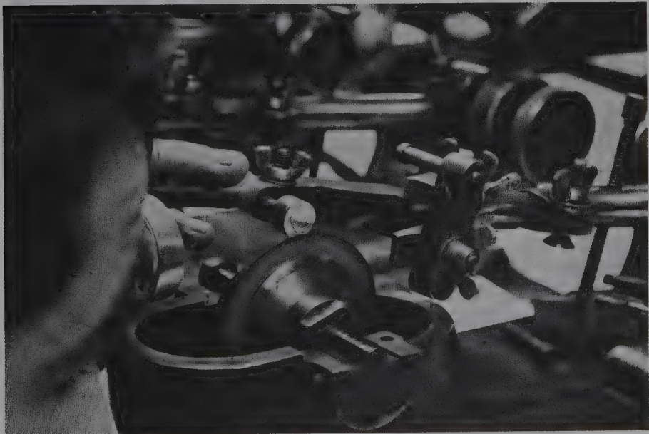
Fig. 11.16 Adjusting a machine to saw an octahedral crystal in a cube plane. The Indian ink mark made by the designer can be seen. On the right edge is a long screw that acts as a stop. It is adjusted so that the diamond is cut in a number of stages.
