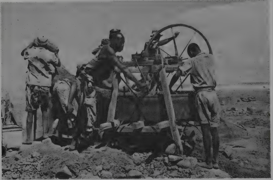
Fig. 4.21. The original form of washing pan, which floated off most of the lighter material and caused diamonds and other heavy material to settle in the bottom.
