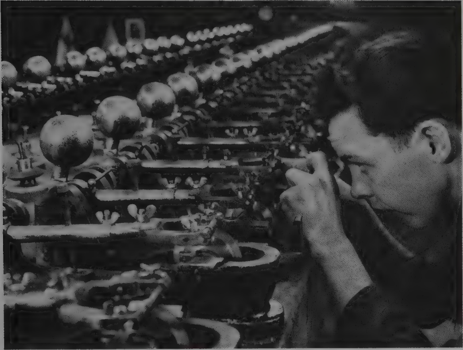
Fig. 11.15 Banks of sawing machines in the works of A. Monnickendam Ltd at Brighton, England. One man attends to a bank of machines.
