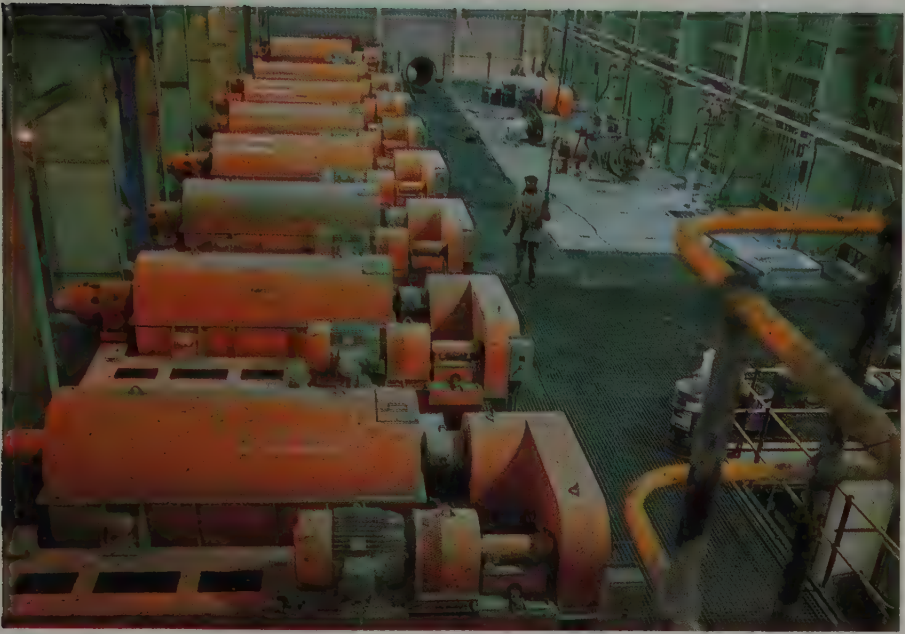
Milling in rotating drums, as seen here at Letseng-la-Terai, is sometimes a convenient part of the extraction of diamonds by grinding down and washing away softer materials.
