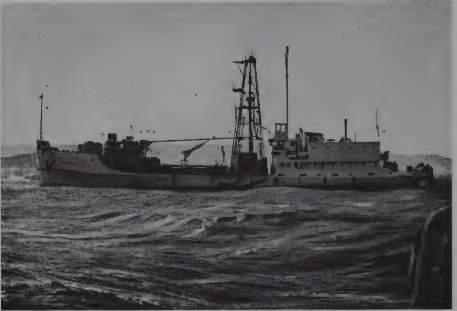
Fig.6 .10. Rockeater, the diamond prospecting vessel under contract to De Beers which is equipped to search for diamond deposits on the sea bed off the South West African coast.
