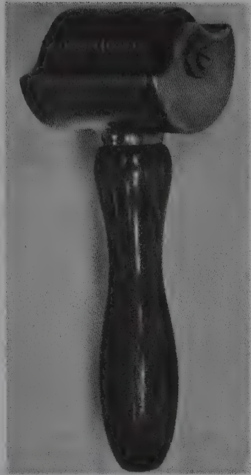
Fig. 11.18. The roller used to apply diamond dust in oil to the edge of the sawing wheel.
