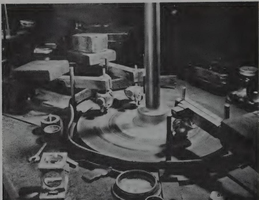
Fig. 11.24. Three diamonds being polished at the same time in mechanical dops. All the tangs are weighted. The scaife is of the traditional pattern. In the foreground, left, is the kind of folding lens favoured by diamond polishers.
