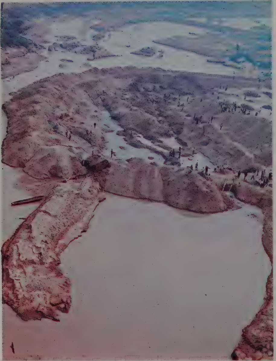
Panning, coffer dams, and air lifts, which are used for transporting diamond-bearing gravels from the Bafi River bed here, in Sierra Leone, to a more convenient place for concentration.
