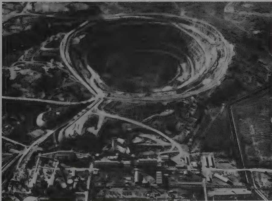
Fig. 2.21. Koffiefontein today. Underground working began in 1977-8 by a long-hole chambering method. By 1981, open-cast operation will be phased out.
