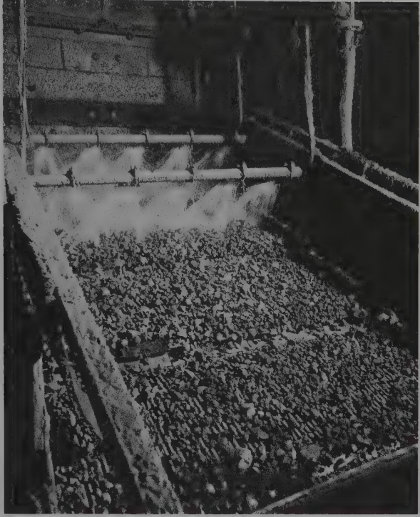
Fig. 5.4. Part of the screening and washing section of a treatment plant. From some screens the fraction that passes over is waste and from others the fraction that passes through is waste.
