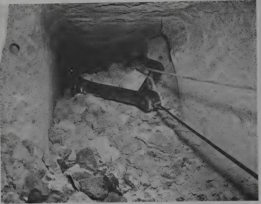
Fig. 4.31. The actual stirrup that draws the blue ground through the scraper drift. On the right and left can be seen a draw points through which broken blue ground has come from the pipe.
