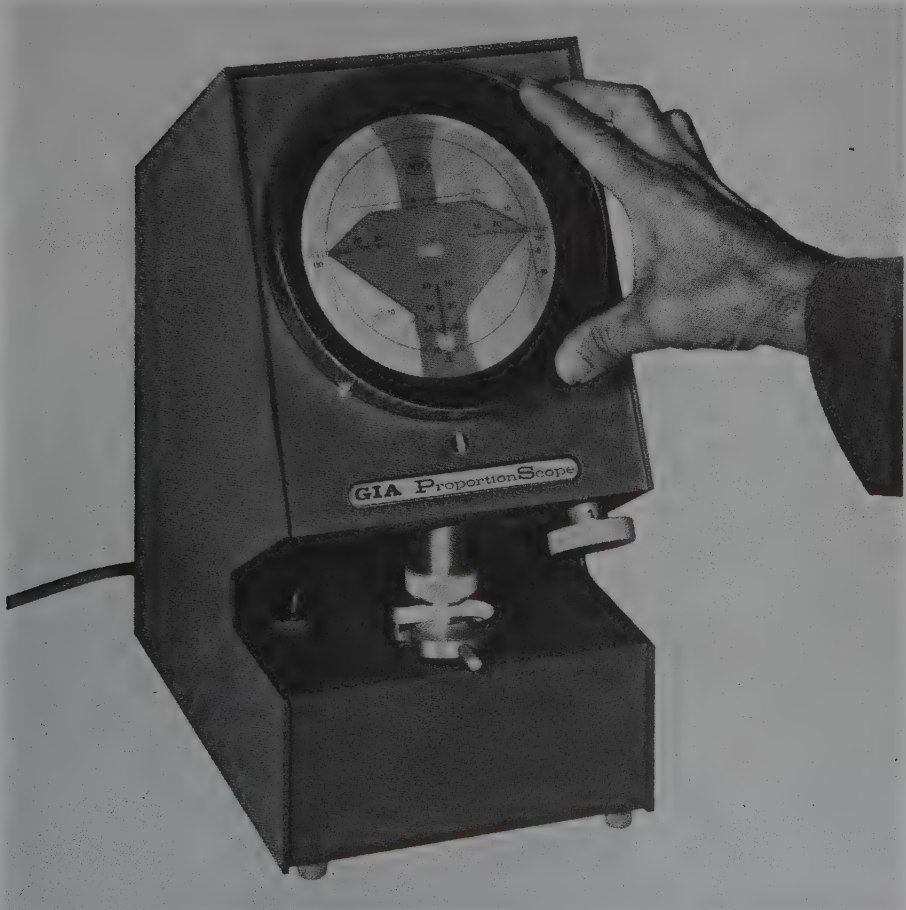
Fig. 14.10. The G.I.A. ProportionScope with the shadow of a diamond under test on the scaled screen.
