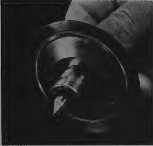
Fig. 11.17. The phosphor bronze wheel, in its spindle, used for sawing.
