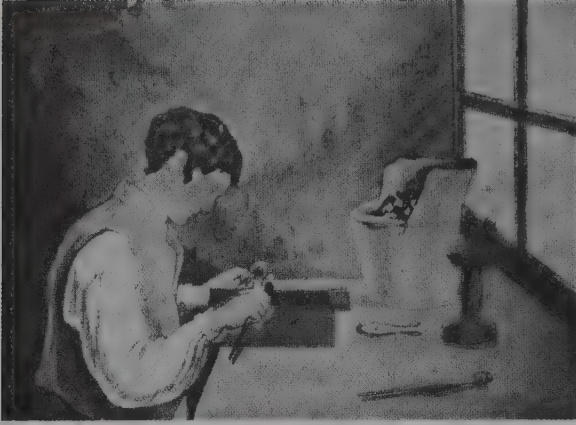
Fig. 9.7. The bruter (cutter) at work, from Mawe's book of 1823. The box receives powder produced. On the right is a charcoal fire to soften the cement for fixing diamonds in the sticks. This method is also used to produce a notch or kerf (Fig. 9.11) for the cleaving blade.
