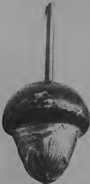
Fig. 9.13. A solder dop which was in use until 1975. It is identical to those used centuries ago and still in use today. The copper stalk is bent to achieve the correct facet angle.
