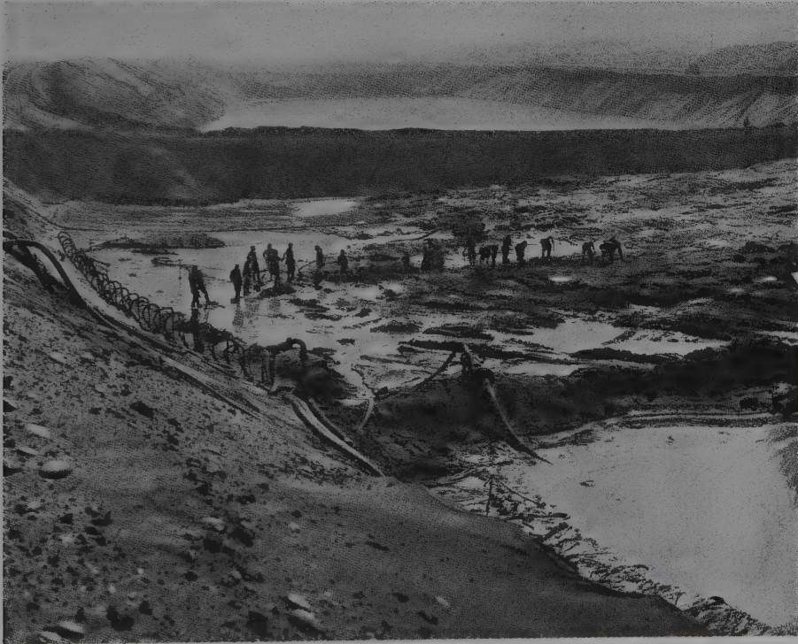
Fig. 4.48. A gang searching the remaining gravel after most of it has been removed from the paddock to the treatment plant.
