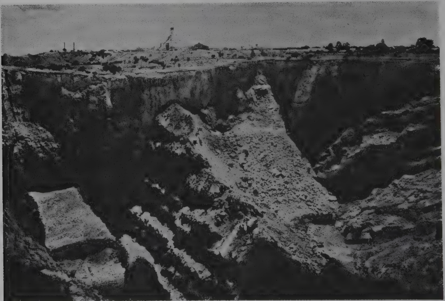
Fig. 4.36. The Premier mine where a combination of surface and underground methods called benching is used.
