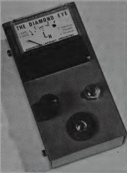
Fig. 21.11. A new reflectivity comparator, introduced by Hanneman in 1978. It is designed to separate diamond from its nearest simulants (zirconium oxide, Y.A.G., strontium titanate and G.G.G.) quickly.
