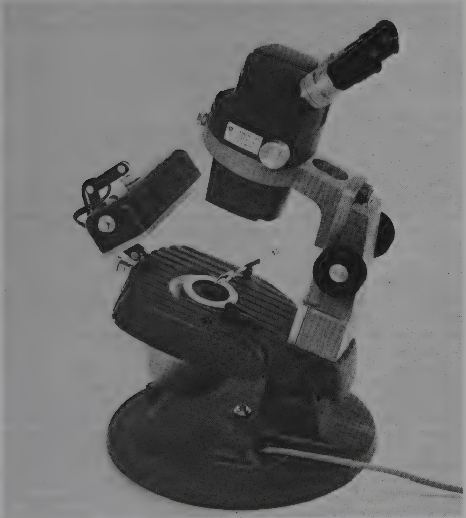
Fig. 13.6. The Gemolite, an effective 10\times binocular microscope for diamond grading supplied by the Gemological Institute of America. The diamond is held in the removable clip seen on the stage, under which is dark field illumination. Over the stage is a colour grading lamp. A zoom lens is incorporated and there are other fittings including a special eyepiece for proportion grading.
