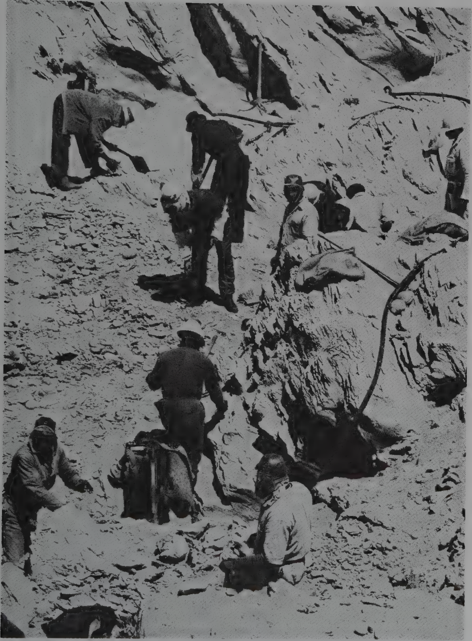
Fig. 4-39. Potholes in the bedrock trap heavy materials, including diamond, and have to be cleared by hand. Final clearing is done by a small brush, being used top left.
