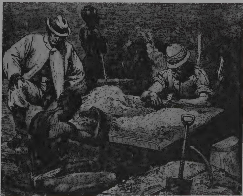
Fig. 2.17. Sorting gravel at the early river diggings. The gravel does not seem to have been washed or concentrated with much skill or care.
