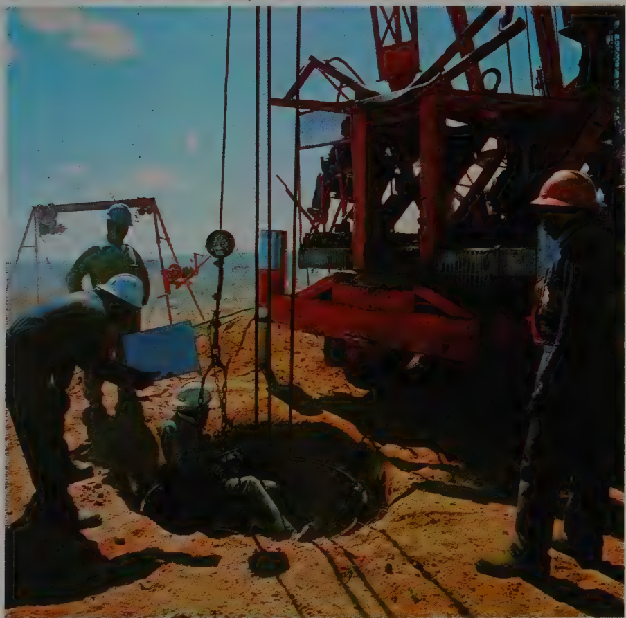
Sampling is an extra important activity when mining is geared to demand for particular sizes and qualities. Pits for sampling are drilled and liners inserted, as shown here, or dug.
