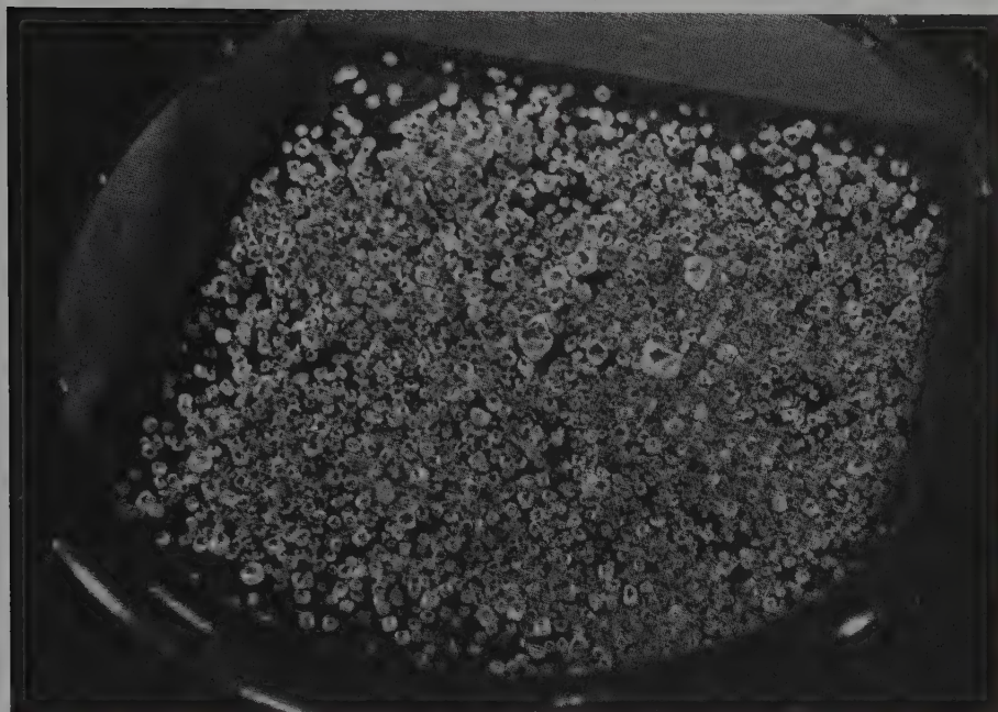
Fig. 5.14. One day's output of diamonds from Consolidated Diamond Mines of South West Africa. About 90 per cent are of gem quality and the total is about 5,600 carats.
