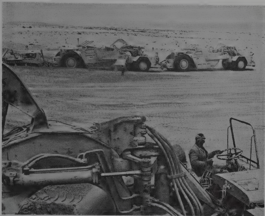
Fig. 4.37. Removing sand by scrapers and bull-dozers on the beaches of South West Africa on the Consolidated Diamond Mines concession. Similar methods are used south of the Orange River at Kleinzee Annex and Dreyers Pan.
