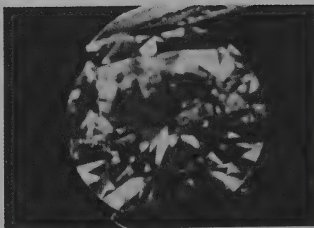
Fig. 14.6. Dark-centred or lumpy stone with an over-angled pavilion.
