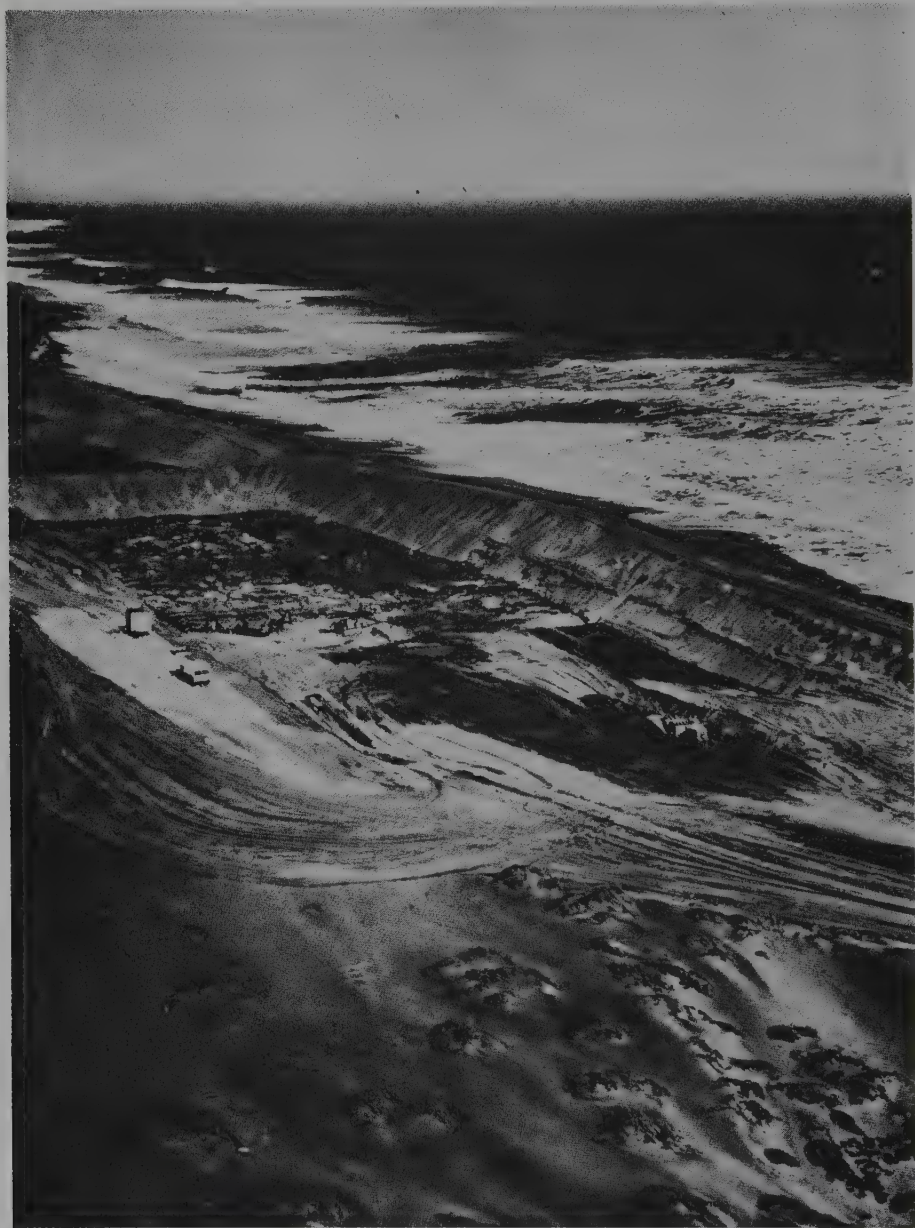
Fig. 4.47. Mining in the tidal strip by building dams before removing overburden. Two of the series of dams seen on the far left have been worked out and allowed to flood.
