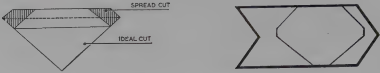
Fig. 11.1. How a brilliant cut is spread to gain weight and increase diameter which results in an overdepth pavilion. A stone can be cut with correct angles, as here, but with a correct depth of pavilion and a table which is too shallow. Fig. 11.2. (right) How a brilliant can be cut from a macle.
