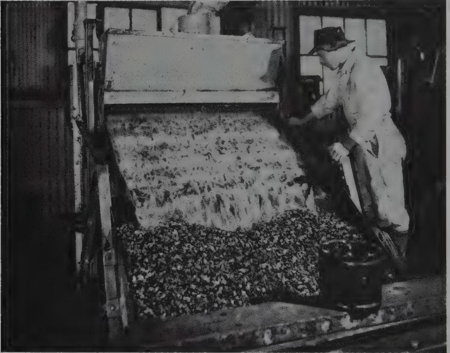
Fig. 5.1. Most diamonds cannot be wetted, neither can grease. If diamond-bearing concentrate is sluiced over a sloping and vibrating table covered with grease, diamonds stick to the grease and the rest of the material is carried off the bottom of the table as waste. Some concentrate has to be given a previous treatment to make the diamonds non-wettable.
