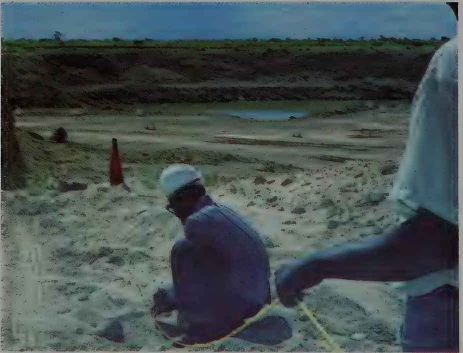
Blasting is often part of open pit as well as underground mining, when the mine is a pipe. Here a fuse line is being laid by Debswana workers in Botswana.
