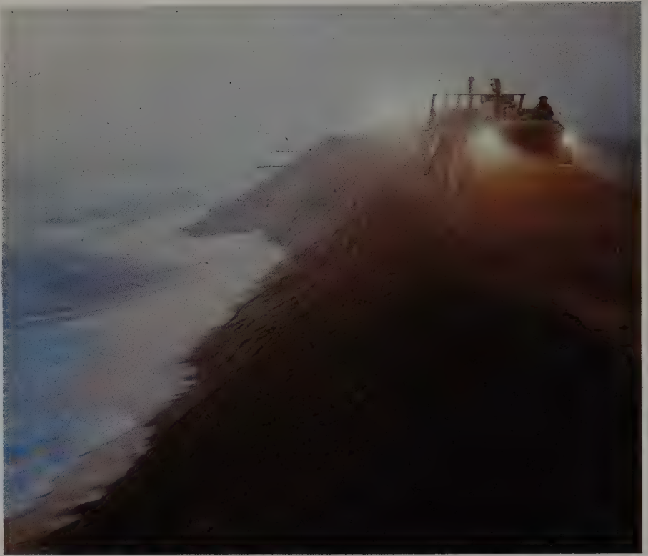
Wall-throwing—creating a sand wall to make a paddock that will last long enough to mine out an area in the tidal strip in the diamond territory being worked by C.D.M. in Namibia.
