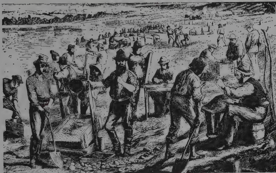
Fig. 4.3. Diggers on the banks of the Vaal river in the early days. On the left two boxes are being used as a rocking sieve where gravel is also washed. In the centre and on the right are picking tables.
