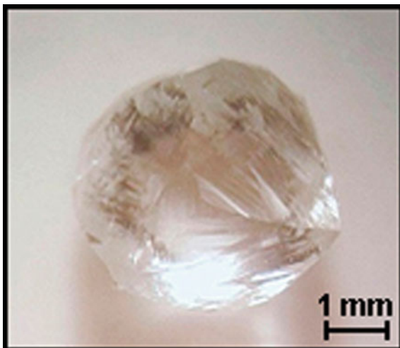
Fig. 6.52 Plastic deformation; crystals with shagreen
