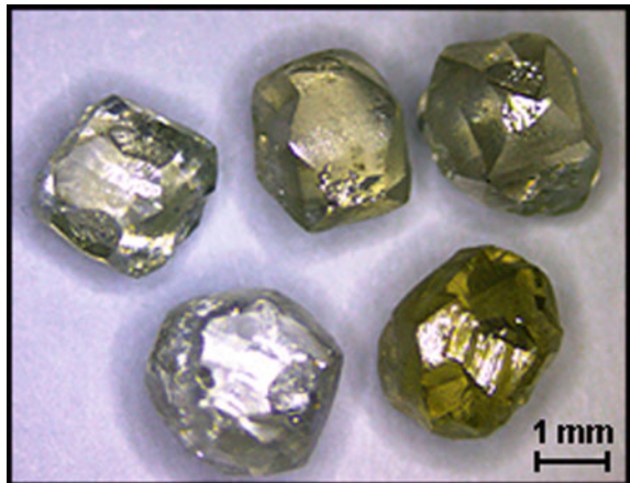
Fig. 6.44 Fibrous growth (striation along the normal to the face) on crystals of cubic habitus
