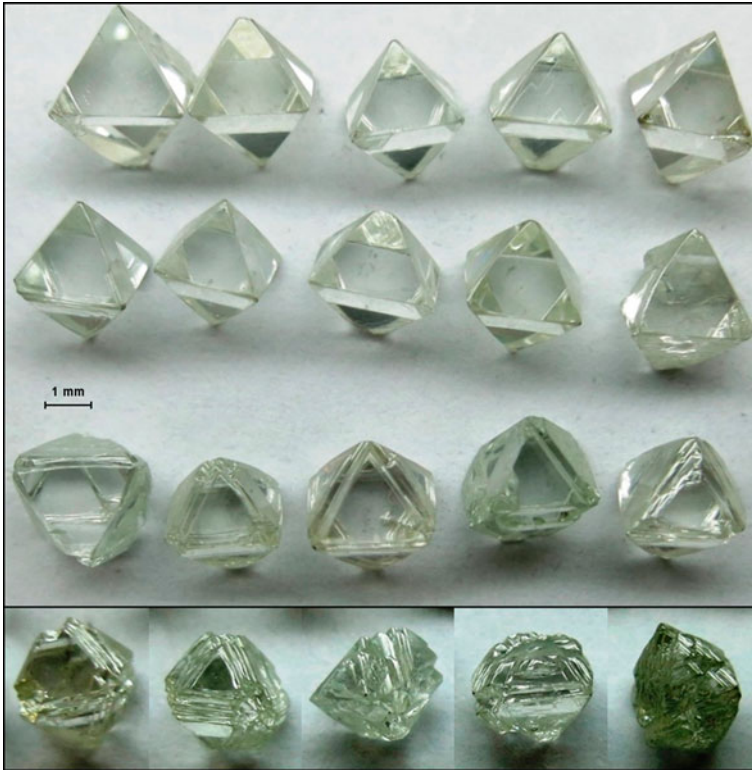
Fig. 6.10 Crystals with varying degrees of lamination from a thin-layered octahedron to a pseudocube with significant layering
