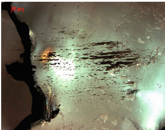
Fig. 3.7 Graphite marks an intergrowth border in two-crystal aggregate, forms separate plate-like inclusions oriented parallel to the diamond's plane {111} (sp. A85). Optical microscope, transmitted light
