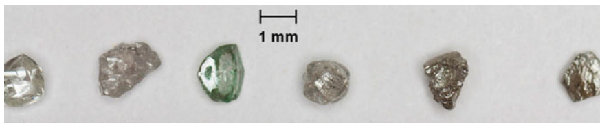
Fig. 4.20 Chips and splinters of curve-faced crystals from the X-ray luminescent separation tailing collection
