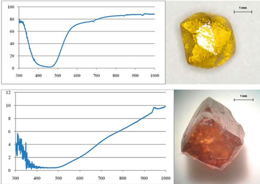
Fig. 2.10 Visible absorption spectra, colored diamonds: straw-yellow (5C, cape) and amber-yellow, orange (colored), cubic and tetrahedral habits
