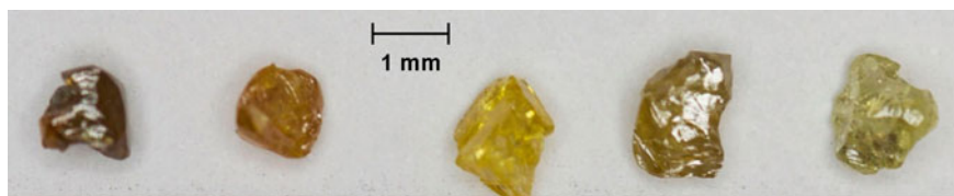
Fig. 4.17 Chips of cubic habit crystals (variety II) from the X-ray luminescent separation tailing collection
