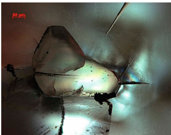
Fig. 3.8 The aggregate of two colorless forsterite crystals and plate-like graphite inclusions confined to them and evolving by cracks (sp. A57). Prepolished specimen; optical microscope, transmitted light
