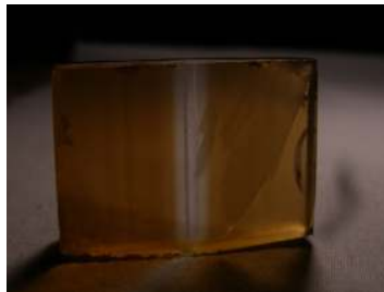
Photo 6.1c. Colourless seed plate and colour zoning in synthetic citrine.
