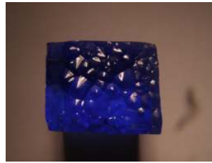
Photo 6.1y. Growth hillocks on synthetic blue quartz.
