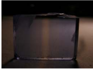
Photo 6.1x. Seed plate in synthetic blue quartz.
