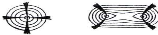
Figure 1.2. Uniaxial (to the left) interference figure. Biaxial (to the right) interference figure if both optic axis is seen otherwise only half is seen.
