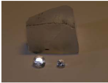
Photo 6.1e. In the back a rough synthetic rock crystal and in the front, to the left a faceted natural rock crystal and to the right a faceted synthetic rock crystal.
