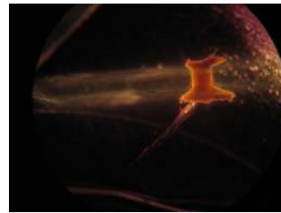
Photo 6.1j. 'Nail head' spicule inclusion in synthetic amethyst.
