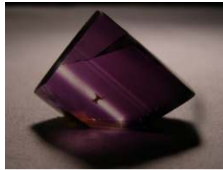
Photo 6.1i. Inclusion, colour zoning and colourless seed plate in synthetic amethyst.
