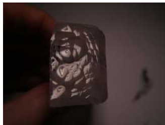
Photo 6.1f. Growth hillocks on synthetic rock crystal.
