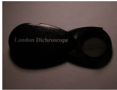
Photo 1.8. London dichroscope from Gam-A.
