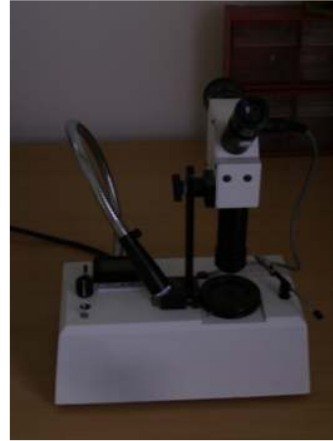
Photo 1.10. The Diascan is a scanning diffraction grating spectroscope produced by the Gem Instrument Corporation. It uses a digital display to indicate spectral wavelengths.
