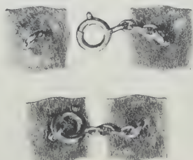
Chain catch, attached and detached.
