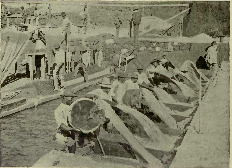
Preliminary concentration of diamond-bearing gravel by dashing water upon it from broad wooden bowls known as bateas. Near Diamantina, Brazil
