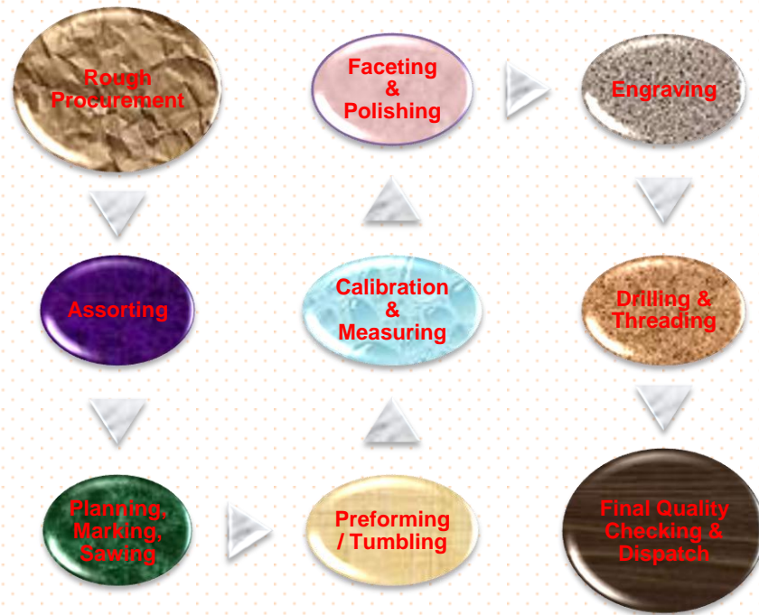
Figure 17: Key processes in coloured gemstone polishing
