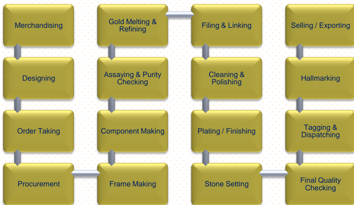
Figure 11: Key processes in handmade and gems-set jewellery manufacturing
