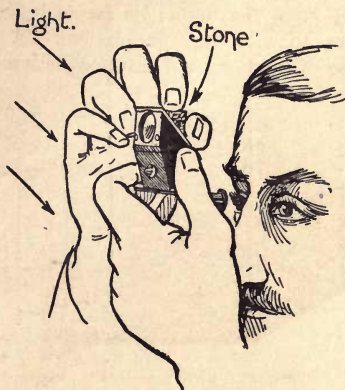
FIG. 17.—Method of Using the Refractometer.
