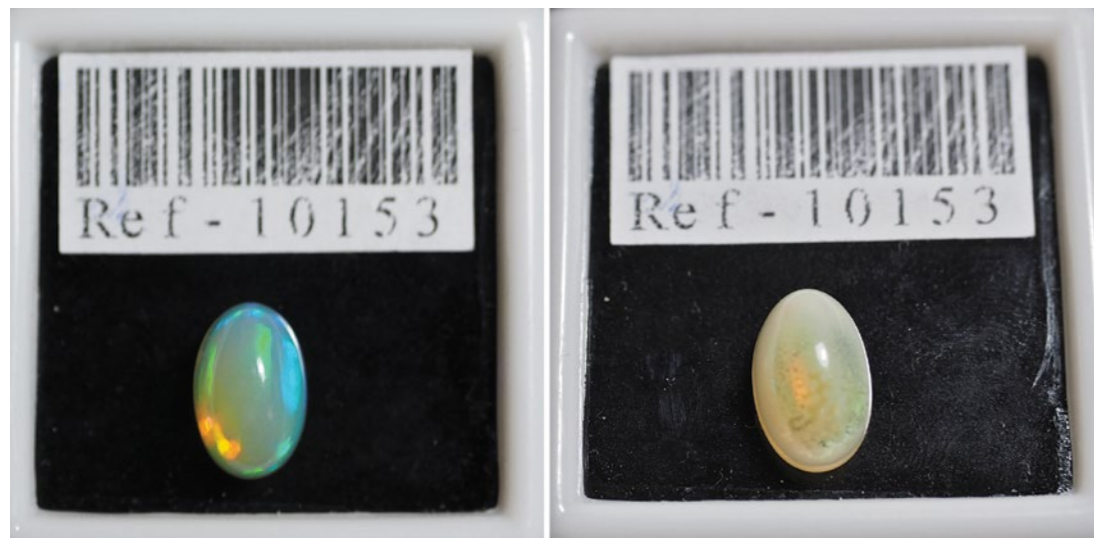
Figure 16. Left: The Ethiopian hydrophane opal before non-branded two-part polyurethane resin treatment. Right: The same stone after treatment that resulted in severe clouding rendering a previously valuable opal worthless.
