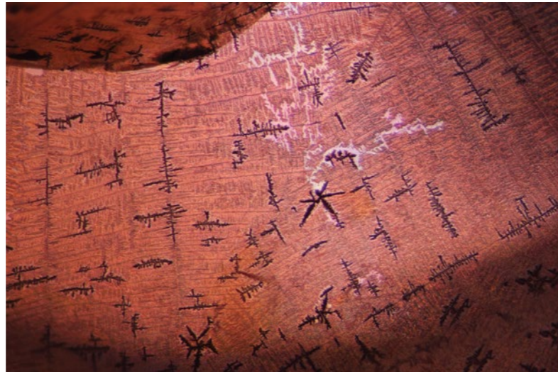
Figure 4. Another view of the filled fissure with its black dendrite inclusions. Photo by Richard W. Hughes/Lotus Gemology.
