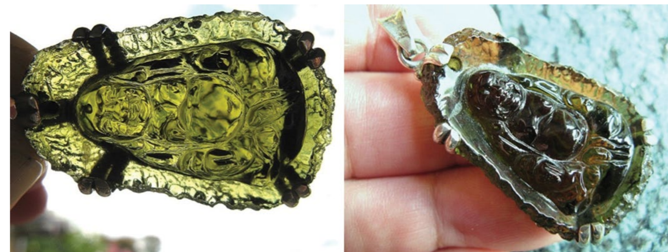
Figure 10. Purportedly a carved Kuan Yin moldavite, actually a mould and sand-cast glass simulant with absence of lechatelierite stringers. Left: in incident daylight. Right: In transmitted daylight.
