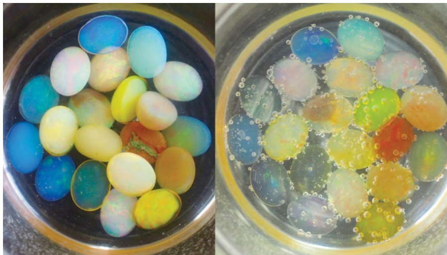
Figure 9. Ethiopian opals immersed in water demonstrating their typical hydrophane nature. The photo on the left is after immersion for one minute and on the right after 60 minutes.
