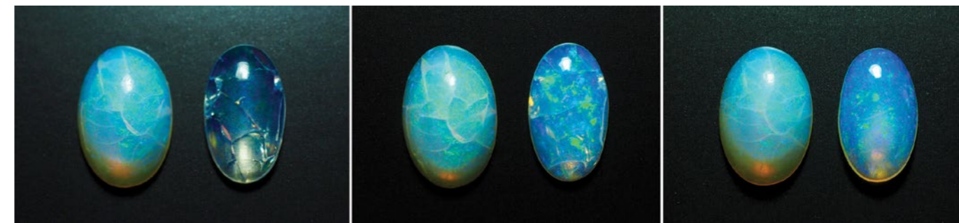
Figure 17. In each image a cracked Australian opal on the left and a cracked Ethiopian hydrophane opal on the right. Left: Fully saturated with water. Centre: Dry. Right: After Opticon treatment. This demonstrates the reduced visibility of cracks, and significant loss of play-of-color in the Ethiopian hydrophane opal.
