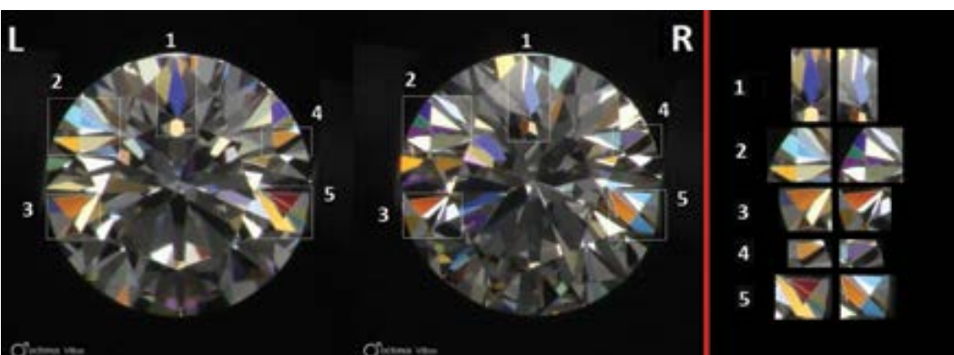
Figure 3.27 Examples of interaction of flashes seen by the left-eye and right-eye of a diamond in the course of forming the resultant image. The numbered frames mark some groups of closely spaced flashes seen by each eye. For convenience, the framed areas are combined in pairs in the right box.
