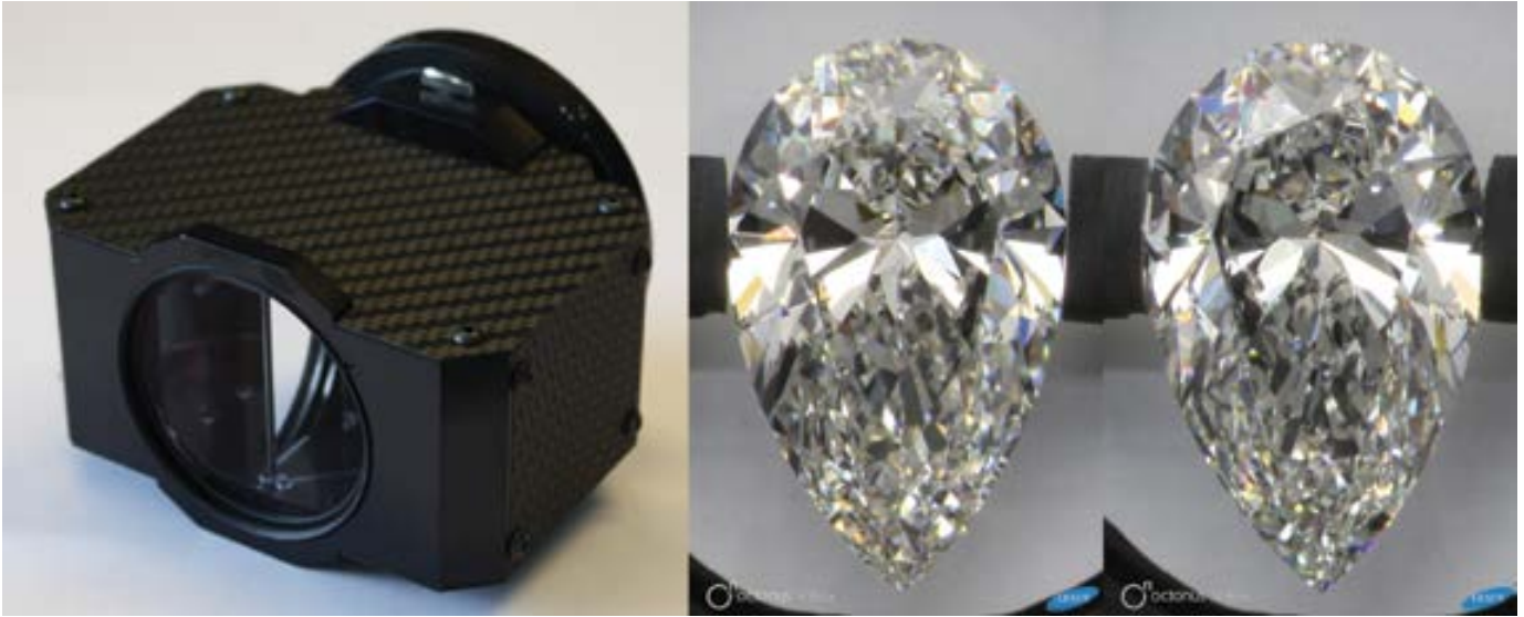
Figure 4.2 On the left is the custom designed stereo splitter that attaches to the end of the macro camera lens. The image on the right side shows a stereo pair of a diamond captured in ViBox with the OctoNus and Lexus watermark logos.
