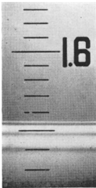
FIG. 3. Anomalous refractive index of a tourmaline showing the basic ray at 1.645 accompanied by 3 satellite shadows, that is, 4 shadows in all. See text.
