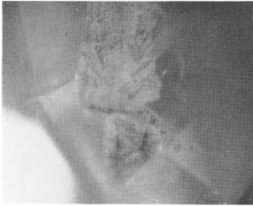
FIG. 7. Peridot—pseudo-hexagonal inclusion and large dendritic feather inclusion 25 × magnification, transmitted light.
