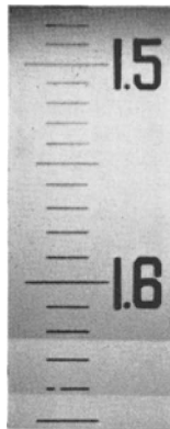
FIG. 1. Typical refractive indices of a normal tourmaline as seen on an Anderson-Payne spinel refractometer, with \omega = 1.642 and \epsilon = 1.623 in sodium light.
