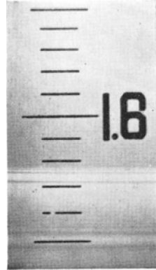
FIG. 3. Anomalous refractive index of a tourmaline showing the basic ray at 1.645 accompanied by 3 satellite shadows, that is, 4 shadows in all. See text.
