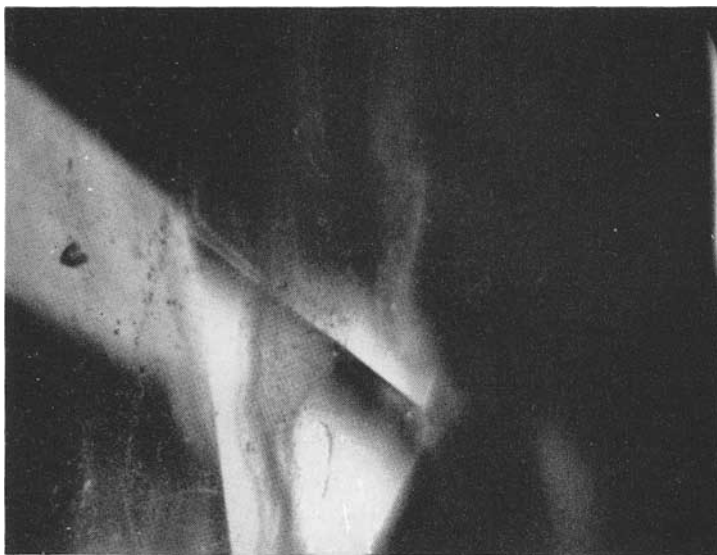
FIG. 2. Obsidian—Coloured bands, tiny crystallites, dust clouds, transmitted light. 30 ×.
