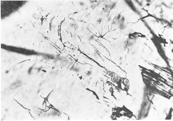
Fig. 5. Highly elucidating picture of the inner world of tourmaline consisting of hair-fine liquid channels (trichites) with two-phase fillings. 20 ×
