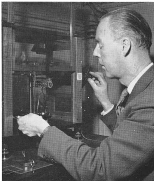
FIG. 4. A. E. Farn weighing stones on an Oertling aperiodic balance. (Photo by courtesy of Gordon McLeish & Associates Ltd.)
