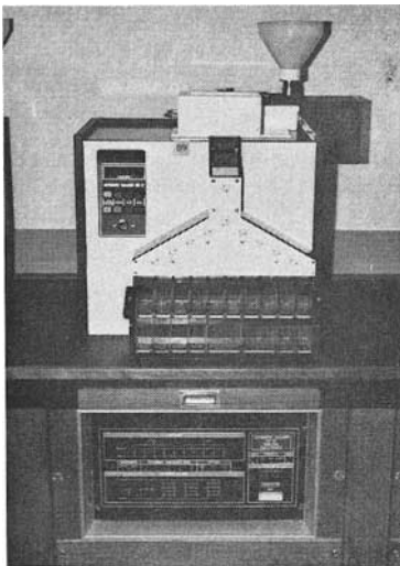
FIG. 7a. Automatic diamond weigher. The top unit contains the weigh head, feeder and sorting mechanisms. The bottom drawer unit contains the control electronics.
