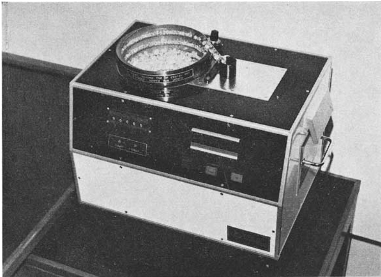
FIG. 6. Counter and batcher for rough diamonds uses a twin infrared light-curtain as detector.
