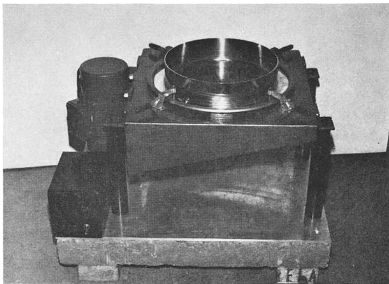
Fig. 2. Motorized sieving machine. Interchangeable ten-inch sieve plates are clamped under a hopper assembly.
