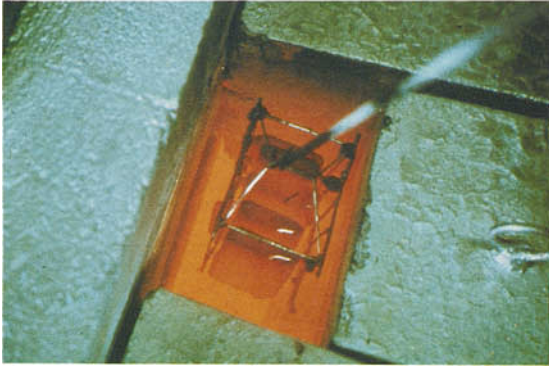
FIG. 5. Gilson synthetic emerald crystals being removed from furnace after nine months' growth.
