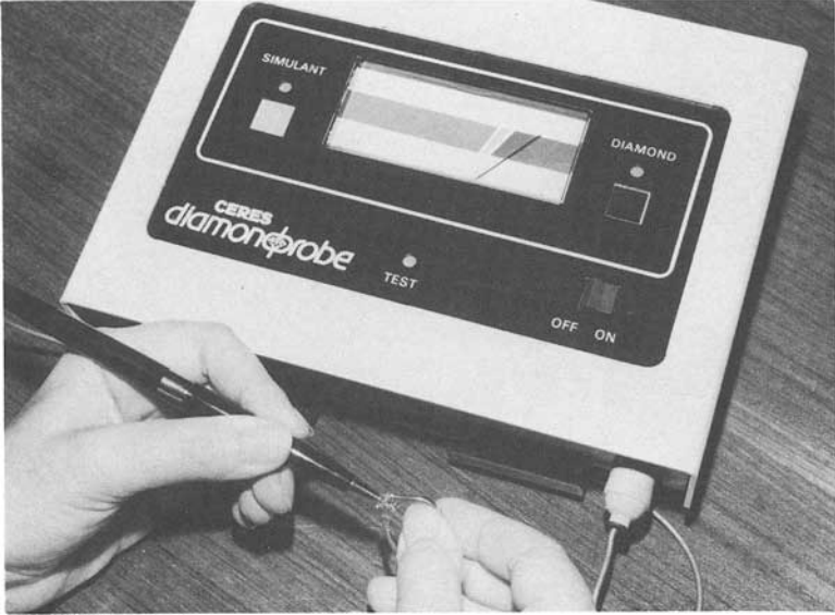
FIG. 6. Testing an 0.75 carat diamond.
