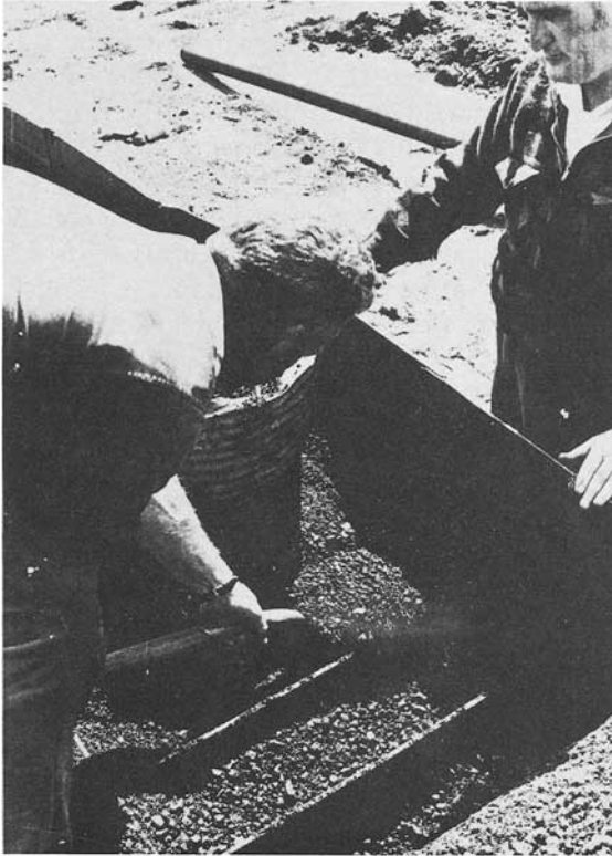
FIG. 8. Cleaning the pulsating jig traps of sapphire-corundum-zircon concentrate on the Reddistone Creek.
