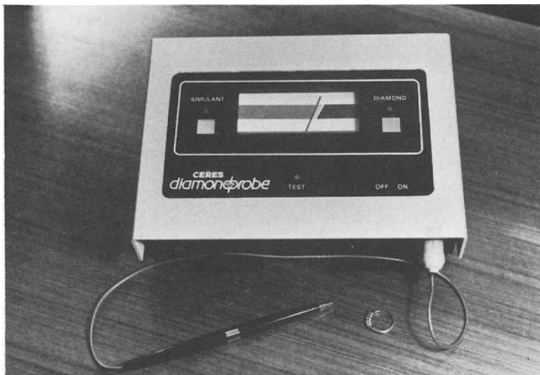
FIG. 4. The Ceres Diamond Probe. On the left of the vertical front panel is the socket for the battery charger and below it the battery warning lamp. (These may be seen better in Fig. 9—but on the right, as the panel is inverted.)
