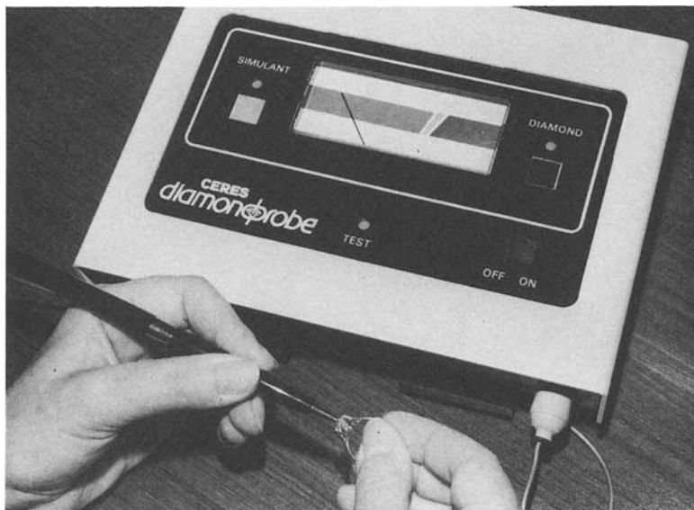
FIG. 8. Testing a 2.5 carat cubic zirconium oxide.
