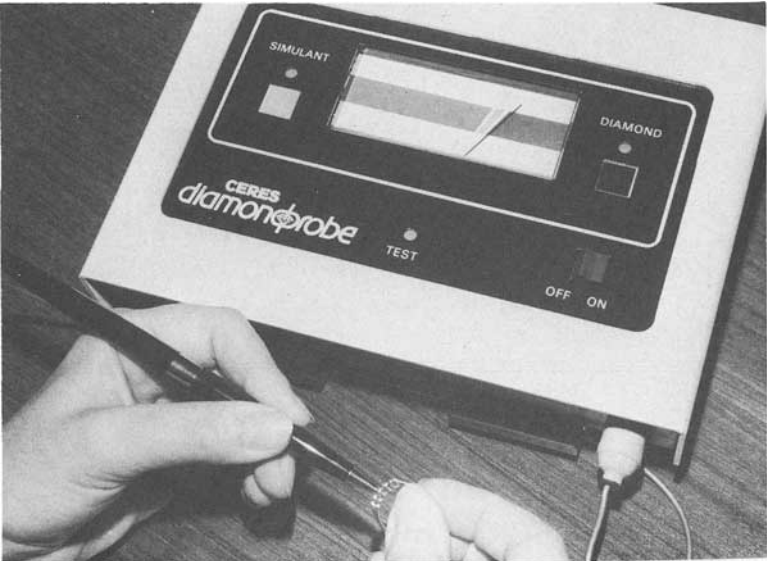
FIG. 7. Testing an 0.03 carat diamond.
