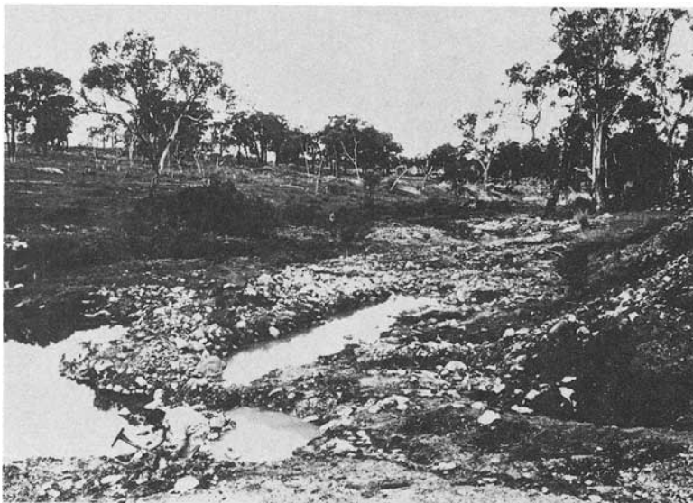
FIG. 5. Gemmiferous alluvium partially excavated along the Fraser Creek. Note the narrow valley fill suitable only for small scale mining operations.
