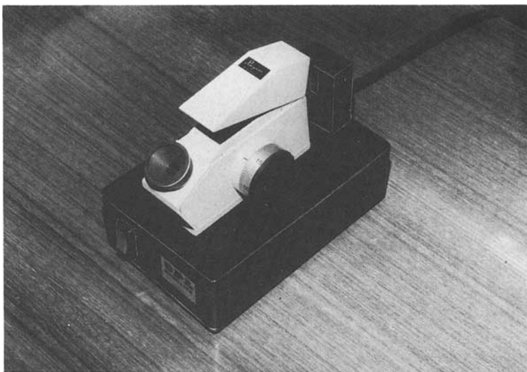
FIG. 1. The 'Monolite' with a Dialdex refractometer.
