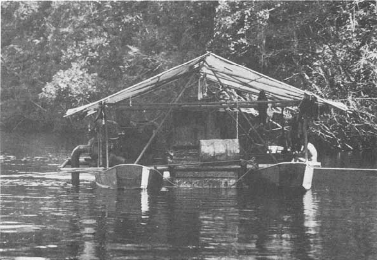
FIG. 9. A pork-knocker's barge on the Mazaruni River. Suction-pump and compressor can be seen on one pontoon, while a diver kits up on the other. The sluice for recovering the gold and diamonds is between the pontoons.
