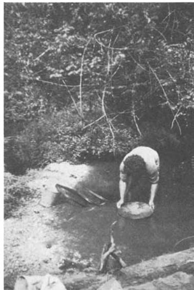
FIG. 4. A pork-knocker prospecting in the 'back-dam'. A set of three sieves is used to recover any diamonds, while the batel which he is holding is used to concentrate the gold.
