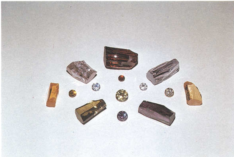
FIG. 1. Seven coloured cubic zirconia crystals (courtesy of Mr J. F. Wenckus, of Ceres Corporation), and seven polished specimens (courtesy of Mr J. F. Turner, of Glenjoy Lapidary Supplies).
