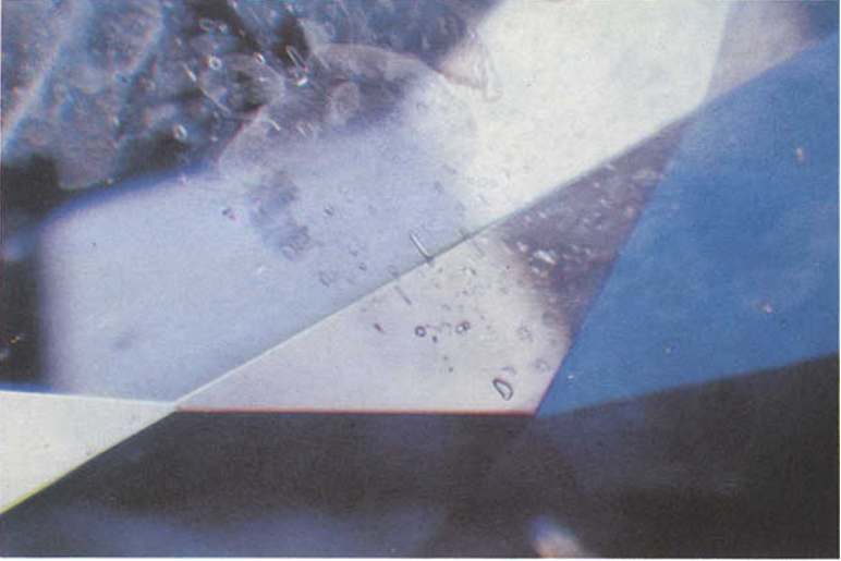
FIG. 5. 'Ceylon feathers' in a blue treated corundum.
