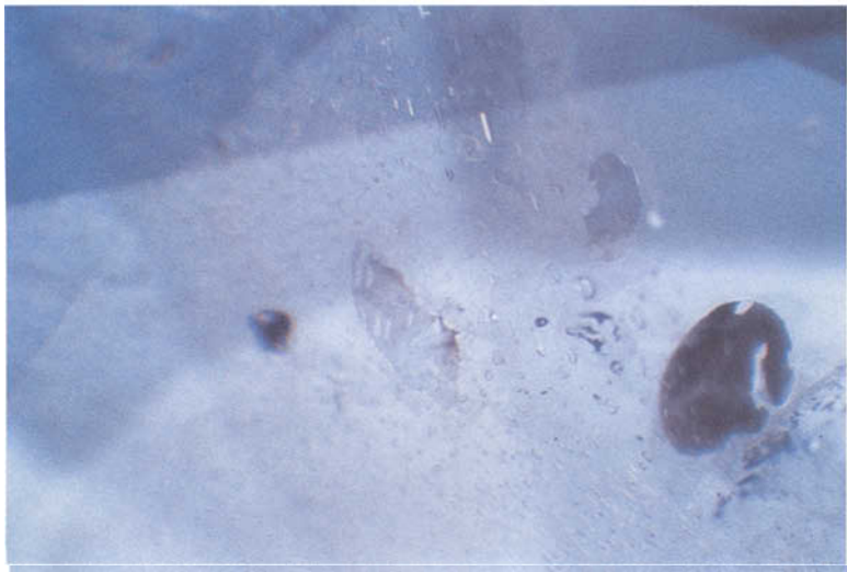
FIG. 7. The 'glassy' or 'watery' centres to Ceylon feathers, which are so characteristic of many heat-treated sapphires, seen here in a treated blue corundum.
