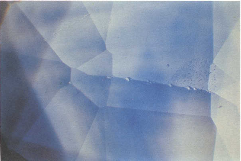
FIG. 6. The patchy colour-zoned appearance of a normal heat-treated blue sapphire.
