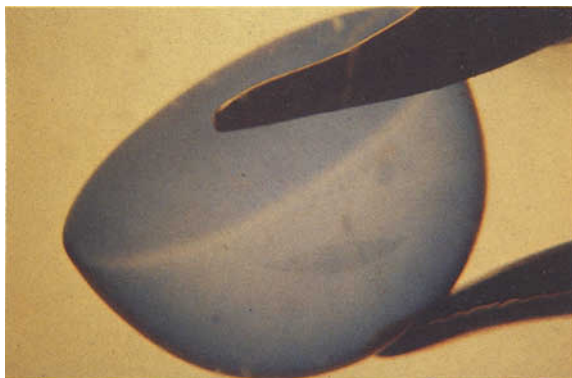
FIG. 9. Colour-diffused cabochon sapphire, with colour removed from an area around the girdle.
