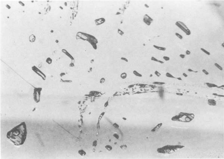
FIG. 6. Two-phase inclusions in sphenite RGM 151 862, \times 25 .
