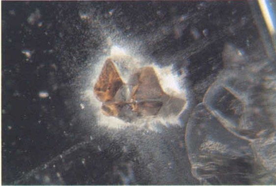
FIG. 11. Group of three large pseudo-hexagonal crystals of phlogopite partly coated by muscovite flakes in close proximity to a large fracture. Greenish-blue aquamarine from Kenya. 35 ×
