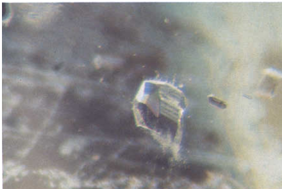
FIG. 3. One well-shaped niobite crystal with metallic lustre and tarnish colours. 50x
