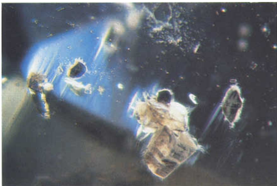
FIG. 4. Survey photomicrograph of part of the internal paragenesis of the second goshenite from Brazil. We recognize large brownish pseudohexagonal crystals of biotite accompanied by numerous black grains of niobite.
