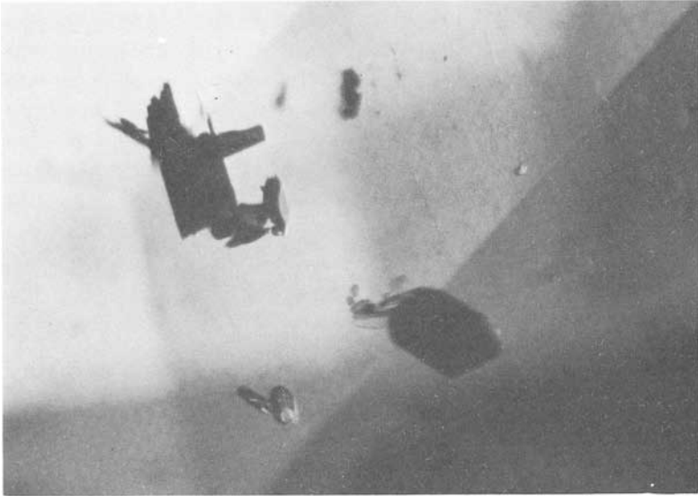
FIG. 5. Crystal inclusions, probably apatite, in sphenite RGM 151 863, \times 25 .
