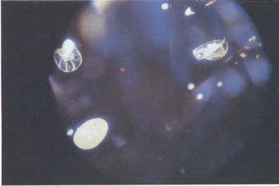
FIG. 2. Internal stress fractures around single-crystal inclusions in heat-treated natural sapphire.
