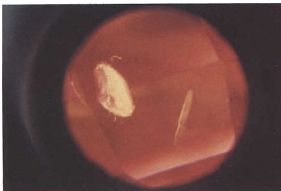
FIG. 16. Induced fingerprint inclusion in Verneuil synthetic pink sapphire.
