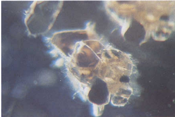
FIG. 2. Detail of Figure 1: cluster of pseudo-hexagonal crystals of phlogopite accompanied by black grains of niobite. 100x
