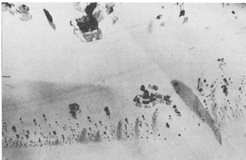
FIG. 4. Liquid inclusions in sphene RGM 151 855, \times 25 . Note the strong doubling of the inclusions.
