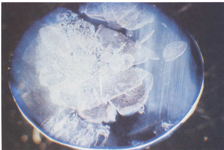
FIG. 9. The colour concentration at the surface of a treated blue corundum, seen here as a royal blue rim following the girdle line.
