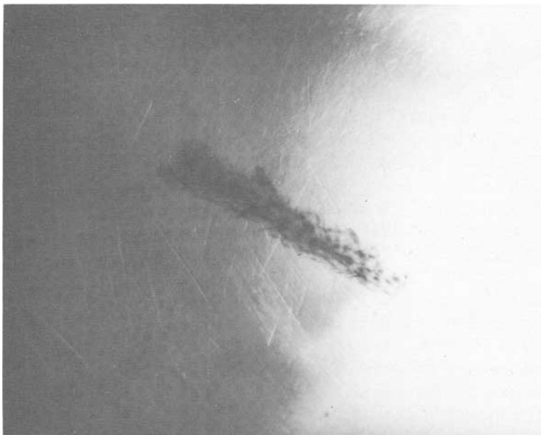
FIG. 3. The mark produced when the surface of the plastic-impregnated synthetic white opal is lightly touched with the tip of the thermal reaction tester.
