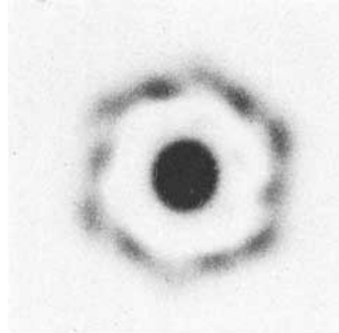
FIG. 10. Lauegram of a natural pearl, drop shape, 21 \times 11 mm, taken through the short axis.
