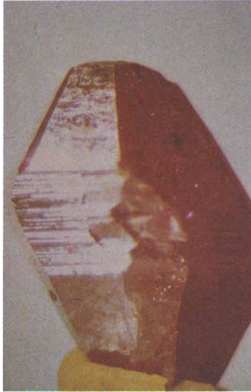
FIG. 1. Single crystal of synthetic ruby made by Knischka showing the pseudo-hexagonal bipyramidal form with horizontal striations.
