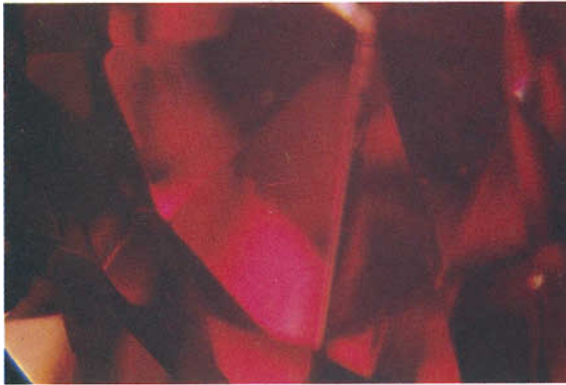
FIG. 32. A minute, almost invisible needle, highly reminiscent of a slender rutile needle, in a synthetic ruby by Kashan. 40 ×
