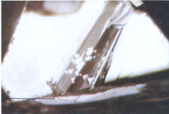
FIG. 8. 'Trigons' on the surface of an octahedral face of a near colourless spinel octahedron.
