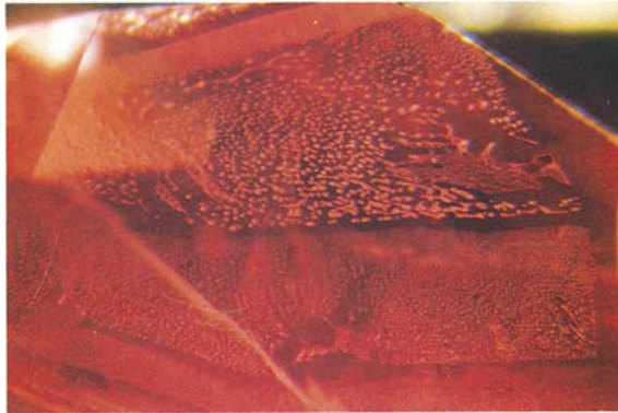
FIG. 15. Broad zones of delusive dactyloptical inclusions in a synthetic ruby by Kashan. 32 ×
