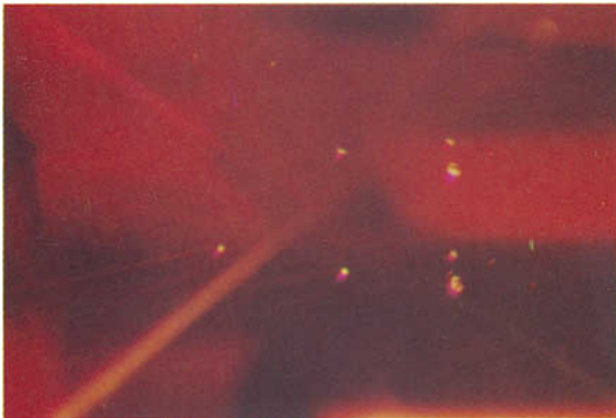
FIG. 31. Several 'comets' consisting of a tiny grain of flux in connexion with divergent tails of ultra-fine flux in a synthetic ruby by Kashan. 50 ×
