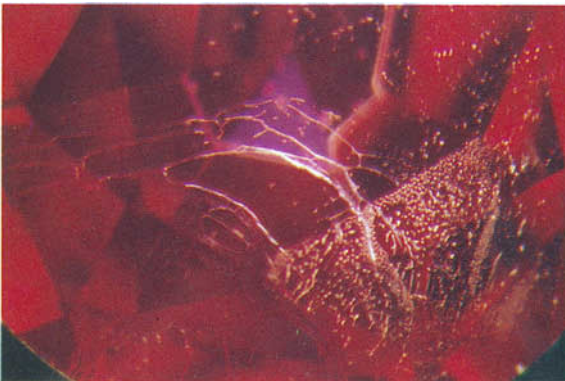
FIG. 22. Misleading inclusion scene which one might expect to find in Thai rubies, yet photographed in a synthetic ruby by Kashan. 30×
