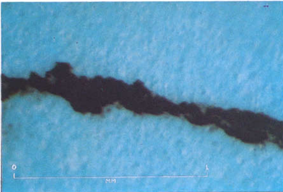
FIG. 2. The surface structure of the 'neolith' imitation turquoise.
