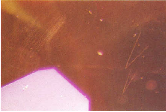
FIG. 35. Two needles meeting at an odd angle simulate one of the rare kneetwins of natural rutile, here accompanied by tell-tale grains of flux in typical arrangement in a synthetic ruby by Kashan. 80 ×
