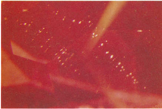
FIG. 12. Parallel bands of minute flux grains (in parallel alignment among themselves) in a synthetic ruby by Kashan. 30 ×
