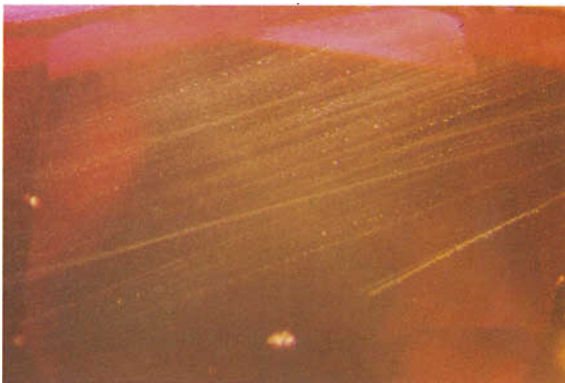
FIG. 28. Narrow, parallel striations of so-called 'fog' in a synthetic ruby by Kashan. 15 ×
