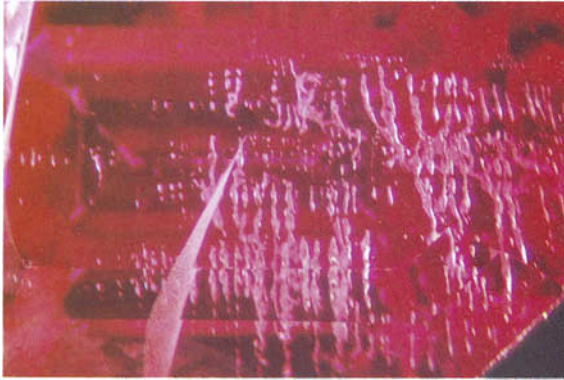
FIG. 8. Profiled 'tubes' of flux inclusions in parallel alignment in a synthetic ruby by Kashan. 30 ×
