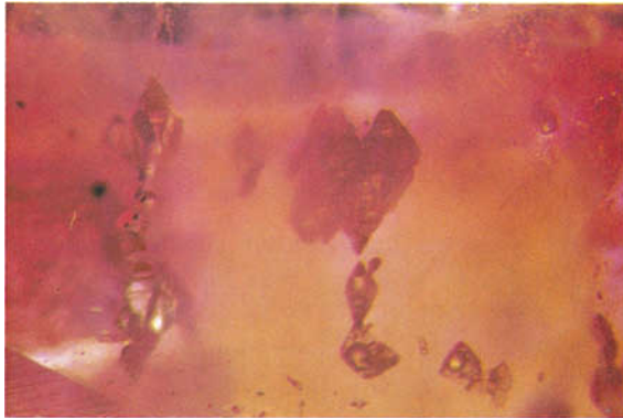
FIG. 40. Small and large negative crystals in parallel orientation and filled with a fluid and a gas bubble in a synthetic ruby by Knischka. 25 ×
