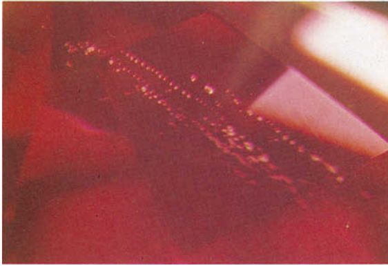
FIG. 11. Parallel rows of small to tiny grains of flux (some with crystalline aspect) in a synthetic ruby by Kashan. 30 ×
