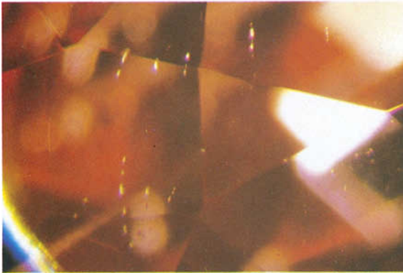
FIG. 24. A V-shaped arrangement and discrete rows of tiny grains of flux in a synthetic ruby by Kashan. 28 ×
