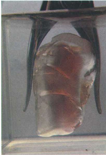
FIG. 6. Heliolite rough with typical colour distribution: a clear border, green (dichroic red-green) band enclosing red (non-dichroic) core—photographed in immersion cell with 35 mm edge. (Photo by author)
