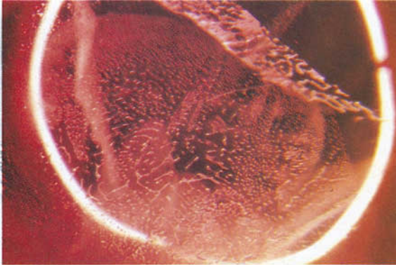
FIG. 5. Deceptive inclusion scenery draped by a large and delicately designed 'fingerprint'-feather and a feather of coarse pattern of flux in a synthetic ruby by Kashan. 25 ×
