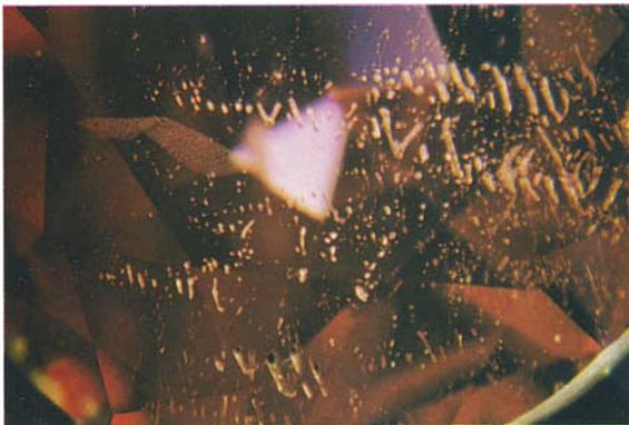
FIG. 25. Flux inclusions simulating archaic characters in a synthetic ruby by Kashan. 30 ×
