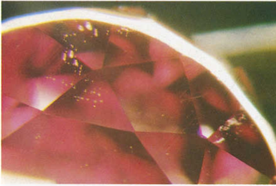
FIG. 26. Tiny flux inclusions looking like crystal shapes accompanied by a double row of minute flux grains in a synthetic ruby by Kashan. 50 ×
