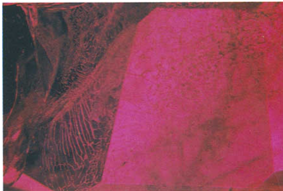
FIG. 16. Tell-tale lace-like inclusions (left in dark-field, right in bright-field illumination) in a synthetic ruby by Chatham. 8 ×
