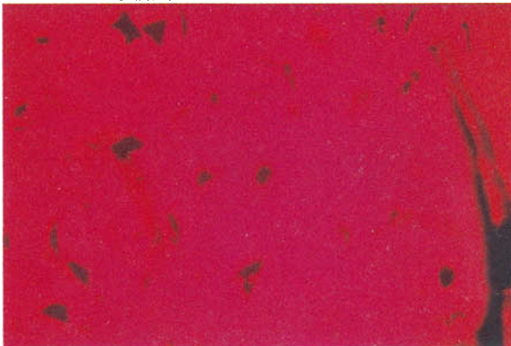
FIG. 6. Platinum platelets in the Knischka synthetic ruby.
