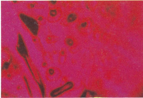
FIG. 7. Peculiar two-phase inclusions in the Knischka synthetic ruby. The high relief of the bubbles contrasts with the hardly visible outlines.
