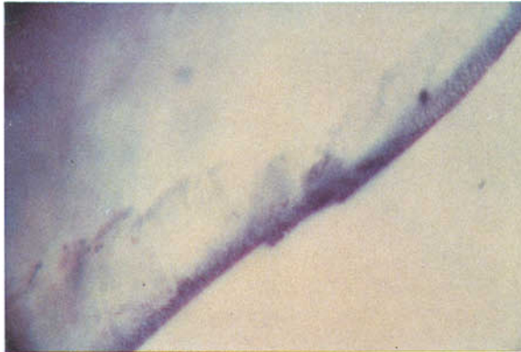
FIG. 5. The blue colour concentration where a feather meets the surface of a cabochon-cut treated blue corundum.
