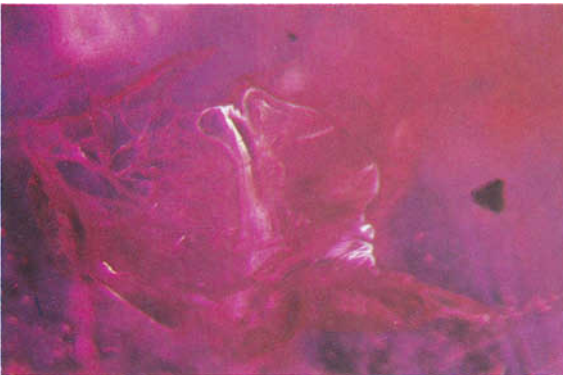
FIG. 7. Large shapeless flux inclusion enveloped by a net-like feather (misleadingly consistent with the rosettes in Thai rubies) in a synthetic ruby by Knischka. 32 ×
