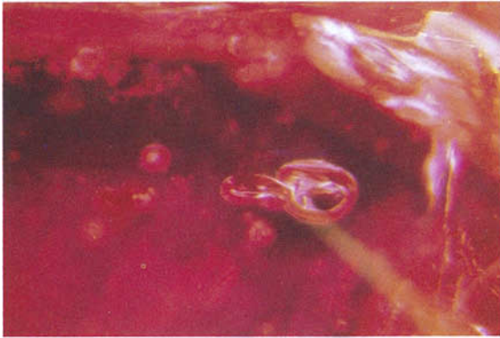
FIG. 41. Two large ellipsoidal two-phase inclusions, which may occasionally extend into long hoses. They always contrast strongly with the enclosing body of the synthetic rubies by Knischka. 50×
