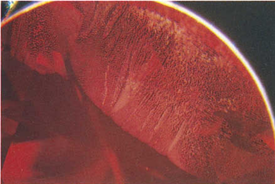
FIG. 19. 'Feathers' with such 'folds' have heretofore been considered as typical hallmarks of Burma rubies. Yet here they were observed in a synthetic ruby by Kasha. 25×
