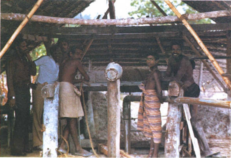
FIG. 4. Vertically sunk pit mining at Meetiyaogoda. (Photo: M. Gunawardene.)
