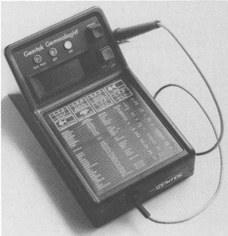
FIG. 1. The Gemtek 'Gemmologist'. Later models have the 'temp' and 'range' pre-sets accessible at the front edge of the control box.
