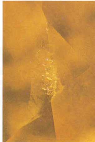
FIG. 10. Healing fissure of drop-shaped and tubular cavities in an annealed yellow corundum; 40 x.
