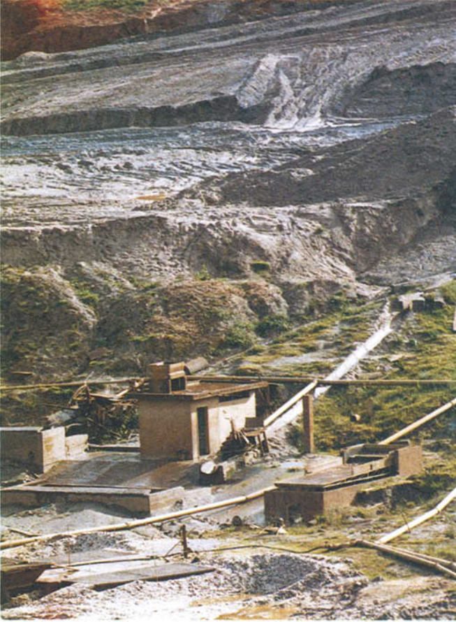
FIG. 1. At the Capao Mine topaz-bearing earth is tumbled down a trough: the topaz is separated by hand.
