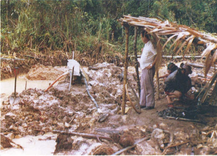
FIG. 10. Andalusite is found in sandy gravel under about two metres of clay. Water seeps back almost as fast as it is pumped out of the pit.
