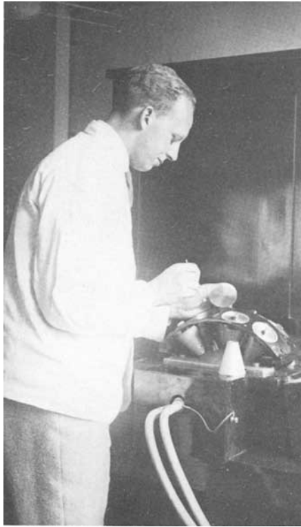
FIG. 1. B. W. Anderson positioning pearls for lauegrams on the 1929 x-ray generating set.
