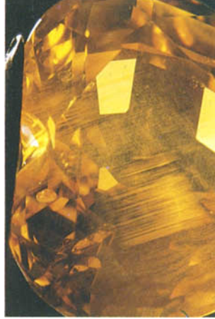
FIG. 11. Fibre-like altered, oriented inclusions and plate-like tension cracks in an annealed yellow corundum; 10 x.
