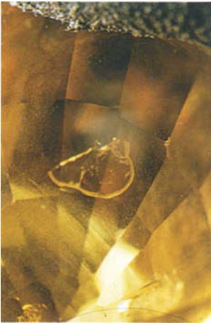
FIG. 8. Clouds of tiny inclusions and reflective, marginally structured tension fissures in an annealed yellow corundum; 40 x.
