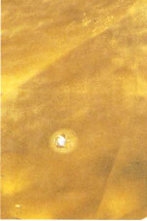
FIG. 9. Plate-like tension fissure resembling an atoll, in an annealed yellow corundum; 30 x.
