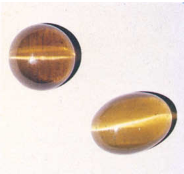
FIG. 1. A, greenish-yellow and a reddish-brown apatite with fine cat's-eye effect, which is produced by scattering of light on goethite fibres. Umba Valley, Tanzania. Long axis of oval cabochon = 15mm.
