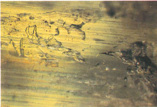
FIG. 18. Photomicrograph of a very irregularly outlined thin film-like partly healed crack in an emerald from the Emerald Mine. ( \times 20 magnification)
