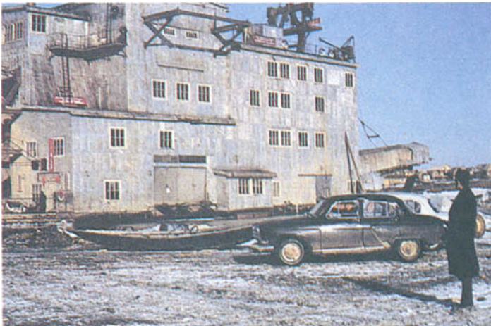
FIG. 8. This huge dredger melts the frozen ice and floats on its own pool; it scoops up the alluvial material, crushes and separates it, and deposits any unwanted material behind it as it moves along.
