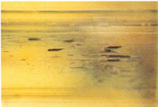
FIG. 11. Photomicrograph of trichite-type inclusions in an emerald from the Emerald Mine. This inclusion has been formed by epigenetic mineral infiltration of resorbed parallel oriented tubular inclusions. ( \times 20 magnification)
