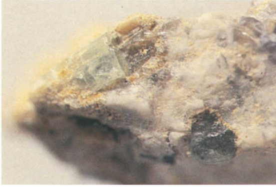
FIG. 3. Emerald crystals in a flattened vugh, in the lode at the Emerald Mine. Note the presence of the minerals that are associated with this lode: fluorite (purplish), dickite (opaque white), arsenopyrite (silvery), quartz (glassy grey).
