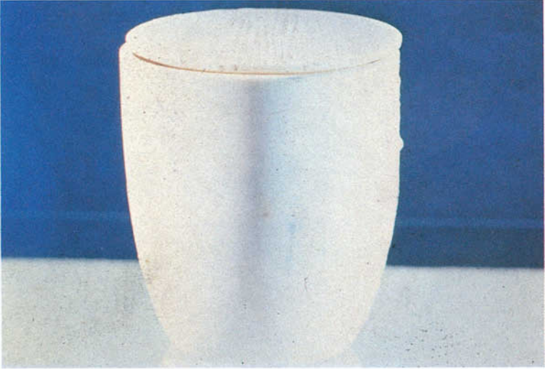
FIG. 1. A crucible extensively used in the heat treatment of ruby.
