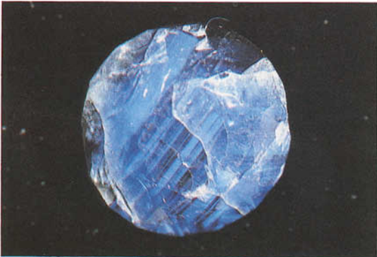
FIG. 5. Brilliant cut (8.5 mm dia × 4.5 mm) 2.7 ct dark blue stone with pronounced colour zoning and many fractures.
