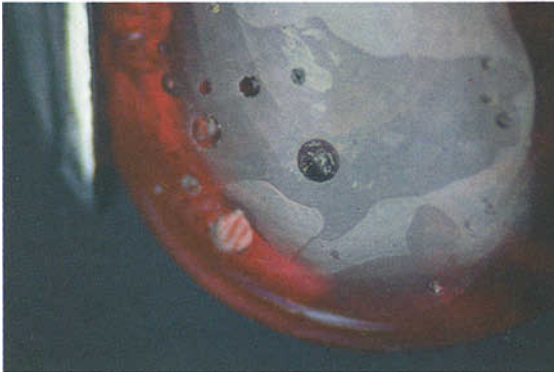
FIG. 3. Repaired areas (with shaded appearance) in Thai ruby visible under oblique illumination. Note suspended gas bubble inside repaired area. 38 ×.
