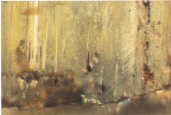
FIG. 10. Photomicrograph of a two-phase primary 'dagger' inclusion included in an emerald from the Emerald Mine. This inclusion has been initiated by an included cassiterite crystal. The 'dagger' is oriented parallel to the c -axis. ( \times 20 magnification)
