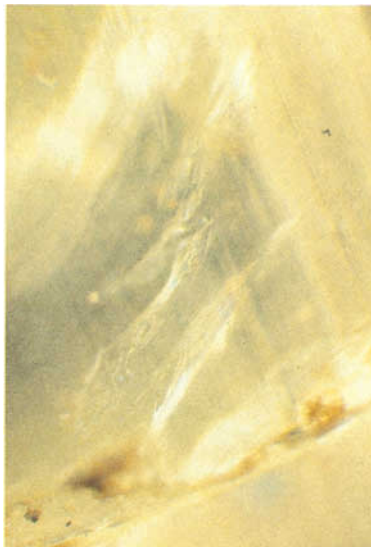
FIG. 16. Photomicrograph of randomly oriented partly healed cracks in an emerald from the Emerald Mine. Note the angulation of these cracks to the basal plane of the crystal. ( \times 20 magnification)
