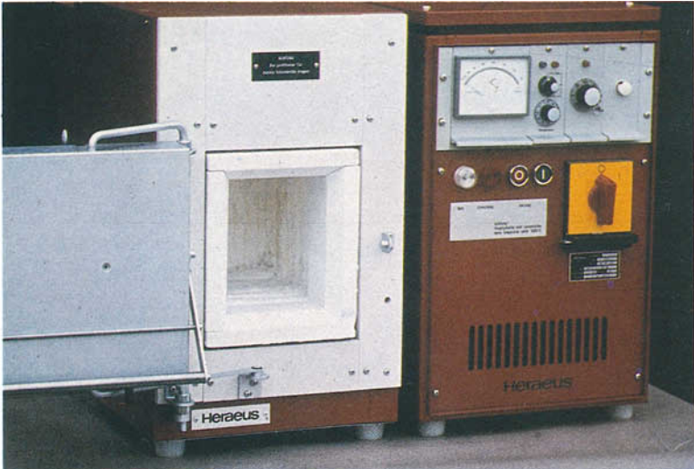
FIG. 2. High temperature chamber furnace manufactured by Heraeus in West Germany. Owing to rapid heating system it is used in the heat treatment of corundum (after Heraeus, model number K 1700/1).
