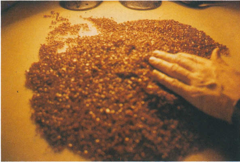
FIG. 3. Sorted rough ruby lot weighing 3000 grams just after heat treatment.
