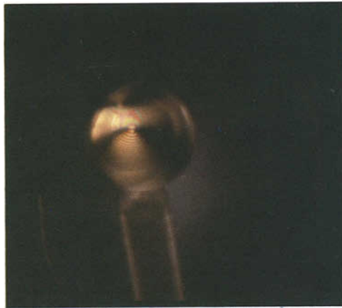
FIG. 1. Biaxial interference figure made visible by a glass sphere between crossed polars.
