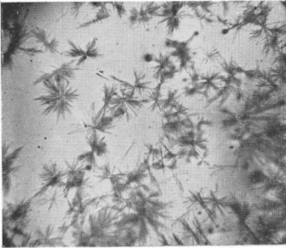
Fig. 3 – Calcium Sulphate Crystal resulting from microchemical test (approx. x 50).
