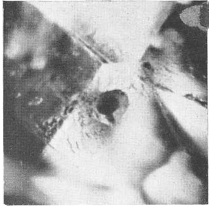
FIG. 10. Opaque corundum crystal sur- rounded by a liquid feather in a Siam Ruby.
