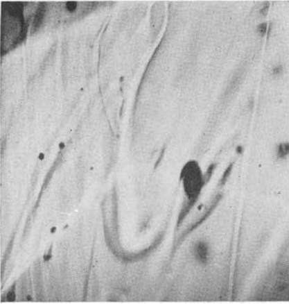
FIG. 44. Swirl marks and gas bubbles in a Moldavite. 30 ×
