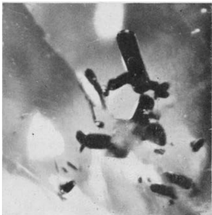
FIG. 2. Well developed crystals of Rutile in a Burma Ruby. 75 x
