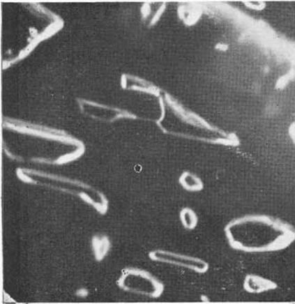
FIG. 35. Same cavities after Aquamarine was heated above 31.5°C. All liquid carbon dioxide has evaporated (no bubbles visible). 50 x
