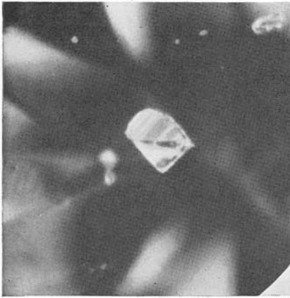
FIG. 27. A distorted diamond octahe- dron in a Diamond. 100 ×
