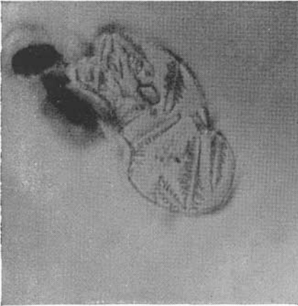
FIG. 43. Recrystallisation in the liquid inclusion of a Siam Sapphire. 125 x
