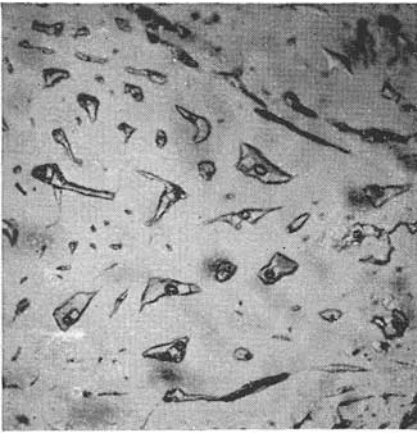
FIG. 41. Three-phase inclusions in a Colombian Emerald. 40 x
