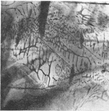
FIG. 58. Scriptine-like design of a feather in a Siam Ruby. 50 x
