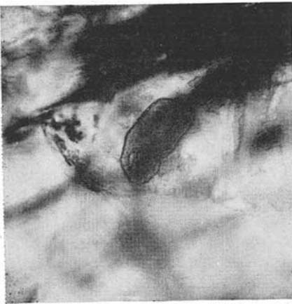
FIG. 7. A xenomorphous flake of mica in a Siberian Emerald. 50 x
