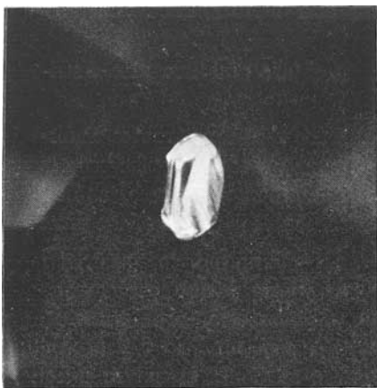
FIG. 13. A zircon crystal embedded in a Diamond. 100 x
