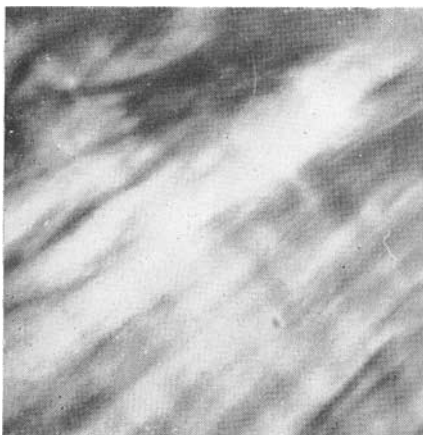
FIG. 78. Anomalous extinction of synthetic Spinel. 10 ×
