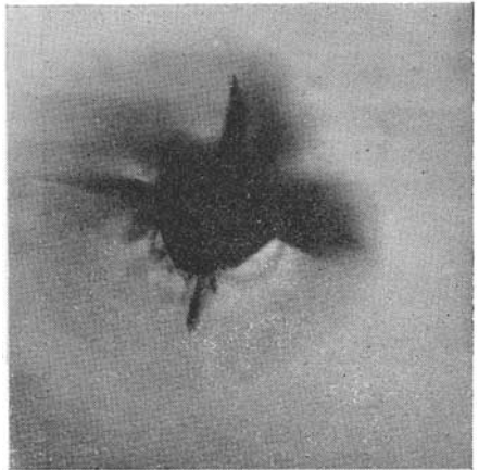
FIG. 29. Radio-active zircon sur- rounded by a radio-halo in a Ceylon Sapphire. 50 ×
