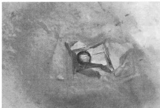
Fig. 3. Two-phase fluid inclusion containing the once-radioactive liquid that caused the brown smoky quartz halo. 5x.
