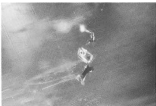
Fig. 7. After a few seconds, the heat from the 30W light bulb of the microscope makes the bubble shown in Figure 6 move slowly to the other end of the negative crystal. 125x.
