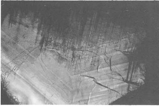
Fig. 4. Topaz from Nigeria irradiated with high-energy electrons; irregular bluish-violet coloration developed at one side of the rim of the sample, intermediate zone with high defect concentration; growth planes are parallel to the prism faces m (110). View parallel to the c -axis; polarized light with E parallel to Y . 20x.
