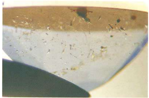
Fig. 11. The crown of the composite stone in Figure 10 is relatively free of inclusions whereas the pavilion, as seen here, contains innumerable two-phase inclusions. The edge of the junction can be seen as a curved red line at the top of the figure, and the pinkish coloration below this is in the plane of the junction. The stone is photographed immersed in benzyl benzoate.
