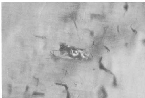
Figs. 5 (a) and (b). Long, two-phase inclusions, one of the most characteristic features, seen under high magnification (125x), (a) in transmitted light, and (b) with dark-field illumination.
