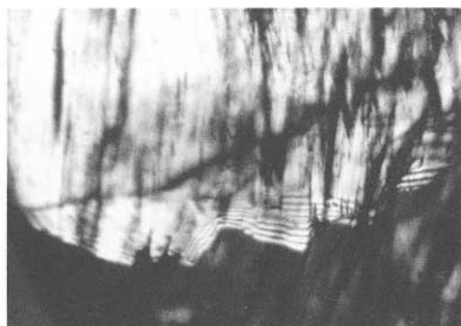
Fig. 3. Sapphire cat's-eye from Burma; interference striations and interference colours are observable at the irregular boundary between the two parts of the crystal. Crossed polarizers. 20x.
