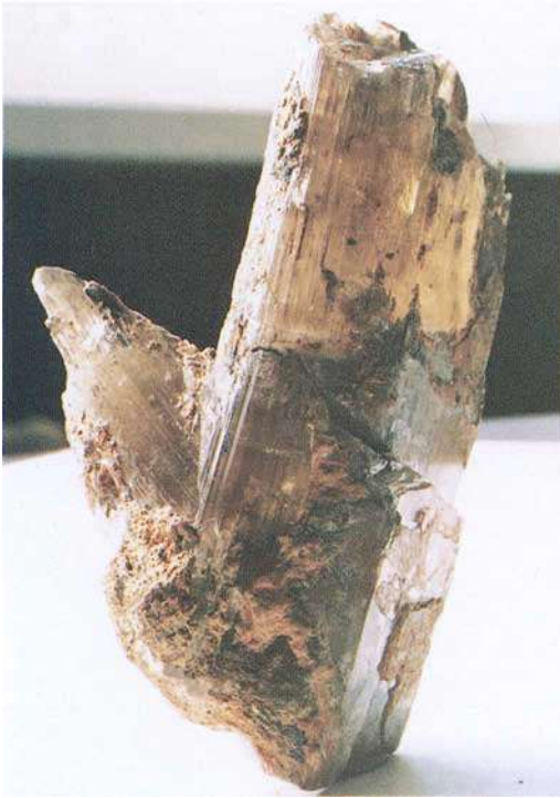
Fig. 1. Diaspore crystal showing twinning. Approximate measurements of crystal: height 68.40 mm, width 32.20 × 27.00 mm, weight 92.34 g.
