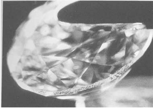
Fig. 1. Fine cleavage fissures running across the slightly polished girdle of a brilliant-cut diamond. Darkfield illumination. 11x.
