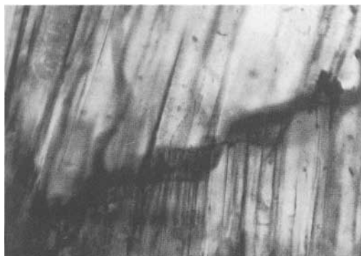
Fig. 2. Sapphire cat's-eye from Burma; the two parts of the stone, which are separated by an irregular surface, reveal glide planes parallel to (0001). The glide planes are inclined against each other forming angles of \approx 169^\circ . 50x.
