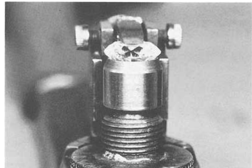
Fig. 4. Brilliant-cut diamond of 2 ct tightly mounted in the dop. Heat accumulation in the finger-like piece of metal sometimes leads to burn marks on the table.
