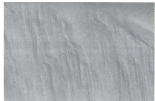
Fig. 21. 'Water in whisky' appearance seen in the Russian synthetic emerald polished rough specimen of Figure 15.
