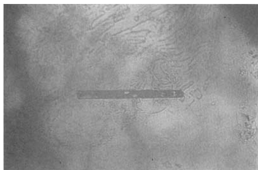
Fig. 26. Blue sapphire from Nigeria, view \perp to the c -axis; prismatic to rounded albite crystals with rosette-like fluid inclusions parallel to the basal pinacoid c (0001). 75x.
