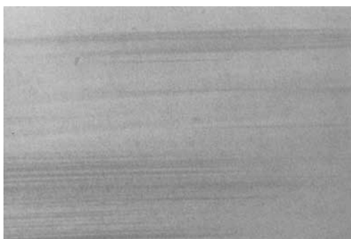
Fig. 18. Blue sapphire from Nigeria, view \perp to the c -axis; growth structure parallel to the basal pinacoid c ( 0001 ), connected with areas of different concentrations of extremely fine mineral inclusions. 45x.
