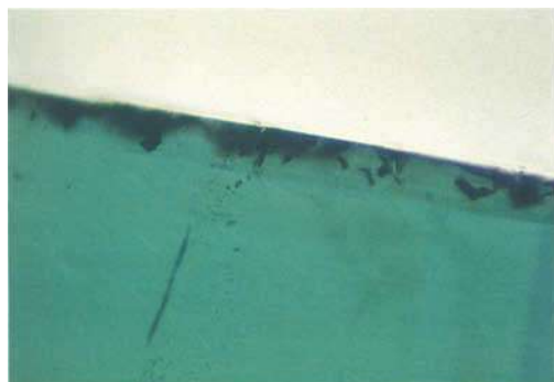
Fig. 25. The platelets seen in Figure 24 are in a layer near the surface which is not of great depth. The layer is seen here in side view.
