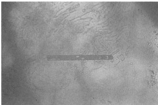
Fig. 28. Blue sapphire from Nigeria; elongated negative crystal with two-phase inclusion, healing fissure. 100x.
