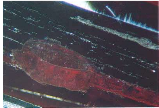
Fig. 34. A closer view of the infilled cavity seen in Figure 33.
