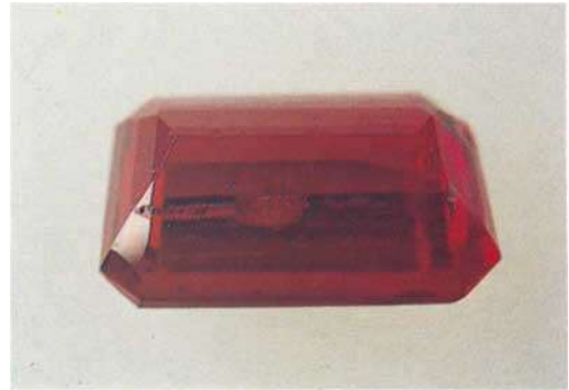
Fig. 33. An infilled cavity in the synthetic ruby of Figure 32 seen here from the bottom of the stone.
