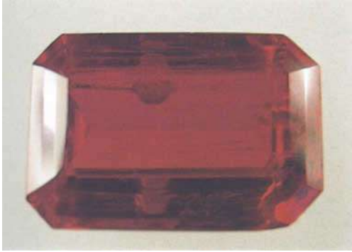
Fig. 32. A 17.81 ct synthetic ruby with infilled cavities. The cavities are seen here looking through the crown to the bottom of the stone, positioned at the lower right corner and at the top edge of the table.
