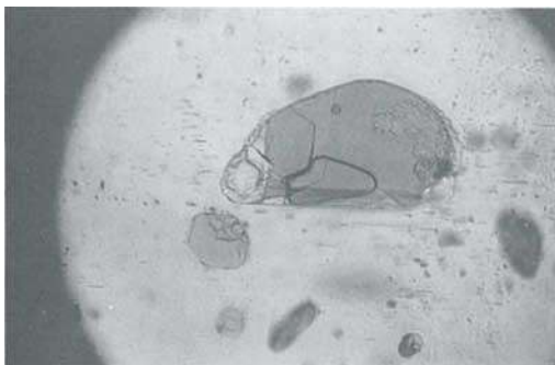
Fig. 9. Mica flake exhibiting solution and recrystallization phenomena. 100x.
