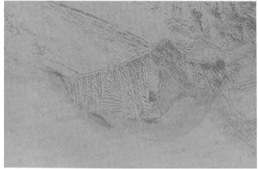
Fig. 31. Blue sapphire from Nigeria; heating fissure. 40x.
