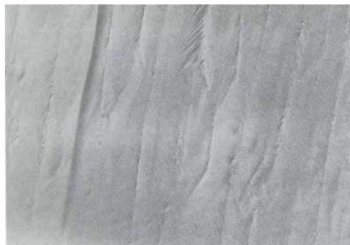
Fig. 22. 'Arrow-head' and 'quill' structures seen in the Russian synthetic emerald polished rough specimen of Figure 15.
