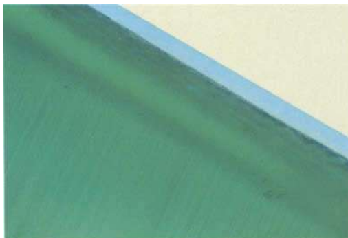
Fig. 26. Colourless seed plate at the surface of the Russian synthetic emerald polished rough specimen of Figure 15.
