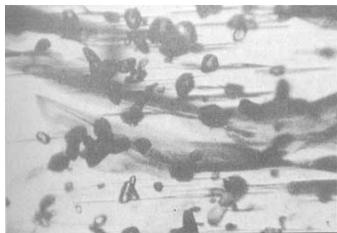
Fig. 25. Blue sapphire from Nigeria; prismatic to rounded albite crystals with rosette-like fluid inclusions parallel to the basal pinacoid c (0001). 65x.
