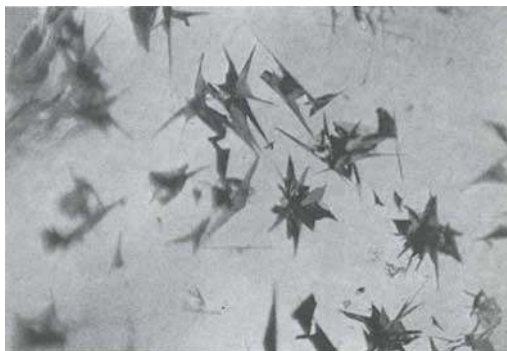
Fig. 24. Reddish/brownish platelets seen at one end of the Russian synthetic emerald polished rough specimen of Figure 15 (see also Figure 16).
