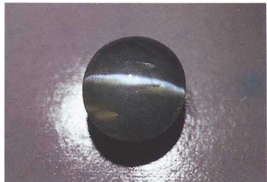
Fig. 2. Heat-treated zircon exhibiting a chatoyancy effect. Most of the stones investigated in this study are of this type. Weight 5.52 ct.
