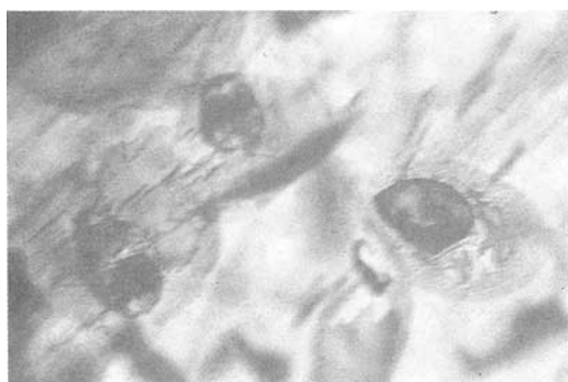
Fig. 14. Lechleitner synthetic ruby; natural seed with platy mineral inclusions (most probably mica) surrounded by liquid feathers. 85x.
