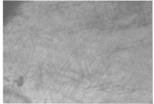
Fig. 2. Asteriated red spinel from Sri Lanka; various sets of parallel orientated needle-like inclusions, most probably rutile. 75x.
