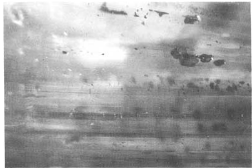
Fig. 4. The growth tubes seen in 'natural' zircon cat's-eye from Sri Lanka are often filled with minute mineral matter. Dark-field illumination. 55 x.
