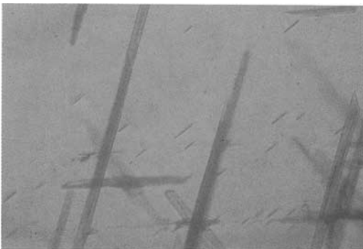
Fig. 5. Bluish-violet spinel from Sri Lanka; view in a direction parallel to one of the three-fold axes \langle 111 \rangle ; cross-sections of one set of lath-like crystals the axes of which are orientated parallel to the direction of view; three sets of parallel inclusions are observable parallel to the remaining three-fold axes \langle 111 \rangle . 75x.
