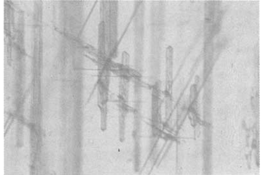
Fig. 4. Bluish-violet spinel from Sri Lanka containing four sets of parallel orientated lath-like inclusions, most probably sillimanite. 70x.
