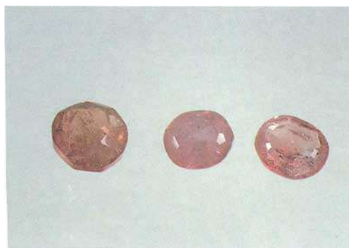
Fig. 1. Lechleitner synthetic rubies with natural seed and synthetic overgrowth. Size of the samples approx. 6 mm. (Photo by O. Medenbach, Bochum, West Germany.)
