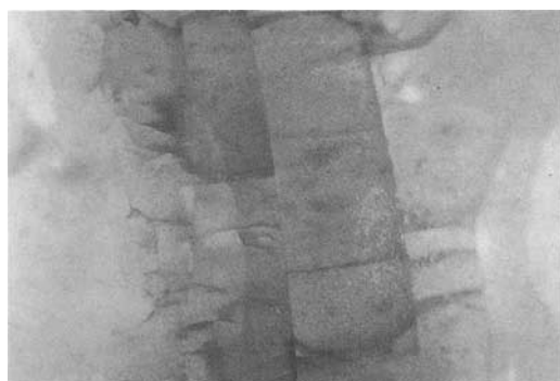
Fig. 7. Visible fire cracks often seen on unpolished surfaces of heat-treated zircons from Sri Lanka. Transmitted light illumination. 53 x.
