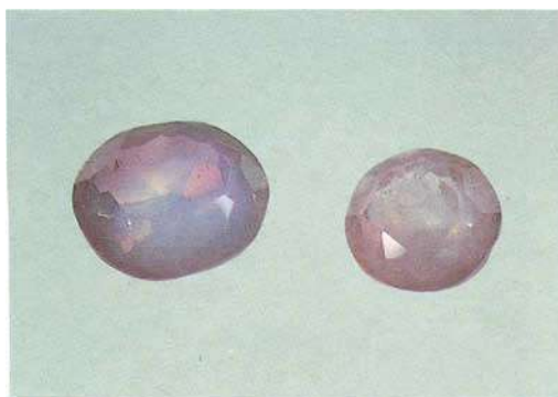
Fig. 2. Colour zoning in Lechleitner synthetic rubies with natural seed and synthetic overgrowth; in one sample the 'silk' of the natural seed is visible. - Size of the samples 8 x 9 and 7 x 7 mm. (Photo by O. Medenbach, Bochum, West Germany.)
