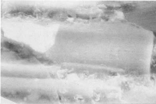
Fig. 6. Long euhedral prismatic crystal of zircon. SEM photograph. 3000x.
