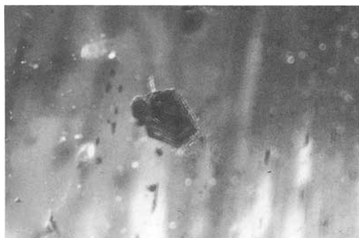
Fig. 5. The enclosed minerals within the tubes were identified as biotite mica in zircon cat's-eye of untreated origin. Dark-field illumination. 80 x.
