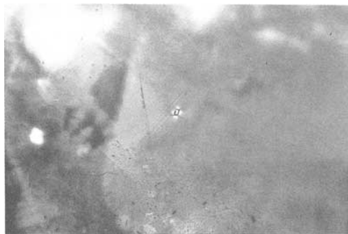
Fig. 13. Lechleitner synthetic ruby; natural seed with rounded doubly refracting mineral inclusion (centre); doubly refracting crystals (most probably corundum) confined to the contact zone between natural seed and synthetic overgrowth (left). Crossed polars, 35x.
