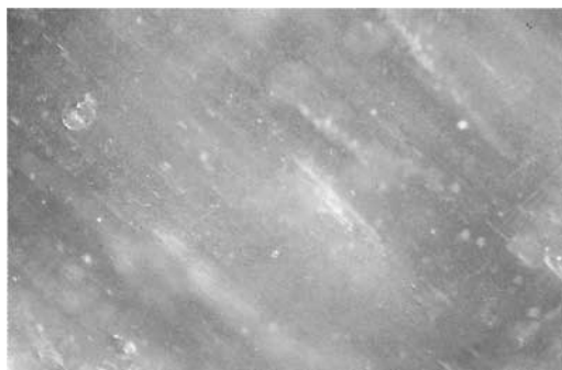
Fig. 1. Numerous transparent crystal inclusions and bunches of narrow channels, cause an evanescent cat's-eye effect. 10x.
