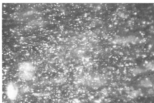
Fig. 6. Fine disc-like tension fissures arranged in parallel orientation in heat-treated zircon cat's-eyes are now available in the trade. Dark-field illumination. 60 x.
