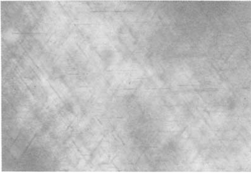
Fig. 1. Asteriated red spinel from Sri Lanka; view in a direction parallel to one of the three-fold axes \langle 111 \rangle ; the axes of three sets of needle-like inclusions, most probably rutile, are orientated parallel to one octahedron face \langle 111 \rangle at 120^\circ intervals. 75x.
