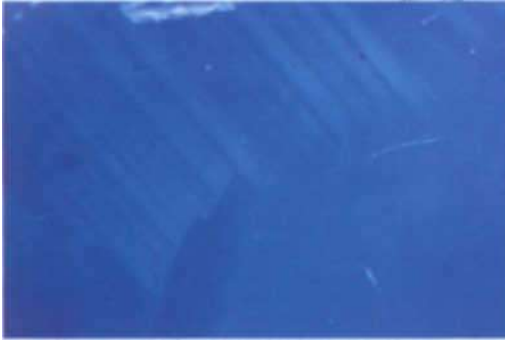
Fig. 3. Turbidity induced by dust particles (rutile?) occurring in zonal lamellae and as fine dust tracks or traces. 30X.
