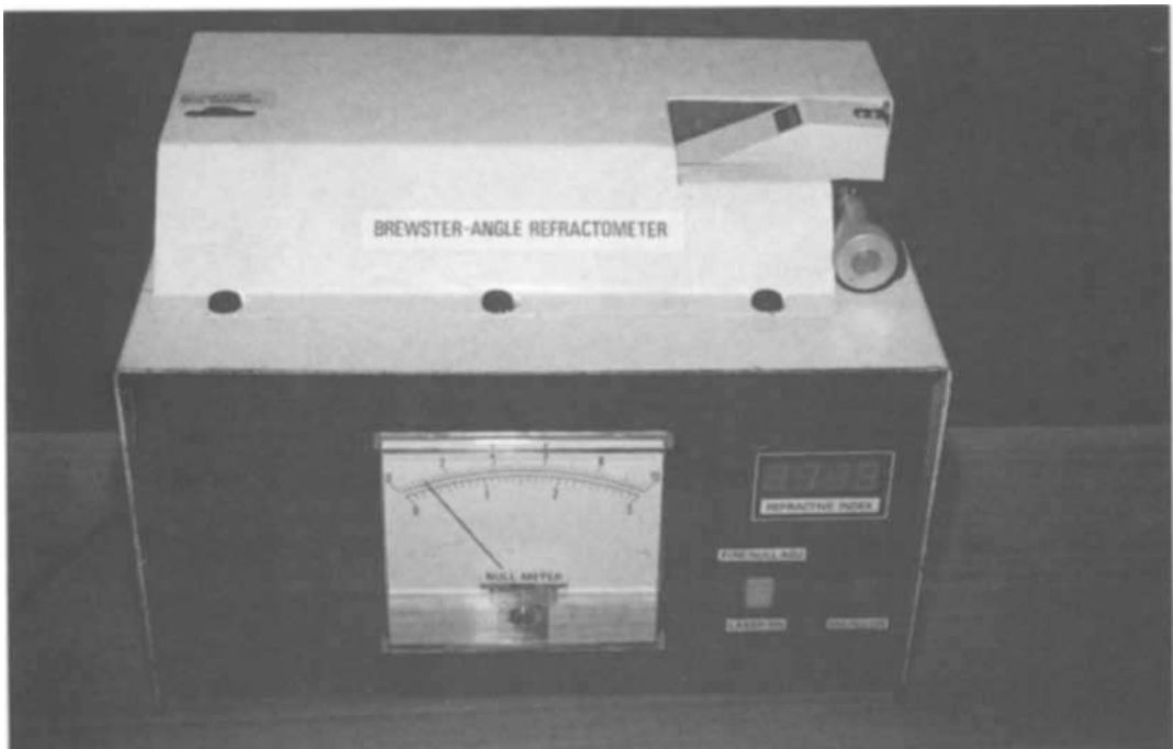
Fig. 7. The latest version of a Brewster-angle refractometer developed by the author. The instrument uses a small polarized laser. The reflected ray from the gem under test is displayed on the null meter in the centre; the laser beam angle is adjusted (by means of the knurled edge control at the top left) for a minimum reading, and the resultant RI reading is displayed on the LED panel meter on the right.
