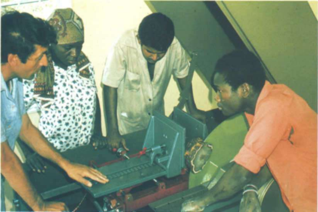
Fig. 7. Teaching seminar at the lapidary workshop in Georgetown showing the cutting of banded agate with a diamond saw.
