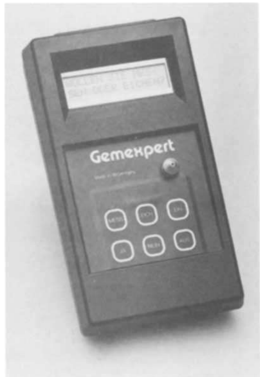
Fig. 4. The GfD Gemexpert contained a microprocessor which enabled it to display the name of the gem under test on its LCD panel.
