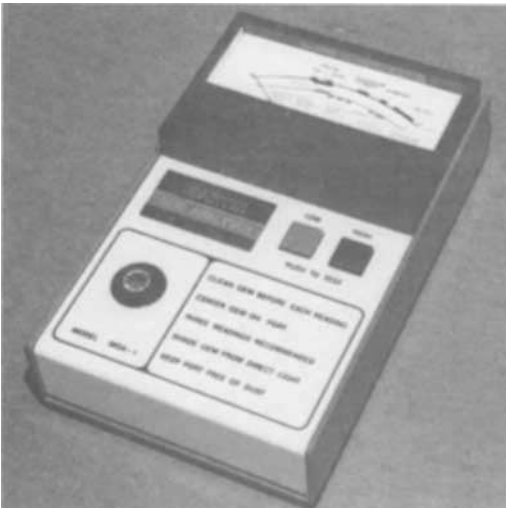
Fig. 2. The Martin Gem Analyser was the first reflectivity meter to use pulsed infra-red illumination which minimized the effect of ambient light entering through the rear of the stone under test.
