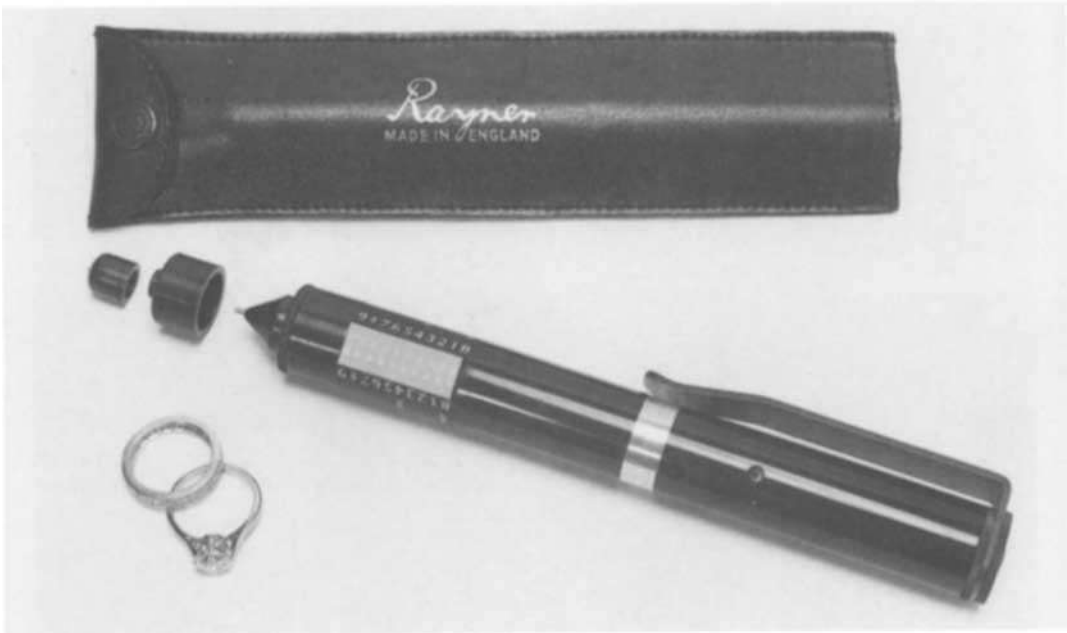
Fig. 5. The Rayner DiamondScan used fibre optics to produce an 0.75mm diameter infra-red beam at normal to the test surface. For large stones it could be fitted with an end cap which provided a flat reference face.
