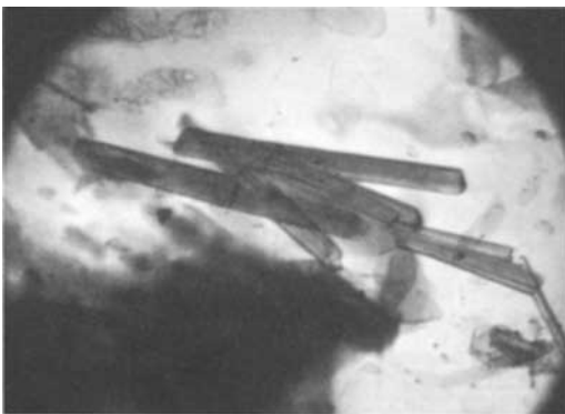
Fig. 12. Dark-brown, prismatic crystals of allanite (orthite). 50x
