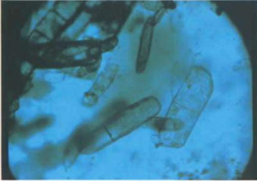
Fig. 13. Apatite in the form of prismatic crystals showing corrosion phenomena and cleavage planes parallel to the basal face. 70x
