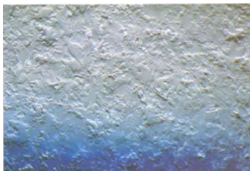
Fig. 2. Undercutting on the largest table cut stone. All four gems showed similar polished-surface undercutting, indicating slight variation in granular hardness and therefore suggesting an impure aggregate nature. Shadowed oblique illumination. 50X.
