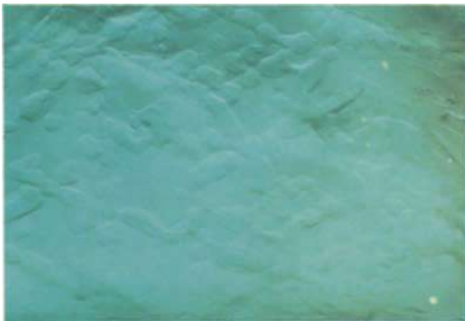
Fig. 21. Axial view onto a basal plane covered with corrosion cells. Shallow etch pits structured with modified or hinted hexagonal contours. Width of photomicrograph about 9 mm.
