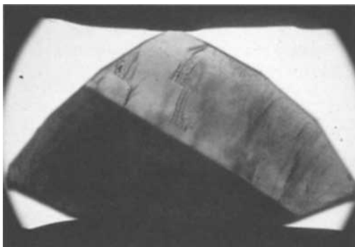
Fig. 44. Growth structures in Pool hydrothermally-grown synthetic emerald; dominant growth line and colour zoning. View 24^\circ inclined to the c -axis. 22x.
