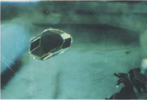
Fig. 11. Distorted polyhedral pyrite crystal with fine tension fissures along its edges, enclosed in a structurally disturbed emerald. Length of pyrite crystal approximately 0.85 mm.
