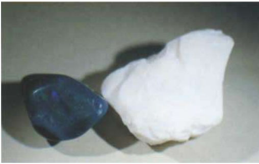
Fig. 8 Highly porous Brazilian opal before (rough) and after being dyed and plastic impregnated.
