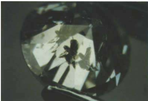
Fig. 18. Black-lined surface reaching fractures in a diamond (as seen from the pavilion) before being treated by the 'oscillating technique'.
