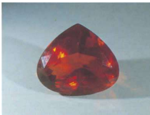
Fig. 3. The pear-shaped fire opal in Figs. 1 and 2 after soaking in water for four weeks. The opaque cone has disappeared leaving only a small turbid area.
