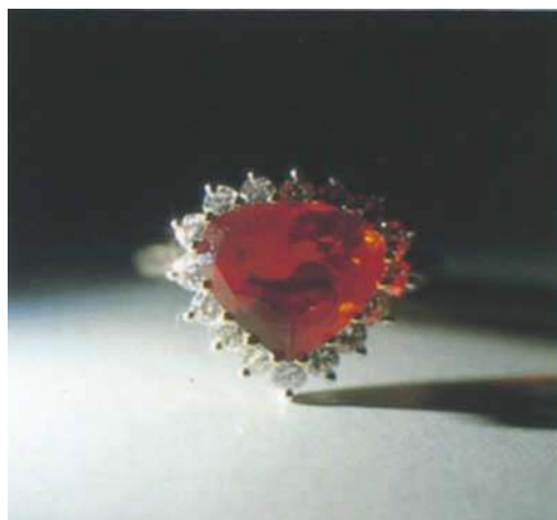
Fig. 1. Pear-shaped fire opal set in a cluster ring. Note the opaque cone at the top right and under the table facet.
