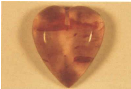
Fig. 2. The interference colours exhibited by the cabochon seen in Fig. 1, when examined through a polariscope.
