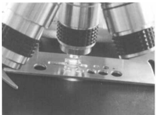
Fig. 4. Unmounted stone, culet down, in slot.
