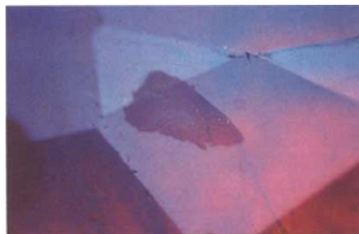
Fig. 5. The larger filled surface cavity in a ruby.
