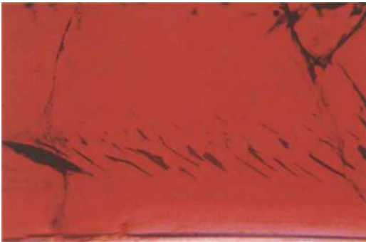
Fig.7. Flux residues in a synthetic ruby from Russia. x15.
