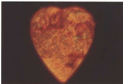
Fig. 2. The interference colours exhibited by the cabochon seen in Fig. 1, when examined through a polariscope.
