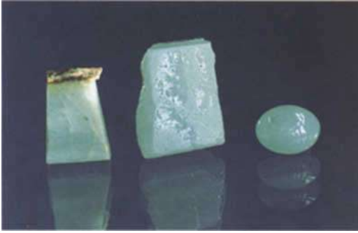
Fig. 1. From left to right: (a) untreated green and white jadeite with a brown iron-stained skin; (b) jadeite which has been bleached and polymer-resin treated; (c) a cabochon fashioned from the polymer-impregnated material.
