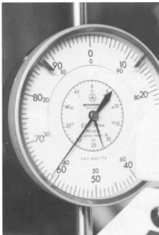
Fig. 1. Dial test indicator 0.50mm, X0.01mm.
