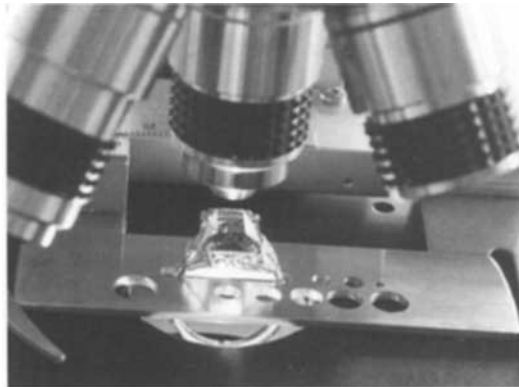
Fig. 3. Mounted stone held in slot of slide.
