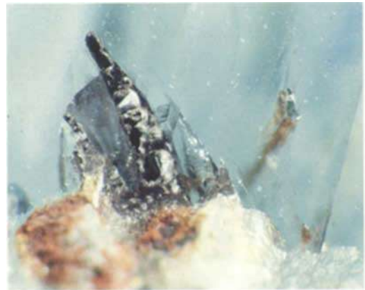
Fig. 7. Heat-treated zircon showing bubbles around thermally decomposed inclusion.
