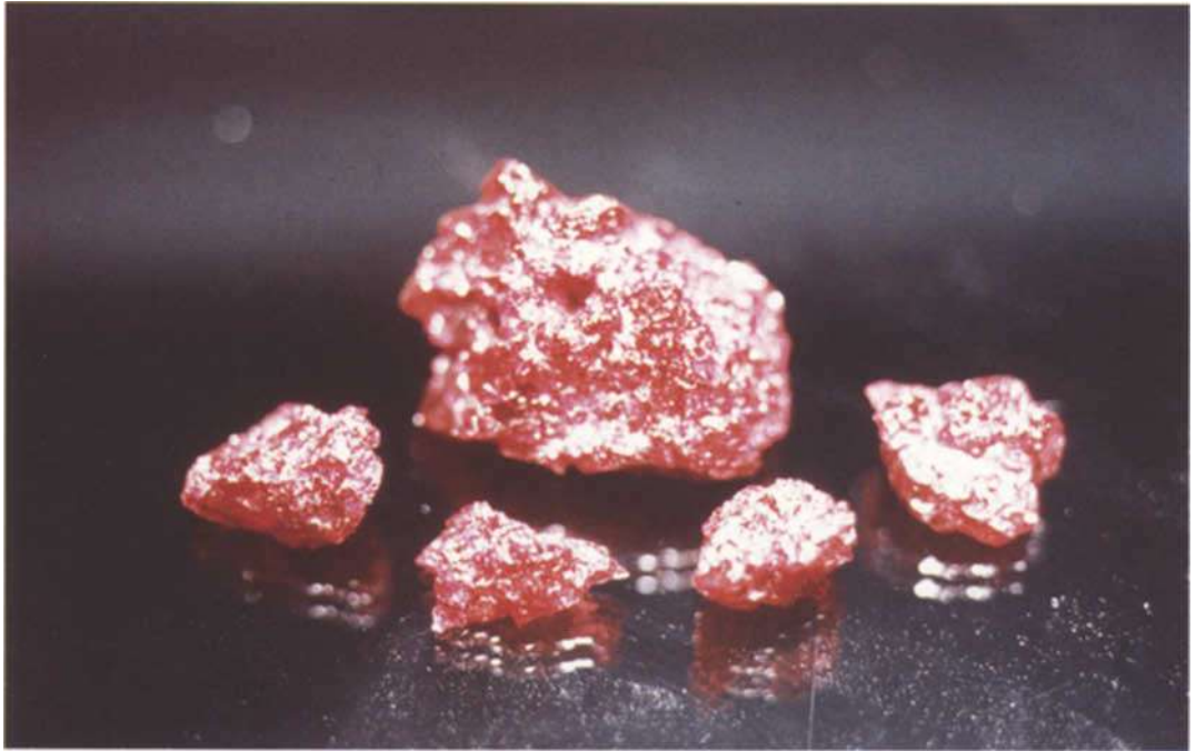
Fig.1. Aggregate-like, polycrystalline synthetic ruby from Russia, first described in 1990 (weight of the large piece 28 ct).
