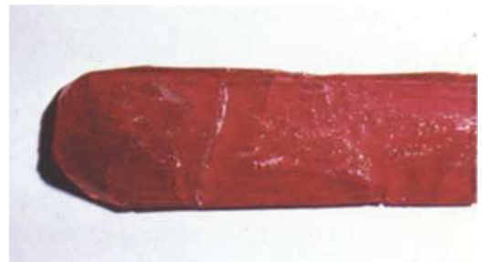
Fig.3. Elongated, tabular prismatic synthetic ruby crystal (type 1) from Russia, weighing 68.8 ct.
