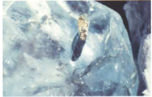
Fig. 4. Distorted crystal of ferrian spinel in highly fractured blue zircon.
