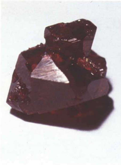
Fig.4. Rhombohedral synthetic ruby crystal of Russian production (type 2), weighing 22.6 ct.
