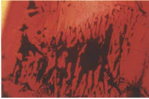
Fig.5. Black, opaque flux residues in a synthetic ruby from Russia. x10.
