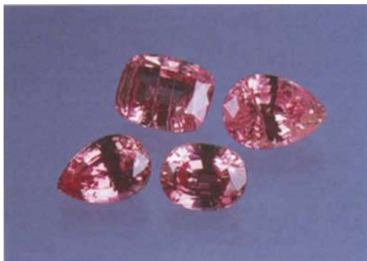
Fig. 1. These four faceted flux-grown synthetic pink sapphires comprised the test sample on which complete gemmological testing was performed for this study. Photo by Maha DeMaggio © GIA
