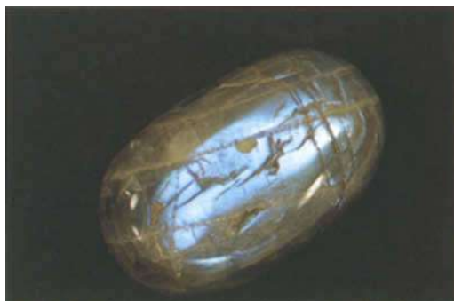
Fig. 3. Poor quality smoky moonstone from Imbulpe with cleavages, cracks and inclusions; cut as a paper weight. Size 50/30mm.
