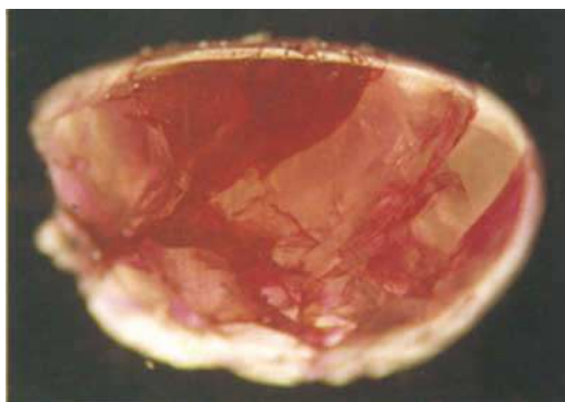
Fig. 10. Treated corundum cabochon immersed in water; red dye along fractures is easily visible. Photo: R. R. Harding
