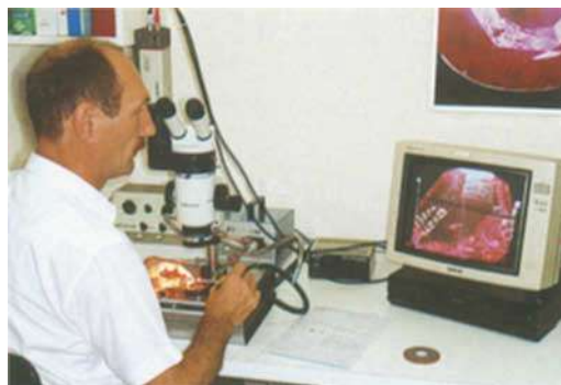
Fig. 2. Using a Leica M8 stereo microscope for identification of internal characteristics in a gemstone. A binocular microscope with different lighting possibilities, working in air and in immersion is essential for a safe gemstone identification. An adaptor enables recording of inclusion pictures by photography or video for research and education purposes.
