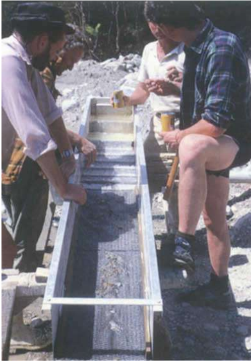
Fig. 4. Aluminium sluice box used to recover gold from the heavy mineral concentrate accumulated at an alluvial gold mine, Bell Hill, Westland, NZ. After a week's operation of the gold recovery plant, there is always an interested audience to see how much gold is produced.
