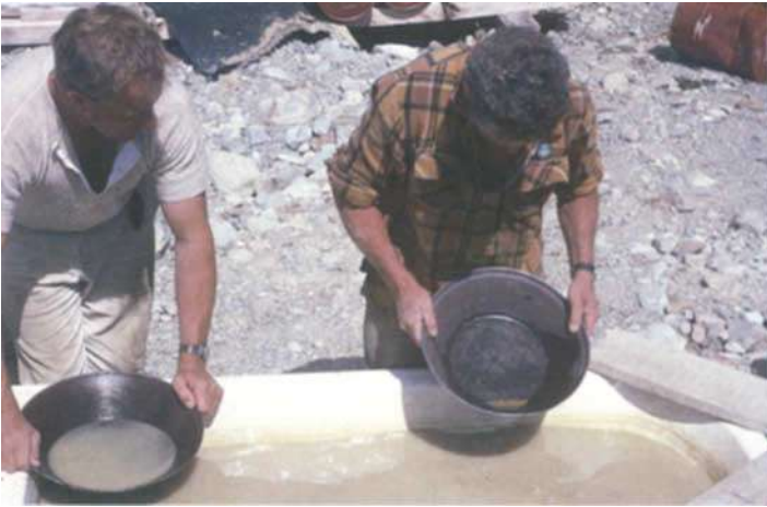
Fig. 2. Geologists use an old bathtub to pan-off concentrates at small alluvial goldmine at Bell Hill, Westland, NZ
