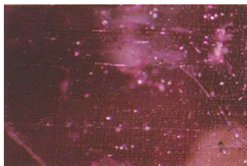
Fig. 5. Delicately arranged in neat intersecting rows producing a grid-like pattern, what appear to be minute primary flux inclusions created an unusual inclusion scene in two of the flux-grown synthetic pink sapphires. Photomicrograph by John I. Koivula © GIA. 10x
