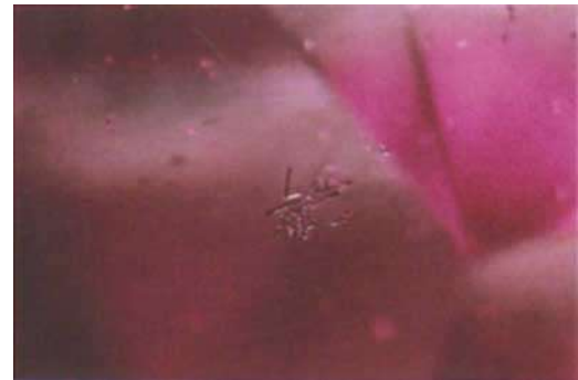
Fig. 9. Dense clusters of small rods and platelets were typical of the platinum inclusions noted. Photomicrograph by John I Koivula © GIA. 35x
