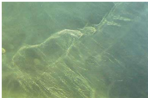
Fig. 6. White, smoke-like veiling is one of the internal characteristics noted in Vietnamese peridot. Field of view approximately 2.5mm. Photomicrograph by John I. Koivula, GIA.
