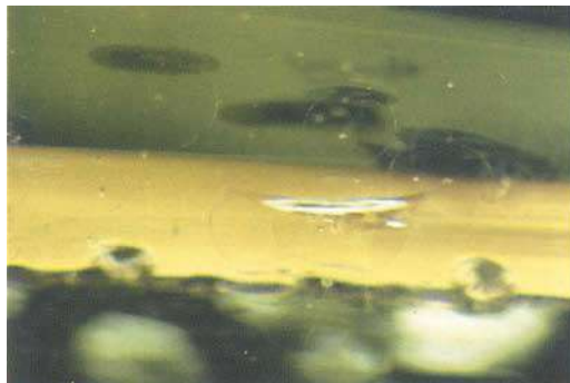
Fig. 4. These 'lily pad' inclusions are so thin as to be almost unnoticeable in darkfield illumination. Field of view approximately 3mm. Photomicrograph by John I. Koivula, GIA.
