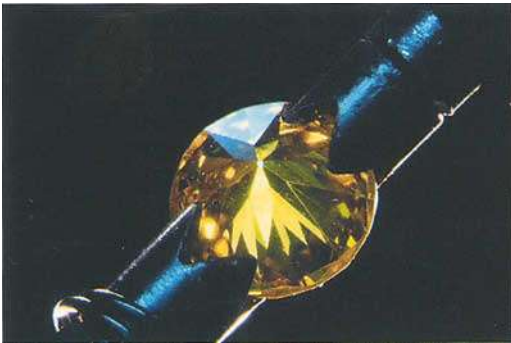
Fig. 2. When illuminated with the mercury light, the diamond exhibits a green overtone over the pavilion facets. Oblique illumination, magnification 5x.
