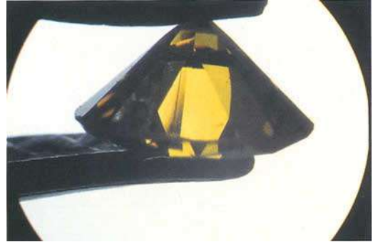
Fig. 4. As the stone is slightly rotated (compared to the position of Fig. 3) the longer grain line appears to be masked by a dark brown rectangular area. Diffuse and oblique illumination, magnification 6x.
