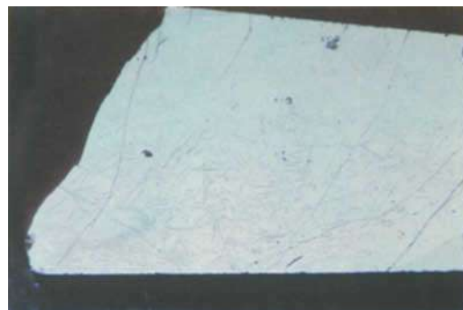
Fig 8c. Evidence of the stress such rubies may experience during the formation of these clouds can be seen by a special feature noted on the surfaces polished prior to heat treatment: the presence of very fine, shallow cracking or crazing which was most concentrated in the areas where the densest clouds reached the surface and was less concentrated where the clouds were less dense. Crazing is absent where there are no clouds, as can be seen when comparing the b and c images of this figure. Oblique fibre-optic illumination, 14x.
