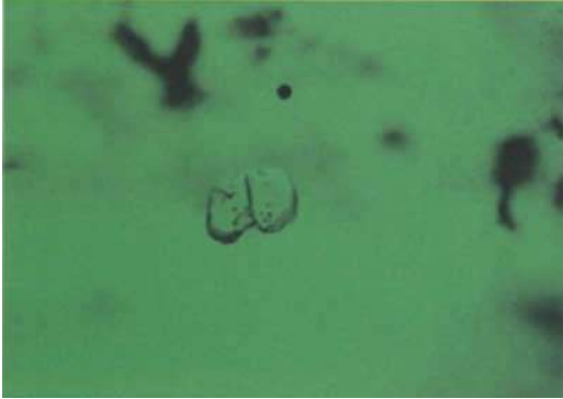
Fig. 7. Colourless, transparent, angular to irregularly shaped albite grains. \times 100
