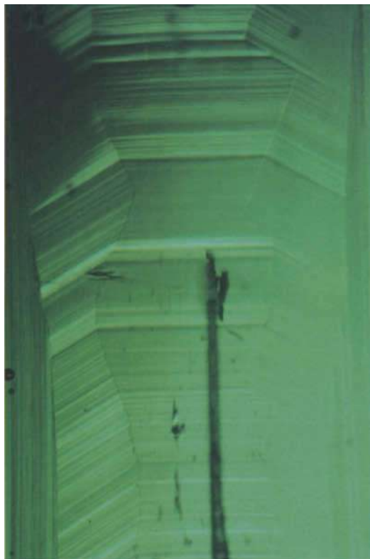
Fig. 4. Growth structures in a Nigerian emerald or green beryl (view perpendicular to the c -axis). The most dominant features run parallel and perpendicular to the c -axis. \times 70
