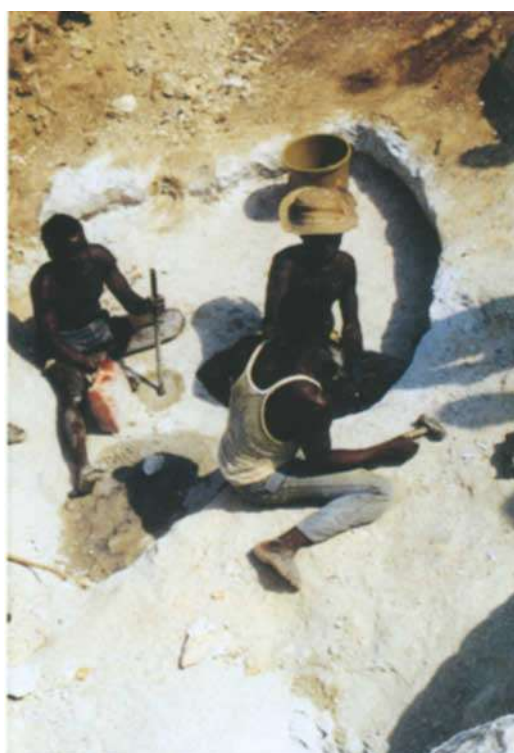
Fig. 3b. Drill holes being prepared for blasting to expose miarolitic cavities in the 'roof' zone of a Younger biotite granite; Rafin Gabas Hills. Photo J. Kanis
