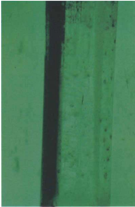
Fig. 6. Two beryl 'generations'. A distinctly visible 'core crystal' is surrounded by an 'envelope' with a different colour. \times 35
