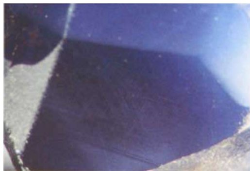
Fig. 13. Crystallographically oriented microscopic rutile inclusions ('silk') in a sapphire from SW Rwanda.
