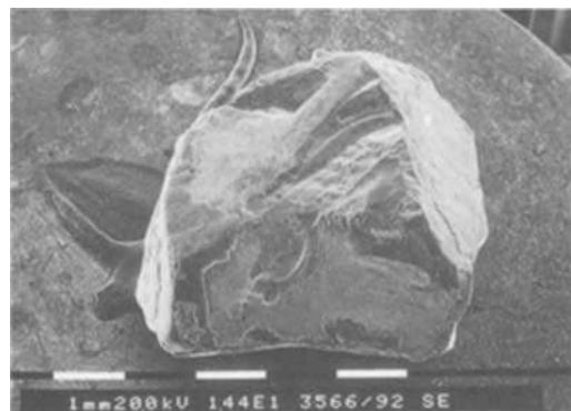
Fig. 23. SEM-micrograph of a sapphire, partially protected by a Fe-hydroxide layer.
