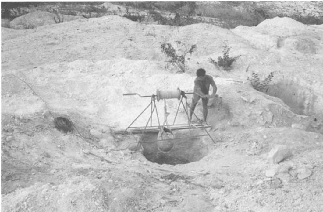
Fig. 22. Hauling with a hand winch from a pit in the kaolinized pegmatite at São José da Batalha mine.
