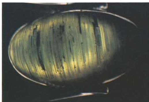
Fig. 9. Cat's-eye green tourmaline cabochon showing the many channels responsible for its chatoyancy.
