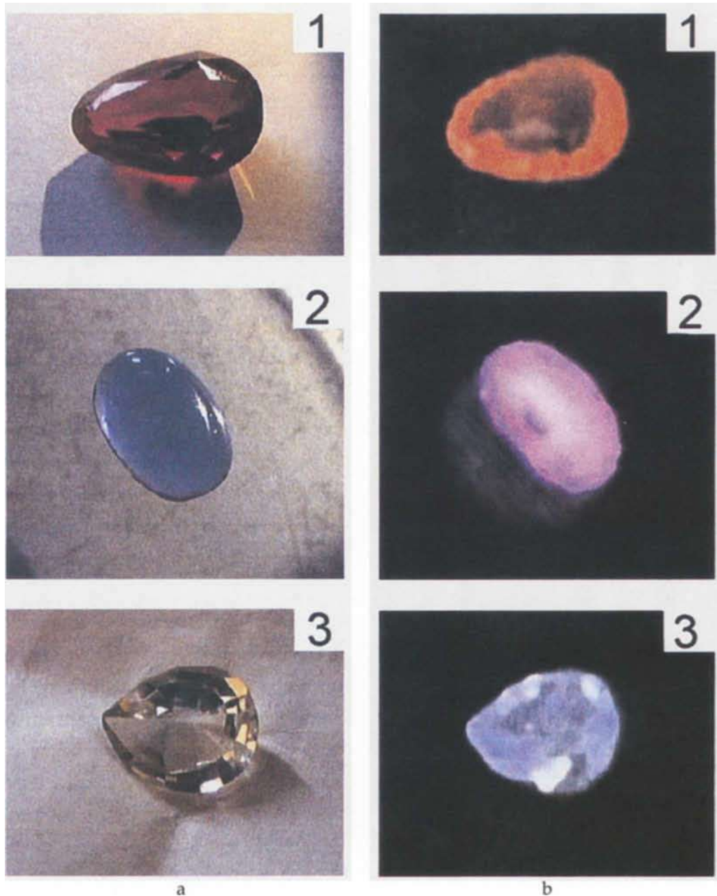
Fig. 1. Ruby (1), sapphire (2) and topaz (3) in (a) natural illumination and (b) displaying a pulsed cathodoluminescence
