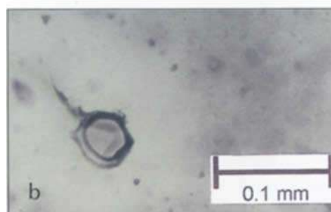
Figure 7: (a) The commonest inclusions in emeralds from Franqueira are negative crystals containing liquid and gas, as shown in this view perpendicular to the c -axis in a cut stone. (b) Negative crystals in emeralds of Franqueira show the typical prismatic faces with dihedral dipyramids terminating in pinacoids, as shown in this view parallel to the c -axis in a cut stone. (c) Some negative crystals in emeralds from Franqueira show a saw-like internal structure. View perpendicular to the c -axis in a cut stone.
