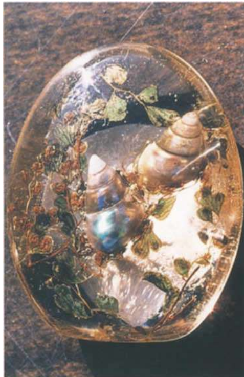
Figure 5: A keepsake manufactured by using Kauri copal to embed two small shells and some maidenhair fern. 30 mm long.
