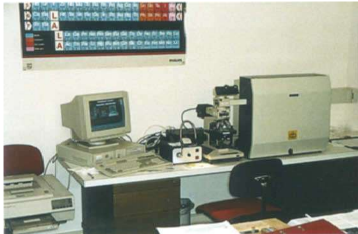
Figure 1: A Renishaw Raman microscope installed on a laboratory table at SSEF. The laser source is situated behind the spectrometer body.
