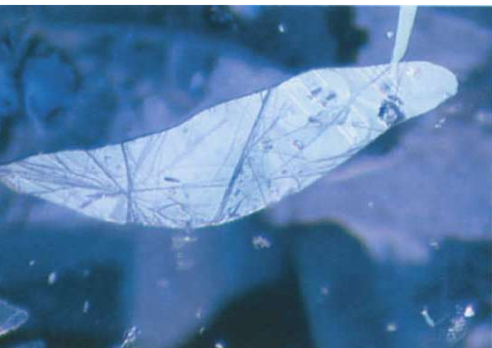
Figure 3a: Three-phase inclusion in sapphire from Madagascar oriented parallel to the basal plane and showing liquid and gaseous CO 2 and diaspore needles. View parallel to the c-axis, magnification 50x.
