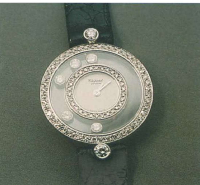
Figure 5a: A watch with moving diamonds under a sapphire cover. By Raman microscopy it is possible to record the Raman line of diamond through the watch glass.
